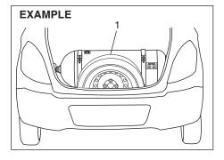
Spare wheel is located behind the CNG cylinder and secured with help of a mounting knob.
