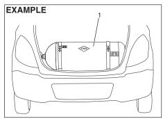
CNG cylinder (1) is installed in the luggage compartment.
