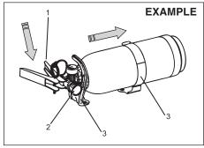
Insert the body of fire extinguisher (1) in to the clamps (3) and place the nozzle (2) carefully downwards.
