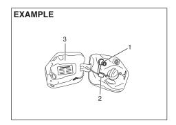
The CNG filler valve is integrated in fuel box next to petrol filling area.
