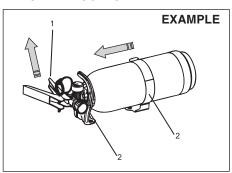
Lift Lever (1) of fire extinguisher slightly upwards and pull the fire extinguisher in the direction as shown in the figure, in order to disengage it from clamps (2).
