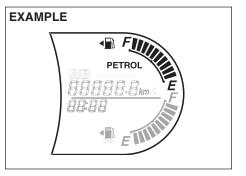
In this mode vehicle starts in petrol and continue running in petrol mode. In this mode, petrol indicator is continuously displayed and CNG indicator will remain "OFF".
