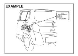
CNG cylinder identification number and CNG kit installation date is located inside the fuel filler lid.
