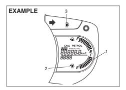
CNG level indicator (1) is built into the display. When the ignition switch is in the "ON" position, this gauge gives an approximate indication of the quantity of fuel in the CNG tank. "F" stands for full and "E" stands for empty.
