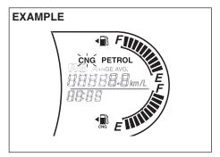
In this mode engine starts in petrol mode and then automatically changes to CNG mode after reaching programmed warming up condition. With ignition switch ON and vehicle started in "AUTO MODE", CNG indicator blinks on the display and PETROL indicator is displayed. After changeover to CNG, CNG indicator will be displayed and Petrol indicator will switch OFF automatically.
