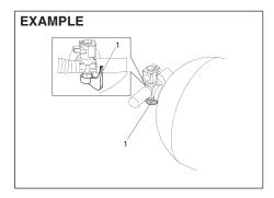
Manual shut-off valve (1) is located on the left hand side of the CNG cylinder.
