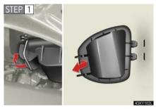
Release the lock and remove the cover.
