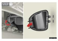
Release the lock and remove the cover.
