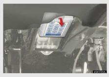
▶ Driver's side instrument panelRemove the lid.
