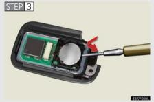
Remove the depleted battery.
