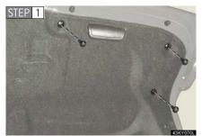
Open the trunk door and remove the trunk panel cover clips.
