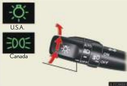
**OFF** The side marker, parking, tail, license plate and instrument panel lights turn on.
