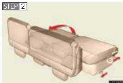
Pull the lever under the seat cushion or pull the strap on the rear end of the seat cushion and swing the whole seat forward.
