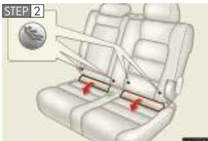
Take off the cover between the seat cushion and seatback and confirm the position of the lower anchorages below the symbol in the seatback.
