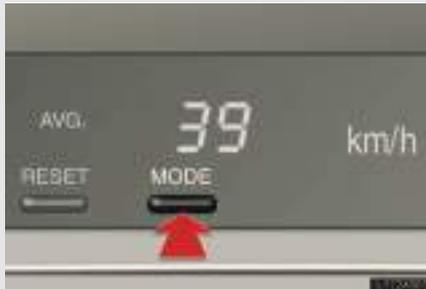
Display items can be switched by pushing the "MODE" switch.
