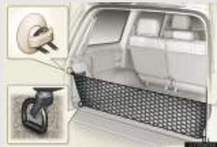
To hang the cargo net, use the cargo net hooks and rear tie-down hooks.
