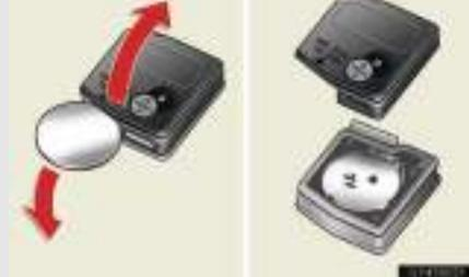
Open the case cover and remove the depleted battery.
