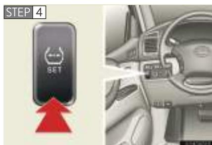
**STEP 4** Push and hold the tire pressure warning reset switch until the tire pressure warning light blinks slowly three times.
