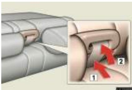
If you cannot raise the seatback because of the locked seat belt, release the lock.
