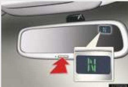
To turn the compass on or off, push "AUTO" for longer than 3 seconds.
