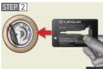
Bring the key case close to the ignition switch within 10 seconds as indicated by an arrow.
