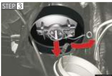
Release the wire clip and remove the light bulb.
