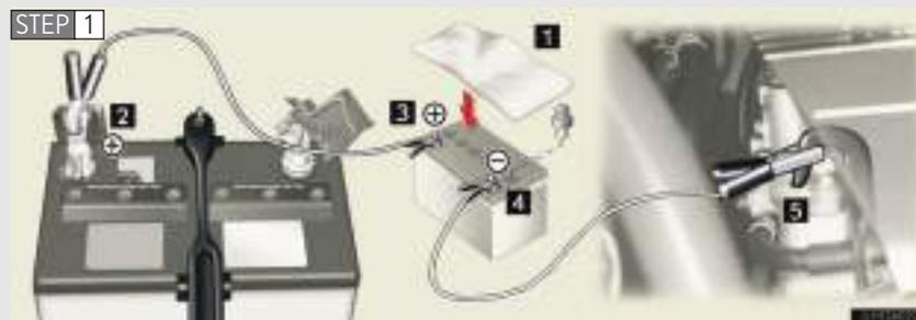
Connecting the jumper cables.
