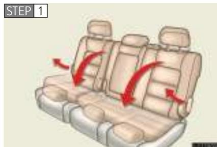
Pull the seatback angle levers and fold the second seats down.
