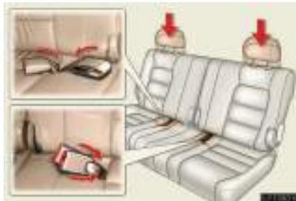
Stow the seat belts and buckles, and lower the head restraints to the lowest position.
