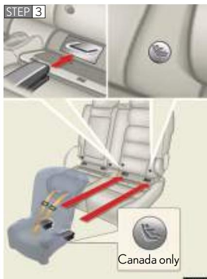
Latch the buckles onto the anchorages.
