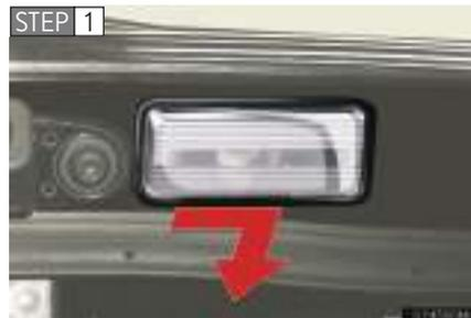
Open the back door and remove the license plate light unit.
