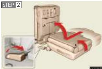
While turning the lever, lift and slide the whole seat backward.
