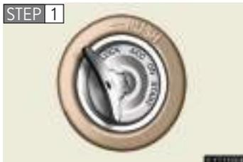
Remove the flat key from its case. Insert the key into the ignition switch.
