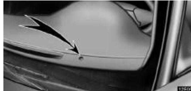
The automatic light control sensor is on the top of the driver's side instrument panel.
