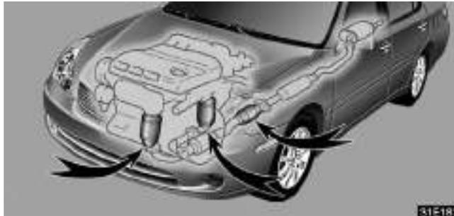
The three-way catalytic converters are emission control devices installed in the exhaust system.
