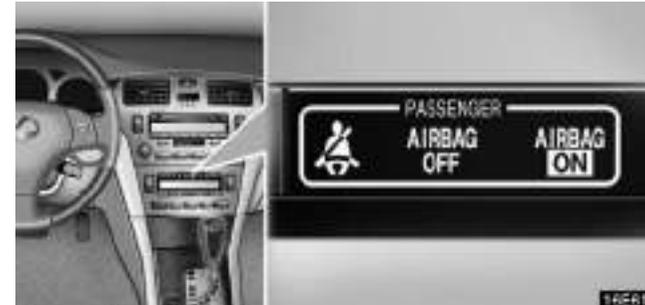
The “AIRBAG OFF” indicator light will be illuminated when the ignition switch is in the “ON” position and a child restraint system is in the front passenger seat (see table-condition 2). This indicates that in the event of a severe frontal or passenger’s side impact, the front passenger airbag and side airbag on the front passenger seat are deactivated and will not deploy.
