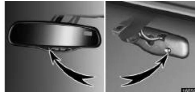
**To ensure correct functioning of anti-glare mirror sensors located on both sides of the mirror, do not touch or cover the sensors with your finger or a piece of cloth, etc.**
