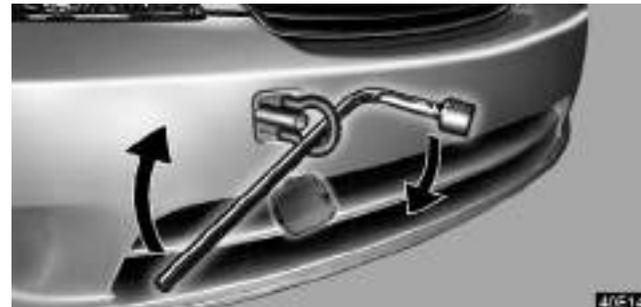
3. Tighten the front towing eyelet securely by a wheel nut wrench.
