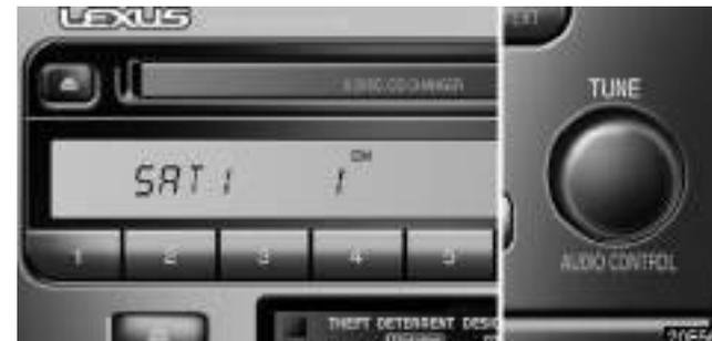
Turn the "TUNE" knob clockwise to step up the channel. Turn the knob counterclockwise to step down the channel.
