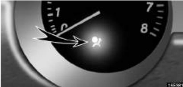
**This indicator comes on when the ignition key is turned to the “ON” position. It goes off after about 6 seconds. This means the SRS front airbags are operating properly.**
