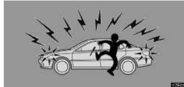
To deter theft of the vehicle, this system is designed to sound an alarm if any of the doors, trunk or hood is forcibly unlocked or the battery terminal is disconnected and then reconnected while the vehicle is locked.
