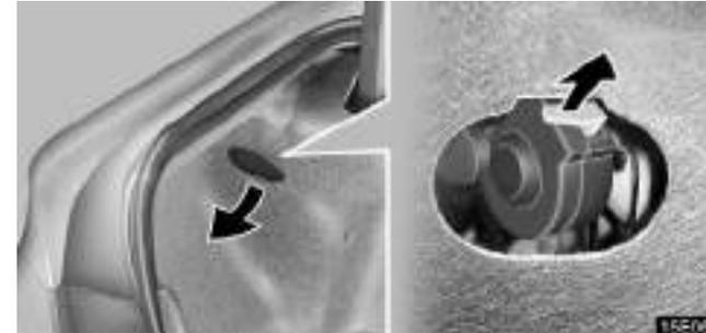
Remove the cover and pull up the manual lever in the trunk.
