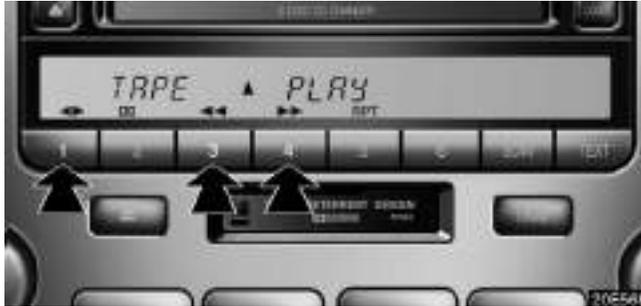
**“Program” button:** Push the “◀▶” button to select the other side of a cassette tape. The display indicates which side is currently selected (“▲” indicates top side, “▼” indicates bottom side).
