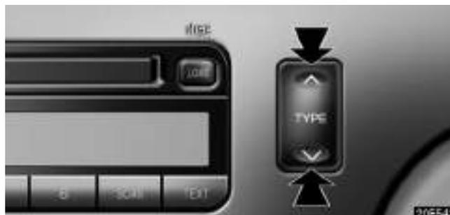
When you push the “TYPE” button while tuned to FM broadcasts, the current program type appears on the display.
