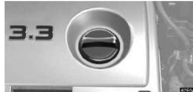
**If the oil level is below or only slightly above the low mark, add engine oil of the same type as already in the engine.**
