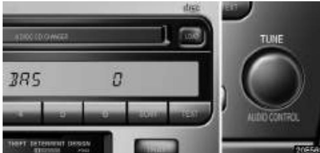
Each time you push the “AUDIO CONTROL” knob, the display changes as in the following. To adjust the tone and balance or turn on or off the Automatic Sound Levelizer, turn the knob.
