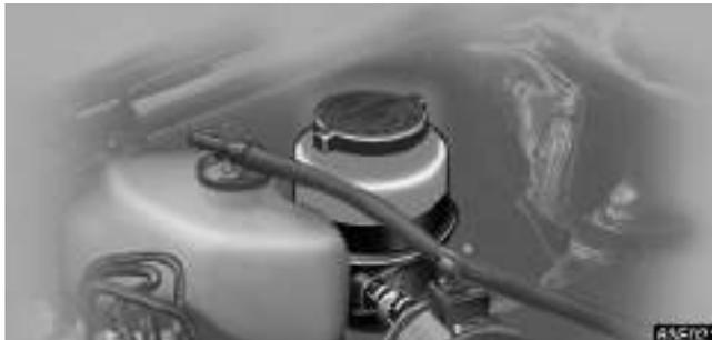
**Check the fluid level through the reservoir. If necessary, add automatic transmission fluid DEXRON® II or III.**
