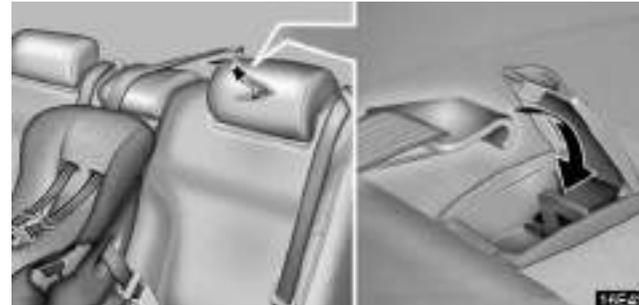
3. Fix the child restraint system with the seat belt.
