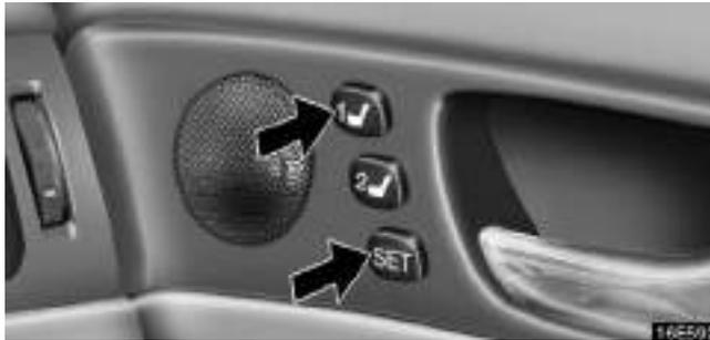
When you push button "1" or "2", the seat position will be automatically adjusted to the position recorded for that button.
