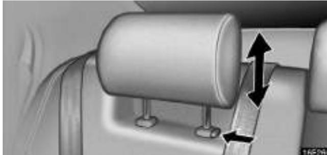
To raise the head restraint, pull it up. To lower it, press the lock release button and push the head restraint down.
