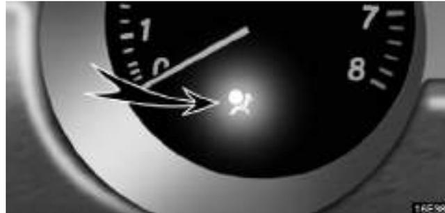
This indicator comes on when the ignition key is turned to the “ON” position. It goes off after about 6 seconds. This means the seat belt pretensioners are operating properly.
