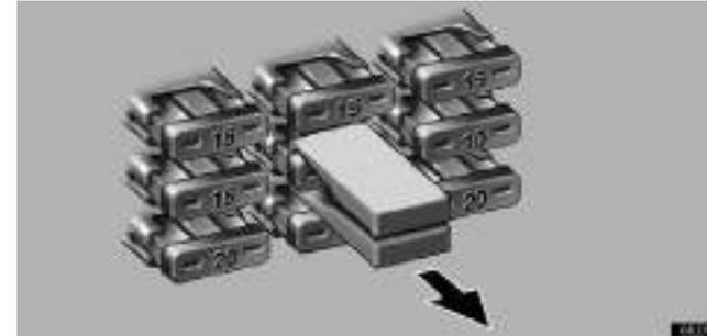
2. Make sure the inoperative component is turned off. Pull the suspected fuse straight out with the pull-out tool and check it. If it has blown, push a new fuse into the clips.
