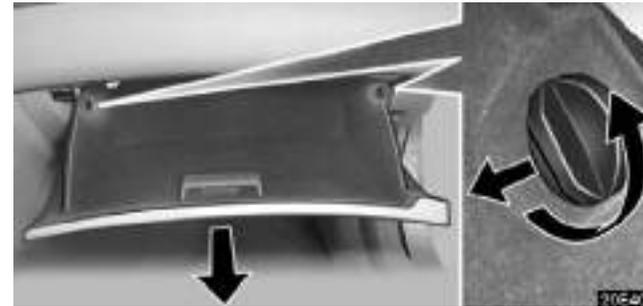
2. Remove the 2 pins installed on the upper part of the glove box and lower the glove box.
