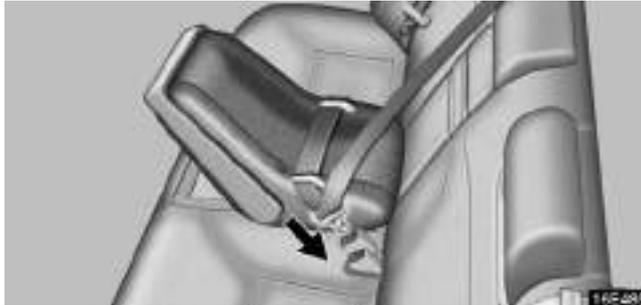
1. Run the lap and shoulder belt through or around the infant seat following the instructions provided by its manufacturer and insert the tab into the buckle taking care not to twist the belt. Keep the lap portion of the belt tight.
