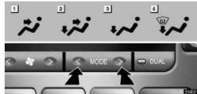
The outlets from which air is delivered can be selected manually by pushing the button. The function of each mode is as follows:
