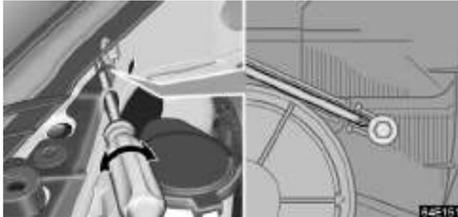
2. Turn the vertical movement adjusting bolt 2 the same number of turns and in the same direction as step 1 using a Phillips-head screwdriver.
