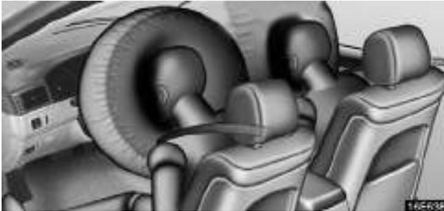
**The SRS (Supplemental Restraint System) front airbags are designed to provide further protection for the driver and front passenger in addition to the primary safety protection provided by the seat belts.**
