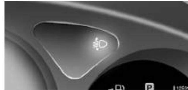
Vehicle position changes according to loading condition, passengers getting on and off, vehicle acceleration and deceleration, etc. However, the headlight beam level is always maintained automatically by the system at the proper level so that your headlights do not dazzle other road users.
