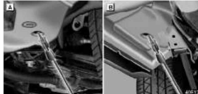
If your Lexus is transported by a flat bed, it should be tied down at locations A and B as shown above.
