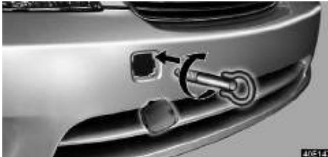
2. Use the front towing eyelet in the trunk. Secure it to the hole on the bumper by turning clockwise. (For the eyelet location, see page cccxi.)
