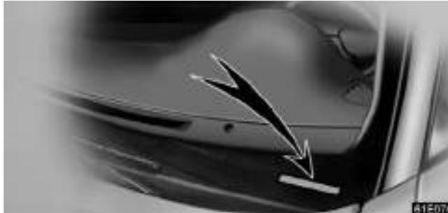
**The vehicle identification number (VIN) is the legal identifier for your vehicle. This number is on the left top of the instrument panel and can be seen through the windshield from outside.**
