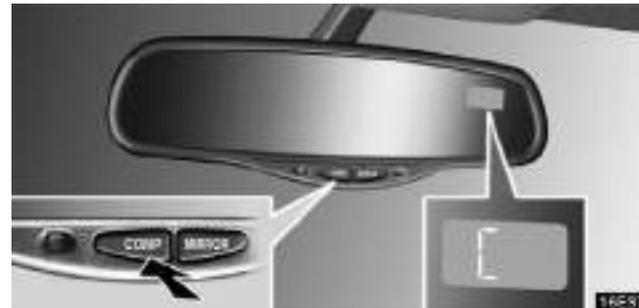
To rectify the compass, stop the vehicle and push and hold the "COMP" switch until "C" appears on the display.
