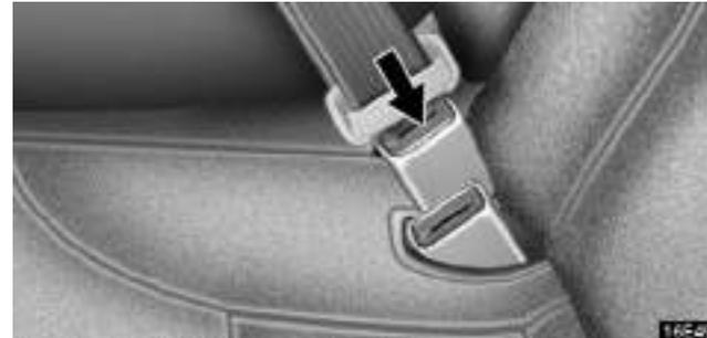
2. To remove the booster seat, press the buckle release button and allow the belt to retract.
