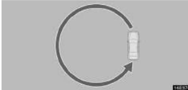
Drive the vehicle slowly (at 8 km/h [5 mph] or lower) in a circle until the direction is displayed. If there is not enough space to drive in a circle, drive around the block until the direction is displayed.
