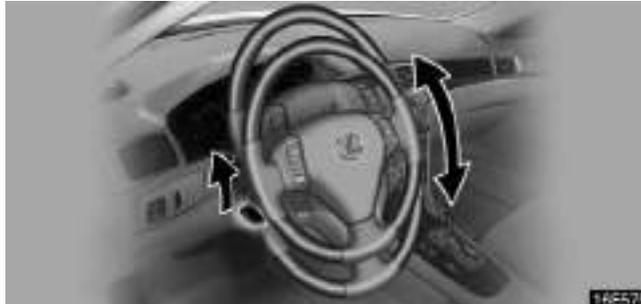
To change the steering wheel angle, hold the steering wheel, pull up the lock release lever, tilt the steering wheel to the desired angle and release the lever.
