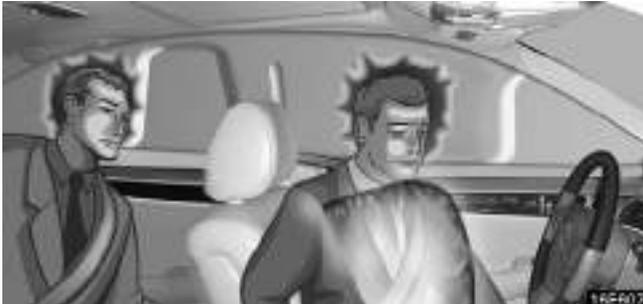
**The SRS (Supplemental Restraint System) side airbags and curtain shield airbags are designed to provide further protection for the driver, front passenger and rear outboard passengers in addition to the primary safety protection provided by the seat belts.**
