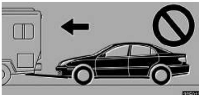
Your vehicle is not designed to be dinghy towed (with four wheels on the ground) behind a motorhome.
