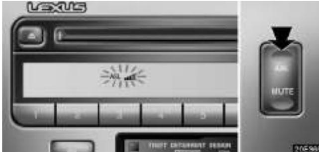
When the audio sound becomes difficult to be heard due to road noise, wind noise, etc. during driving, the system adjusts to the optimum volume and tone quality according to the noise level. While the Automatic Sound Levelizer is on, "ASL" appears on the display.
