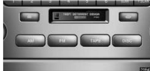
**Push the “AM”, “FM”, “TAPE” or “DISC” button to turn on that mode. The selected mode turns on directly.**
