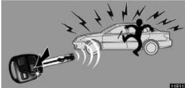
When you push the “PANIC” button for about 2 to 3 seconds, an alarm sounds to deter any person trying to break into or damage your vehicle.
