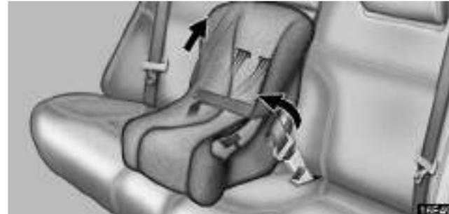
3. While pressing the convertible seat firmly against the seat cushion and seatback, let the shoulder belt retract as far as it will go to hold the convertible seat securely.
