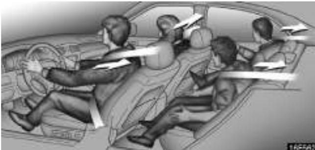
**Both front seats and the two outboard rear seats are equipped with seat belt pretensioners and are designed to be activated in response to a severe frontal impact.**
