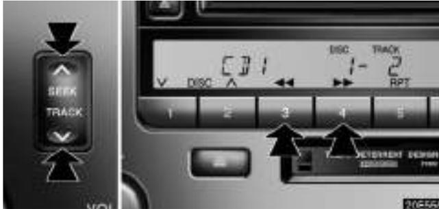
**“TRACK” button:** Use for direct access to a desired track.
