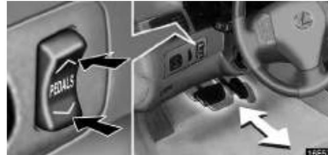
To adjust the position of the accelerator and brake pedals, push the switch.
