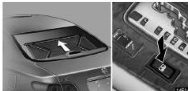
To raise the rear electric sunshade, push the switch. To lower the sunshade, push the same switch again.
