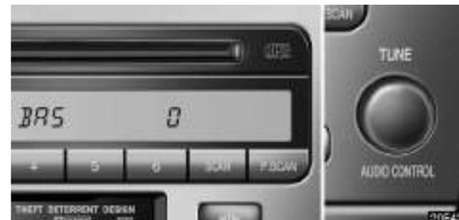
Each time you push the “AUDIO CONTROL” knob, the display changes as in the following. To adjust the tone and balance, turn the knob.
