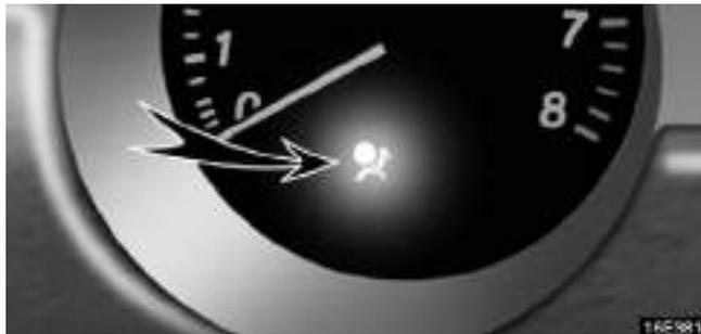
**This indicator comes on when the ignition key is turned to the “ON” position. It goes off after about 6 seconds. This means the SRS side airbags and curtain shield airbags are operating properly.**
