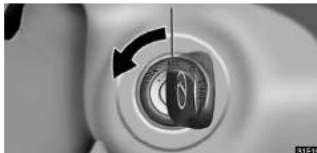
**“LOCK”** — Engine is off and the steering wheel is locked. The ignition key can be removed only at this position.
