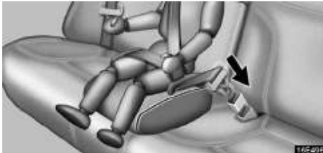
1. Sit the child on a booster seat. Run the lap and shoulder belt through or around the booster seat and across the child following the instructions provided by its manufacturer and insert the tab into the buckle taking care not to twist the belt.
