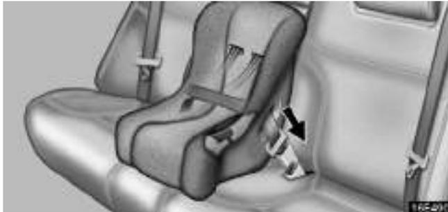
1. Run the lap and shoulder belt through or around the convertible seat following the instructions provided by its manufacturer and insert the tab into the buckle taking care not to twist the belt. Keep the lap portion of the belt tight.
