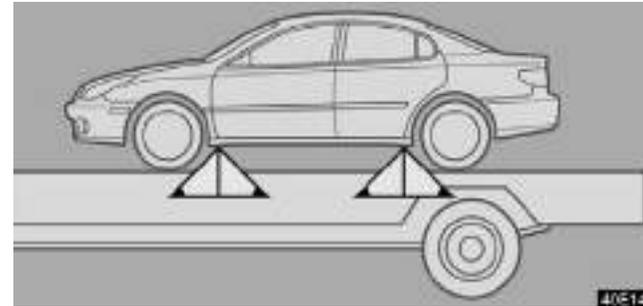
If you use chains or wires to tie down your vehicle, the angles shaded black must be at 45°.
