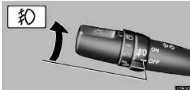
To turn on the fog lights, turn the switch to the “ON” position. The fog lights come on only when the headlights are on low beam.
