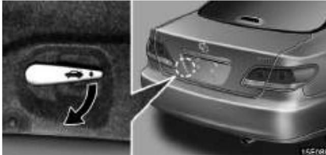
If a person is locked in the trunk, he/she can pull down the phosphorescent handle on the inside of trunk lid to open the trunk lid.
