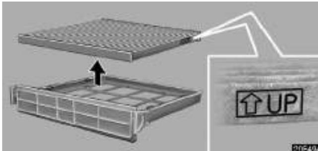
4. Remove the filter from the filter case.
