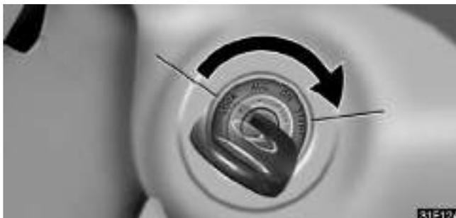
**“START”** — Starter motor on. The key will return to the “ON” position when released.
