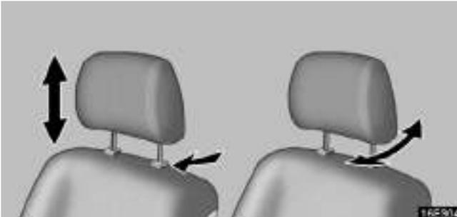
To raise the head restraint, pull it up. To lower it, press the lock release button and push the head restraint down. To move the head restraint forward or rearward, pull or push the base of the head restraint.
