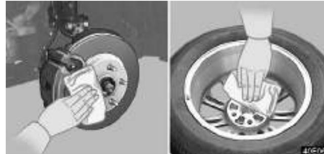
Before putting on the wheel, remove any corrosion on the mounting surfaces with a wire brush or such. Installation of wheels without good metal-to-metal contact at the mounting surface can cause wheel nuts to loosen and eventually cause a wheel to come off while driving.
