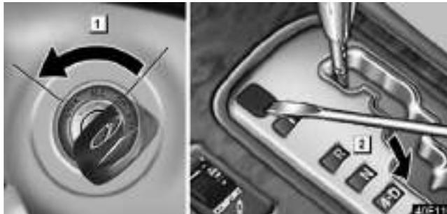
**If you cannot shift the selector lever out of “P” position to other positions even though the brake pedal is depressed, use the shift lock override button as follows:**
