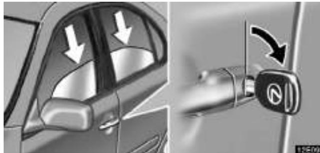
**Insert the ignition key into the key hole on the driver's door.**
