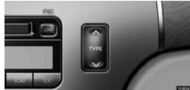
When you push the “^” or “v” side of the “TYPE” button while receiving a XM channel.
