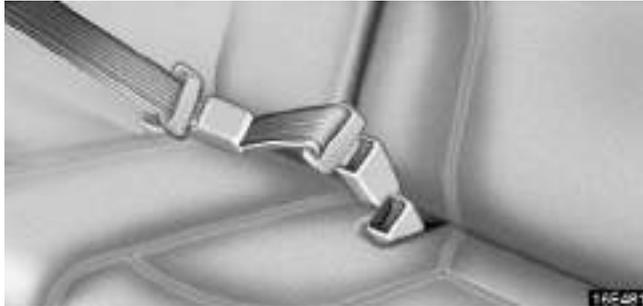
To connect the extender to the seat belt, insert the tab into the seat belt buckle so that the “PRESS” signs on the buckle release buttons of the extender and the seat belt are both facing outward as shown.
