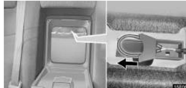
**2. Pull the loop of wire to unlock the trunk lid.**
