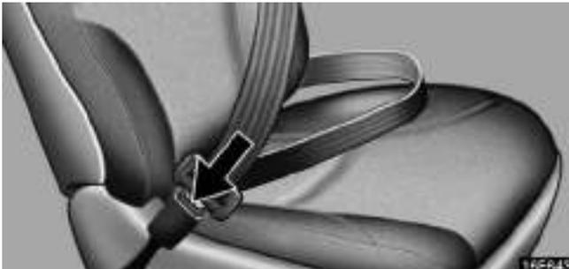
**To release the belt, press the buckle release button and allow the belt to retract.**
