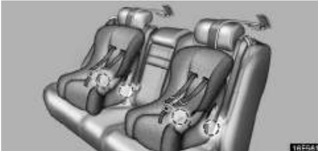
**Lower anchorages for the child restraint systems complying with the FMVSS225 or CMVSS210.2 specifications are installed in the rear seat.**
