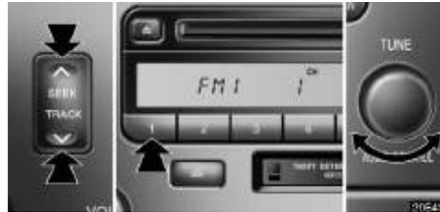
**Seek tuning:** Push the “SEEK” button. The radio will begin seeking up or down for a station of the nearest frequency and will stop on reception. Each time you push the button, the stations will be searched automatically one after another.
