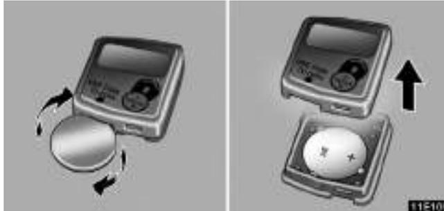
3. Open and remove the battery case cover using a coin.
