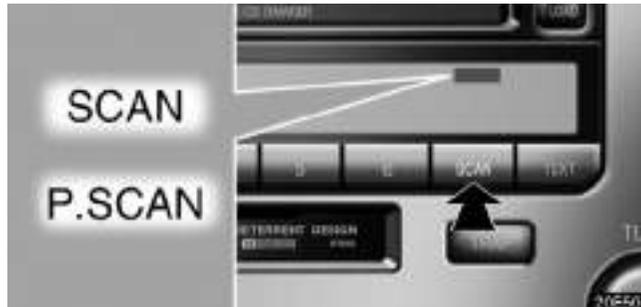
**To scan the currently selected channel category:** Quickly push and release the “SCAN” button. “SCAN” appears on the display. The radio will find the next channel in the same channel category up the band, stay there for 5 seconds, and then scan again. To stop scanning, push this button again.
