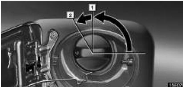
**2. To remove the fuel tank cap, turn the cap counterclockwise by 90 degrees (to the pressure point **1**), and then turn it an additional 30 degrees (to point **2**). Pause slightly before removing it.**
