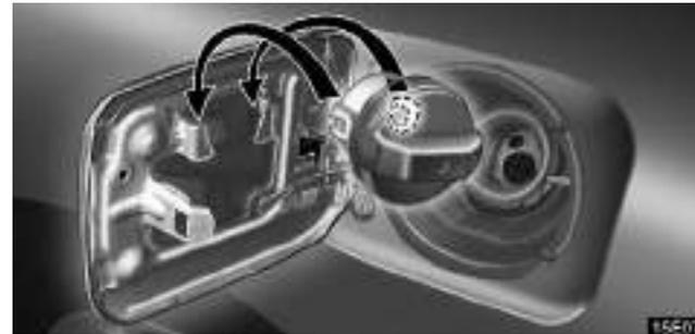
**3. The removed cap can be stored on the back side of the fuel filler door.**
