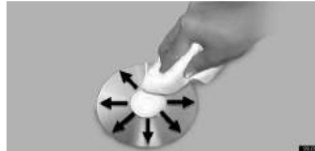
**To clean a CD:** Wipe it with a soft, lint-free cloth that has been dampened with water. Wipe in a straight line from the center to the edge of the CD (not in a circle). Do not use a conventional record cleaner or anti-static device.
