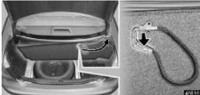
**1. Lift up the deck board and hang the deck board hook on the right hinge of the trunk lid.**
