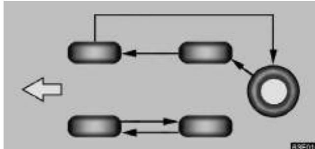
To equalize tire wear and help extend tire life, Lexus recommends that you rotate your tires according to the maintenance schedule. (For scheduled maintenance information, please refer to the “Owner’s Manual Supplement/Scheduled Maintenance”.) However, the most appropriate timing for tire rotation may vary according to your driving habits and road surface conditions.
