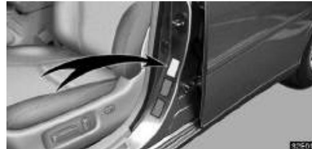
The vehicle identification number (VIN) is also on the Certification Label.
