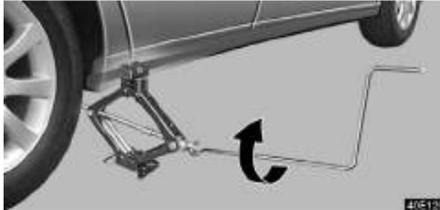
**6. After making sure no one is in the vehicle, raise it high enough so that the spare tire can be installed.**
