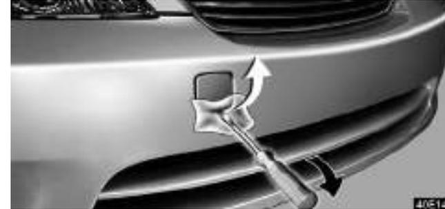
1. Remove the front towing eyelet cover on the front bumper using a flathead screwdriver. To protect the bodywork, place a piece of rag over the cover.
