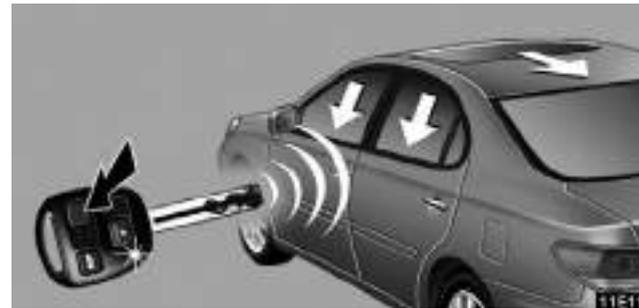
Push the “UNLOCK” button until the windows and moonroof start to move. When you release the button, the windows and moonroof stop operating.
