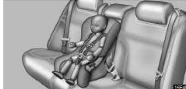
**A convertible seat must be used in forward-facing or rear-facing position depending on the age and size of the child. When installing, follow the manufacturer's instructions about the applicable child's age and size as well as directions for installing the child restraint system.**
