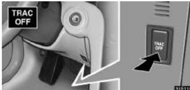
**If your wheels get stuck in a ditch when you are driving on a severe off road and sand, turn off the traction control system. This system that controls engine performance interferes with the process of freeing your wheels.**
