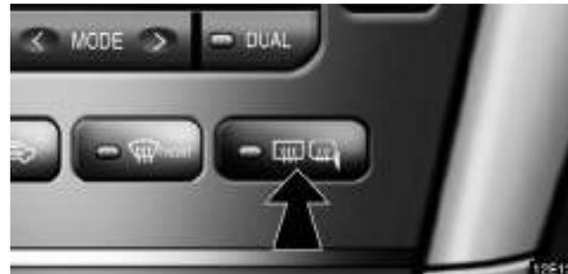
**To turn the electric rear window and outside rear view mirror defogger on, push the switch.**
