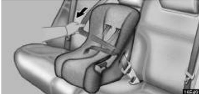
2. Fully extend the shoulder belt to put it in the lock mode. When the belt is then retracted even slightly, it cannot be extended.
