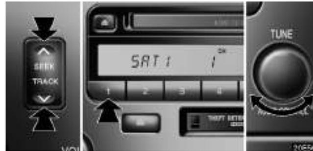
**Seek tuning:** To select the next channel within the current channel category, push the “^” or “v” side of the “SEEK/TRACK” button. Repeat until a desired channel is found.
