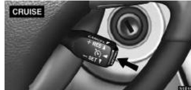
To turn the cruise control on, press the “ON–OFF” button. The “CRUISE” indicator light in the instrument cluster will come on to indicate that the cruise control is operational. Pressing the “ON–OFF” button again turns the system off.
