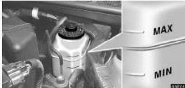
To check the fluid level, simply look at the see-through reservoir. The level should be between the “MAX” and “MIN” lines on the tank.
