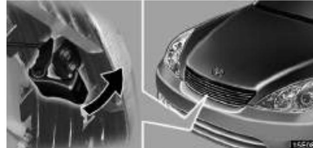
**2. Insert your fingers under the hood, push up the auxiliary catch lever and lift the hood.**
