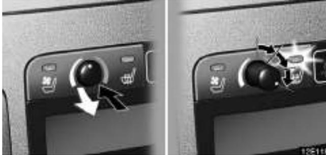
**To turn on the seat heater, push the knob to pop it out and then turn the knob clockwise. The indicator light (yellow) comes on.**
