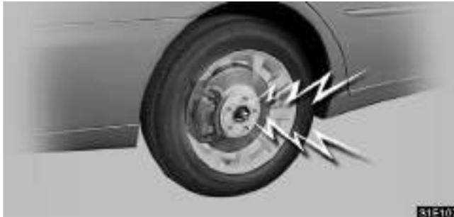
**The brake pad wear limit indicators on your disc brakes give a warning noise when the brake pads are worn to the extent that replacement is required.**
