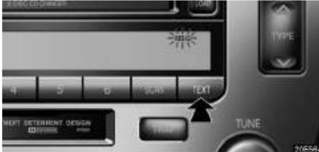
If the radio receives a radio text from RDS station, "MSG" appears on the display. Push the "TEXT" button, and a text message is displayed.
