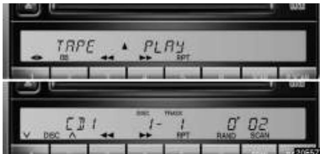
In the “TAPE” or “CD” mode, the applicable functions are shown in the lowest part of the display. Push the switch just below to turn on each function.
