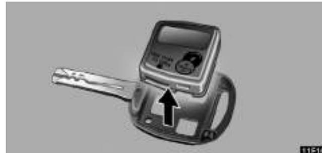
2. Remove the module from the key frame.
