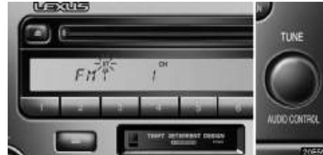
Turn this knob to the right to step up the station band or to the left to step down.
