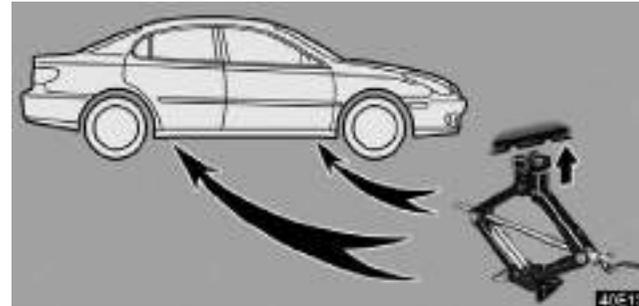
**5. Position the jack at the jack points as shown. Rotate the load rest 90° from storage position to lifting position.**
