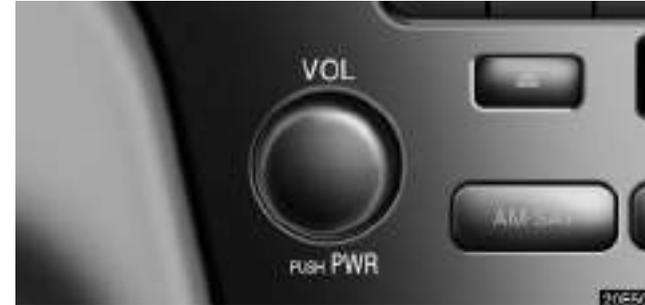
Push this knob to turn the audio system on and off. Turn this knob to adjust the volume.
