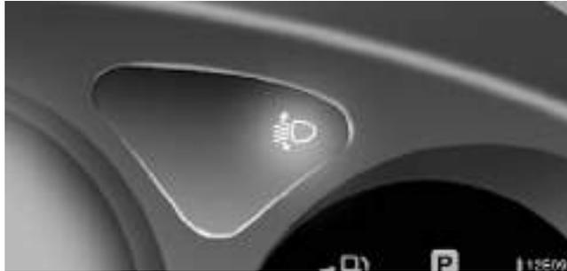
Vehicle position changes according to loading condition, passengers getting on and off, vehicle acceleration and deceleration, etc. However, as the headlight beam level is always maintained automatically by the system at the proper level, your headlights do not dazzle other road users.
