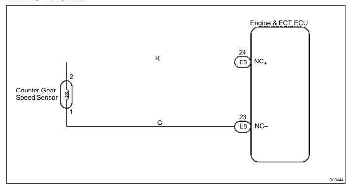
1 Check resistance between terminals NC+ and NC- of Engine & ECT ECU.
