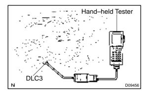
To check the DTCs, connect the OBD scan tool or hand–held tester to the Data Link Connector 3 (DLC3) on the vehicle. The OBD scan tool or hand–held tester also enables you to erase the DTCs and check freezed frame data and various forms of engine data (For operating instructions, see the OBD scan tool's instruction book.).
