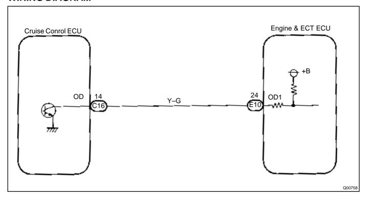
1 Check voltage between terminal OD1 of Engine & ECT ECU and body ground.
