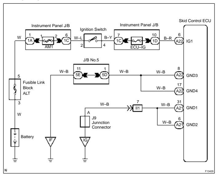
1 Check that the ECU connectors are securely connected to the ECU.
