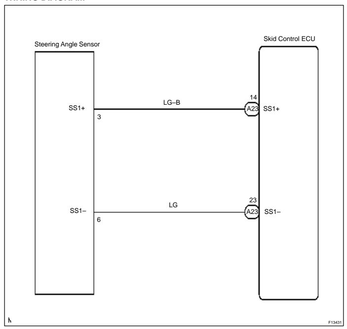
1 Check for open and short circuit in harness and connector between steering angle sensor and skid control ECU (See page IN–32).
