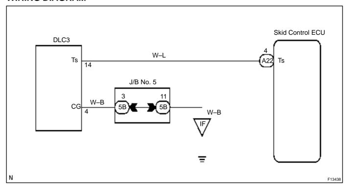
1 Check voltage between terminals Ts and CG of DLC3.
