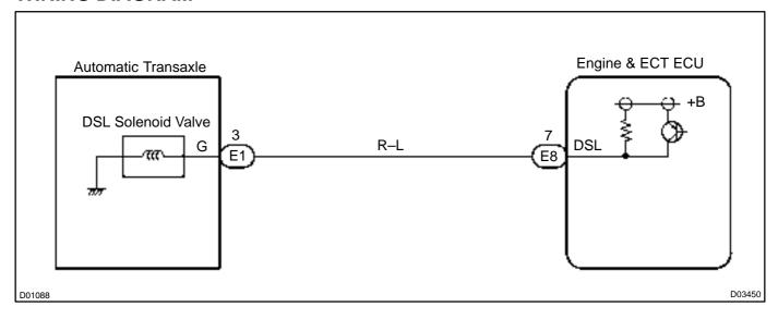
1 Check harness and connector between Engine & ECT ECU and automatic transaxle solenoid connector (See page IN-32).
