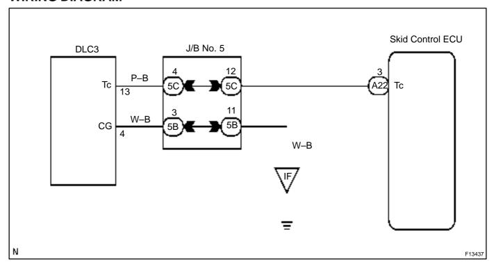
1 Check voltage between terminals Tc and CG of the DLC3.
