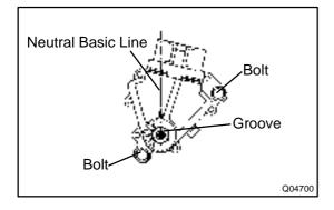
(e) Inspect and adjust the shift lever position. When shifting the shift lever from the N range to other ranges, check that the lever can be shifted smoothly and accurately to each range and that the position indicator is
