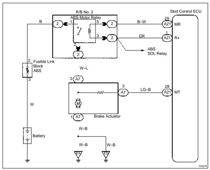
1 Check operation of pump motor.
