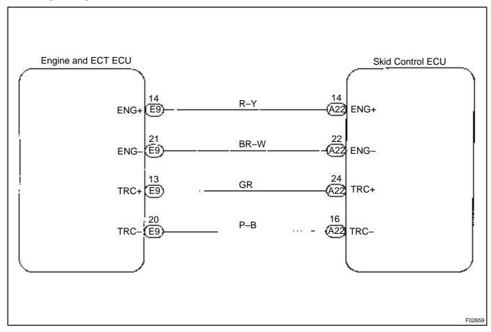
1 Check for open and short circuit in harness and connector between each of terminals ENG+, ENG-, TRC+, TRC- of skid control ECU and engine and ECT ECU (See page IN-32).
