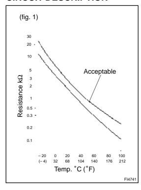
The intake air temp. sensor is built into the air flow meter and senses the intake air temperature.
