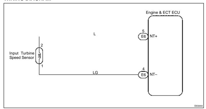
1 Check resistance between terminals NT+ and NT- of Engine & ECT ECU.
