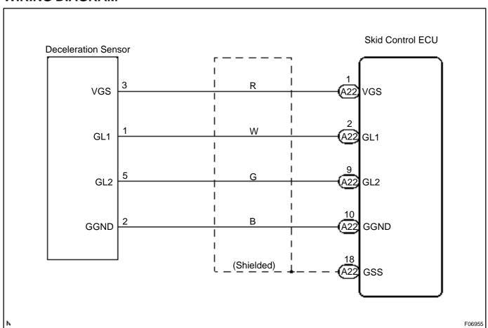
1 Check for open and short circuit in harness and connector between deceleration sensor and skid control ECU (See page IN–32).
