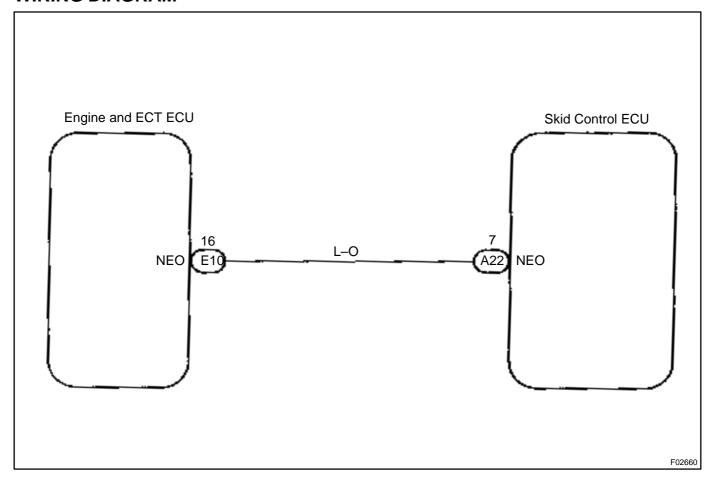
1 Check for open and short circuit in harness and connector between terminal NEO of skid control ECU and terminal NEO of engine and ECT ECU (See page IN-32).
