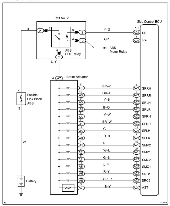
1 Check brake actuator solenoid.
