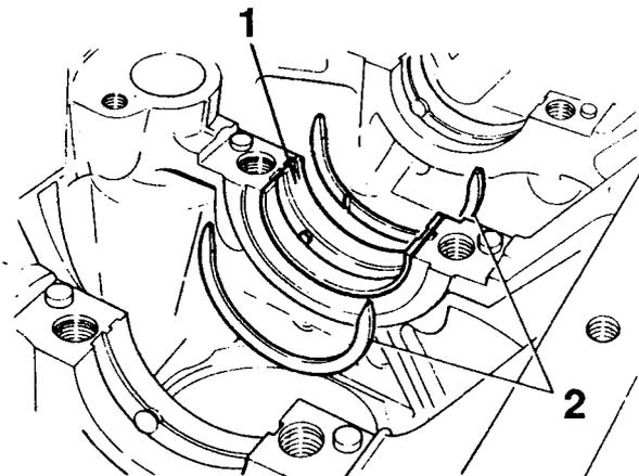
**Fig.24 Crankshaft thrust washers.**
