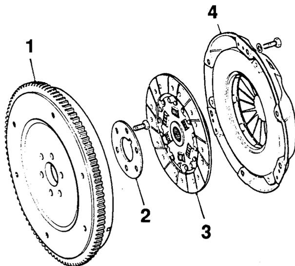
**Fig 1 Clutch Assembly**
