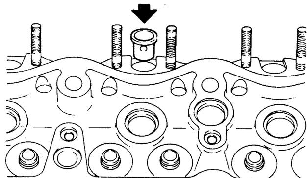
**Fig 7 Fitting shroud**
