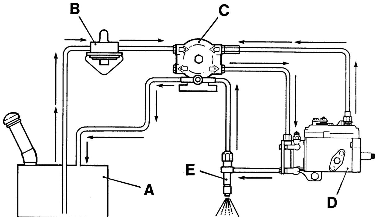
**Fig 1 Fuel system layout**
