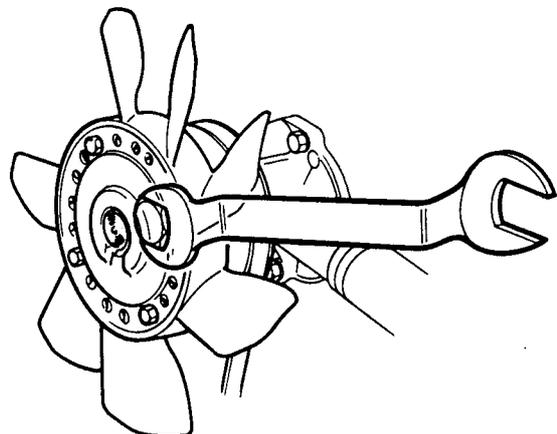
**Fig.4** Using tool MS1517 to release the fan assembly
