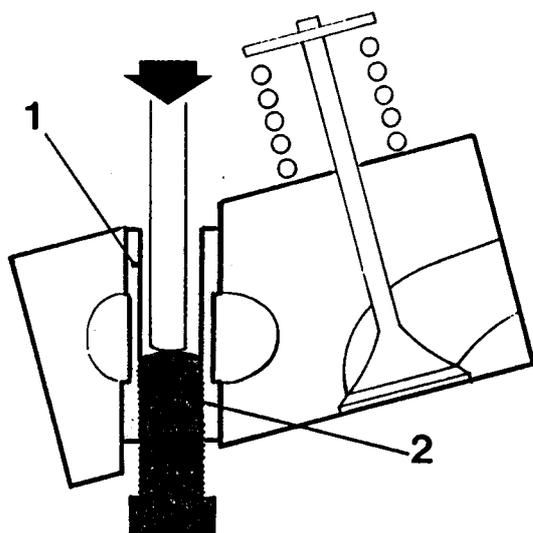
**Fig.9** Removing push rod tube.
