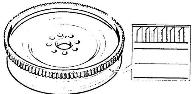
**Fig.3 Fitting starter ring gear. (Inset shows squared edge of teeth downwards)**
