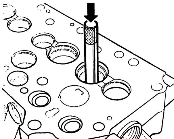
**Fig.10** Removing valve guide.
