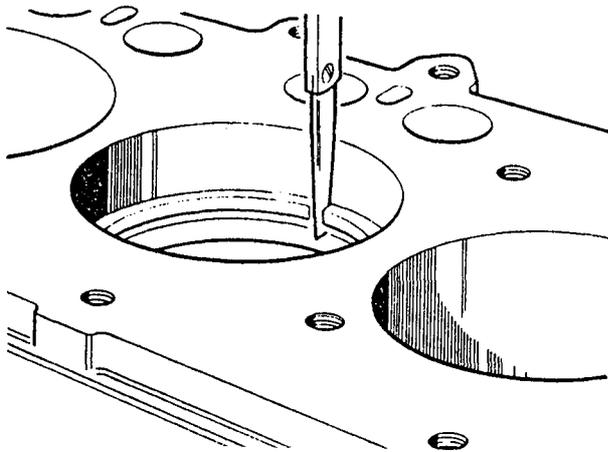
**Fig.14 Measuring piston ring gap in bore.**
