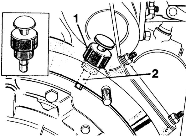
**Fig.9 Timing pin LST 107 fitted to flywheel housing**
