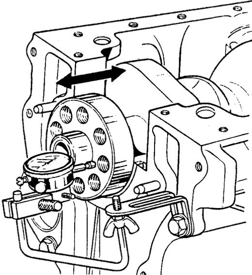
**Fig.25 Measuring crankshaft end float.**
