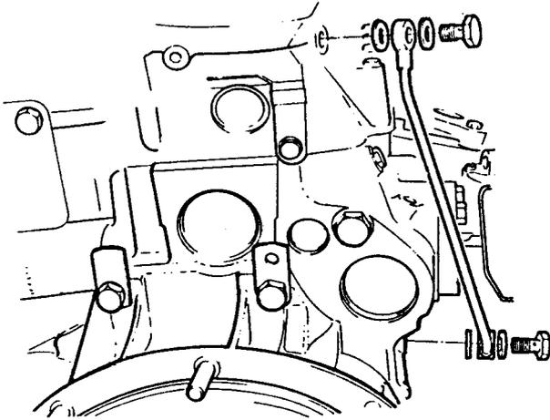
**Fig.24** Cylinder head oil feed pipe.
