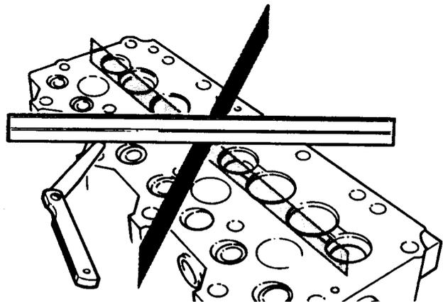
**Fig.4 Checking cylinder head distortion.**
