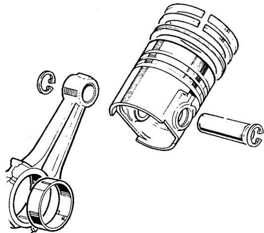
**Fig.11** Connecting rod and piston.
