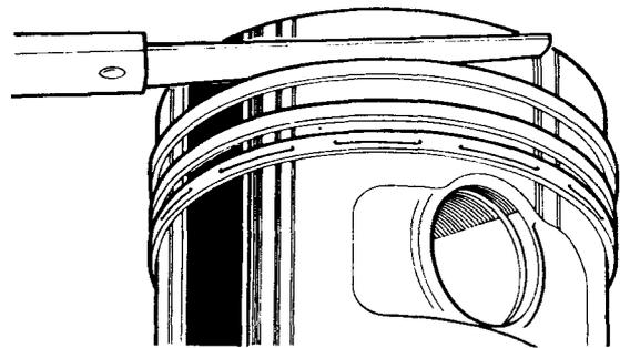
**Fig.15 Measuring piston ring side clearance.**
