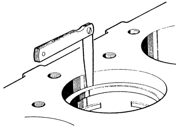
**Fig.13 Measuring piston clearance.**
