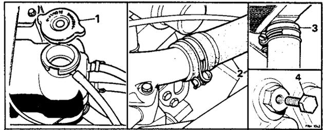
**Fig.2 Coolant draining**
