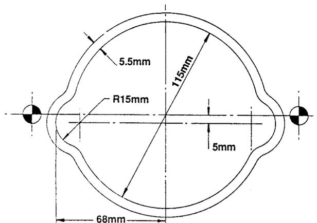
**Fig.6 Sealant application - flywheel housing**
