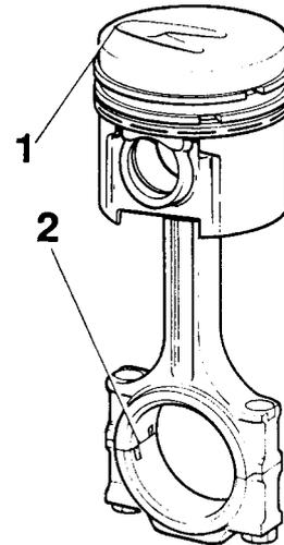
**Fig.19 Fitting piston to connecting rod.**
