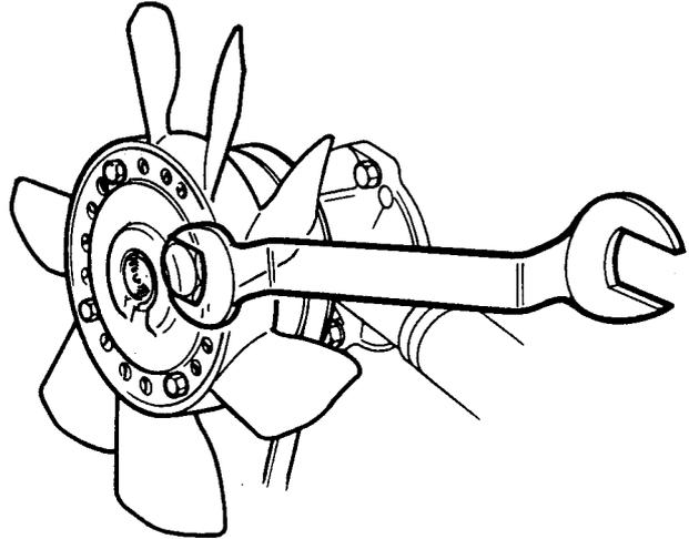
**Fig.1 Using tool MS 1517 to release fan assembly**
