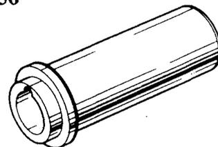
Crankshaft front oil seal replacer
