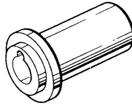
Camshaft oil seal replacer
