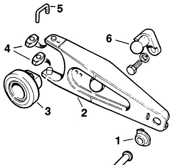
**Fig.2 Clutch release mechanism.**
