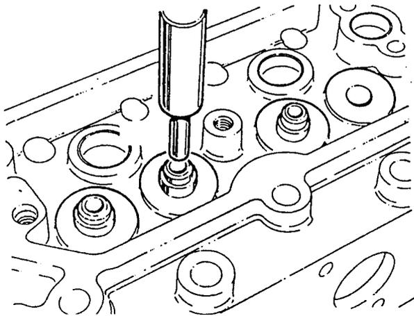
**Fig.11 Fitting valve guide.**
