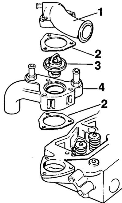
**Fig.3 Thermostat housing**
