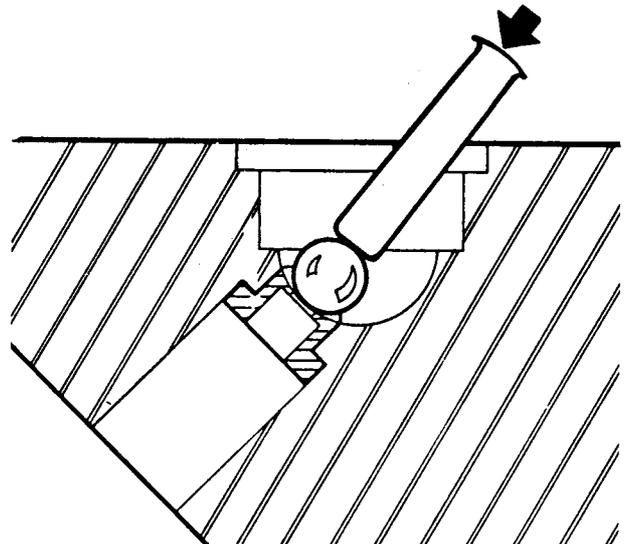
**Fig.6 Removing shroud**
