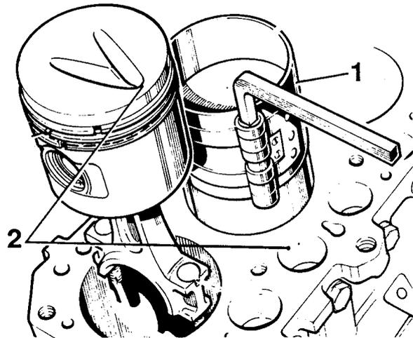
**Fig.29 Fitting piston and connecting rod assembly.**
