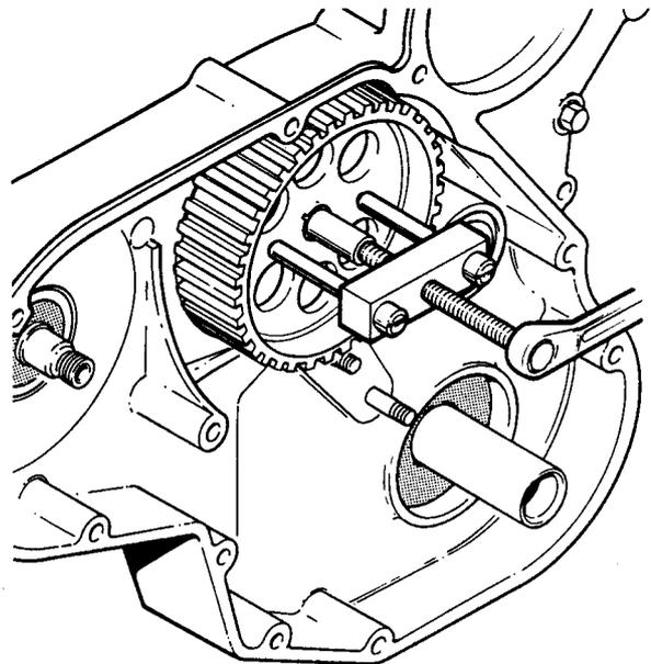
**Fig.5 Camshaft pulley removal with 18G 1464**
