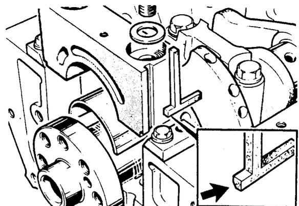
**Fig.27 Fitting rear main bearing cap (inset shows chamfer on the cork seal).**
