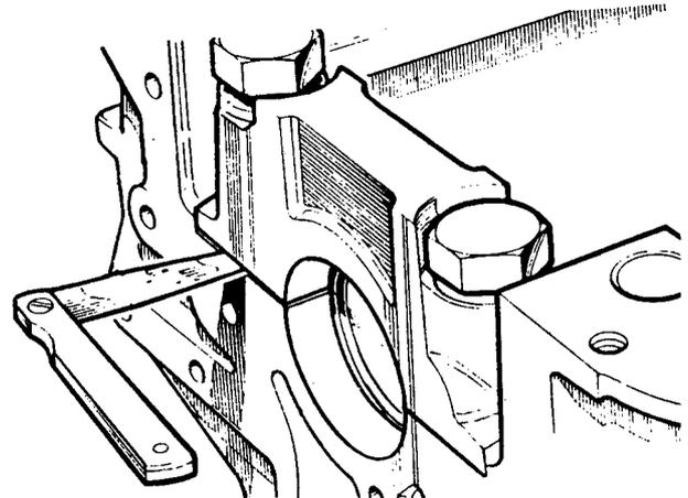
**Fig.20** Checking main bearing caps for distortion.
