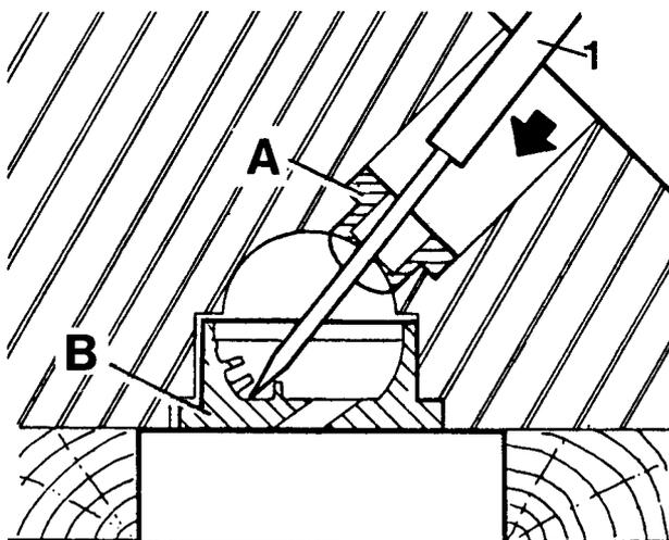
**Fig.5 Removing hot plug**
