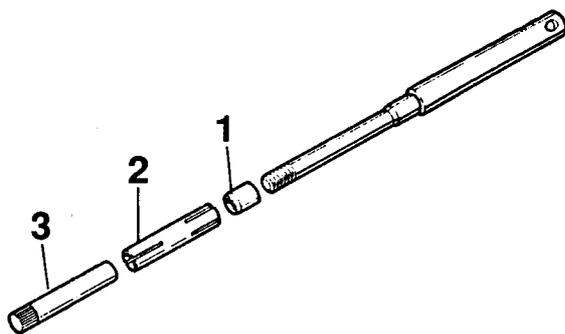
**Fig.12 Valve guide pilot.**
