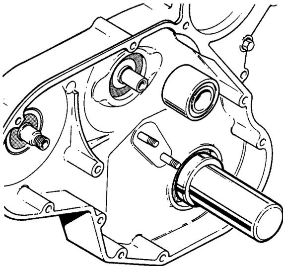
**Fig.6 Fitting crankshaft seal with 18G 1456**
