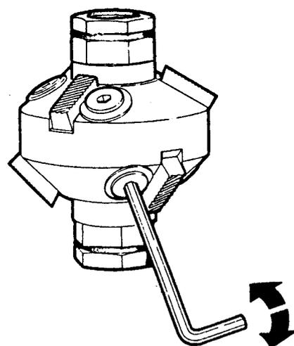
**Fig.14 Valve seat cutter MS 621.**
