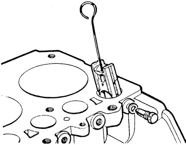
Fig.1 Removing tappets
