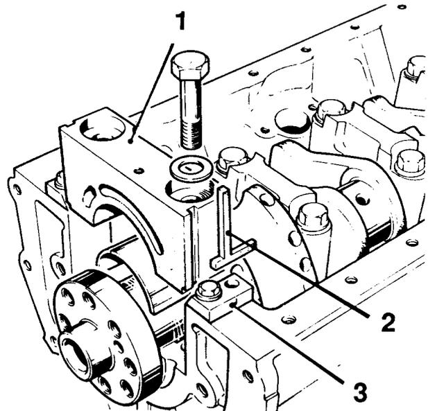
**Fig.26 Fitting rear main bearing cap.**
