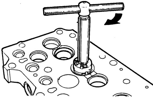
Fig.15 Cutting valve seat.
