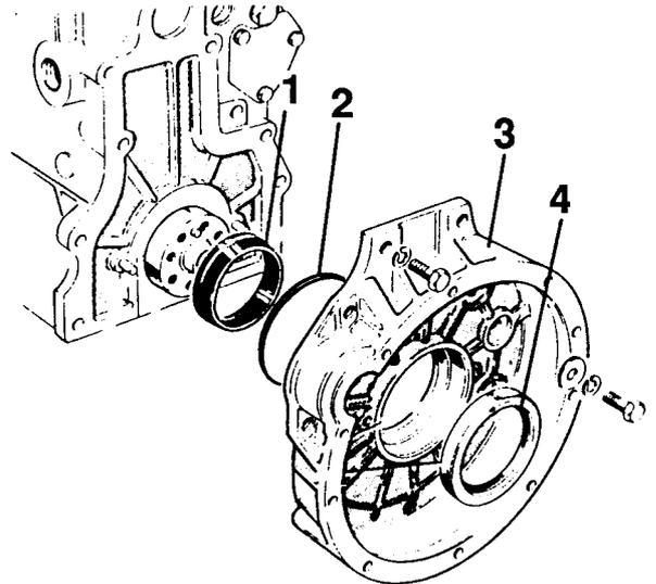
**Fig.7 Fitting flywheel housing**
