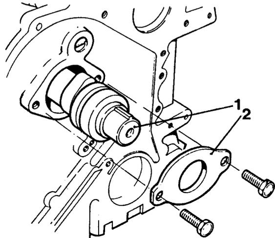
Fig.3 Removing camshaft
