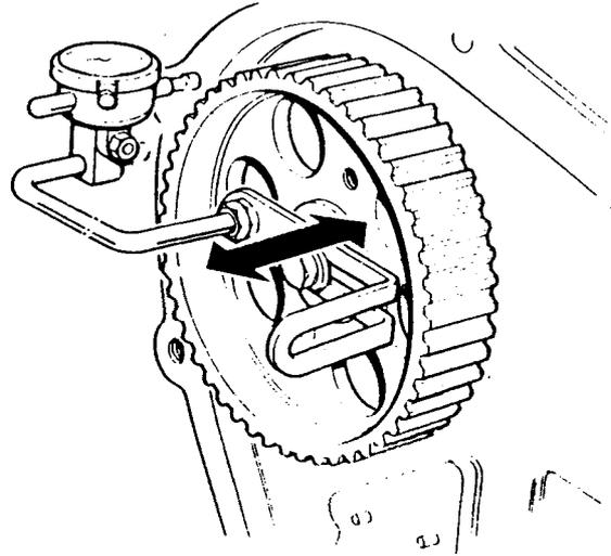
**Fig.32 Measuring camshaft end-float.**
