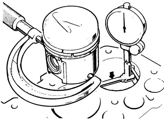
**Fig.12 Measuring piston and bore diameters.**
