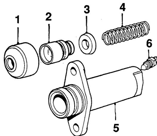
**Fig.5 Slave cylinder components**
