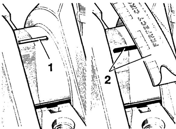
**Fig.23 Using Plastigage to measure bearing clearance.**
