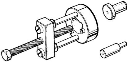
Crankshaft and camshaft pulley remover
