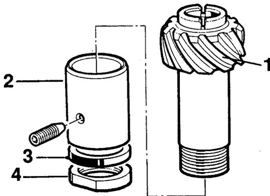
**Fig.5 Skew gear assembly**
