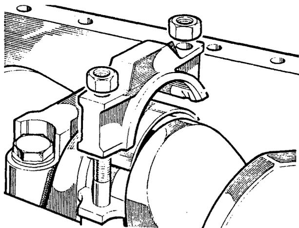
**Fig.10** Connecting rod cap and bearing.
