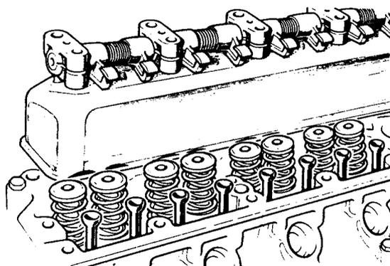
**Fig.1** Using the rocker cover to retain the rocker shaft assembly.
