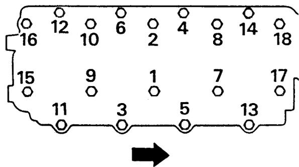
**Fig.23 Cylinder head tightening sequence.**
