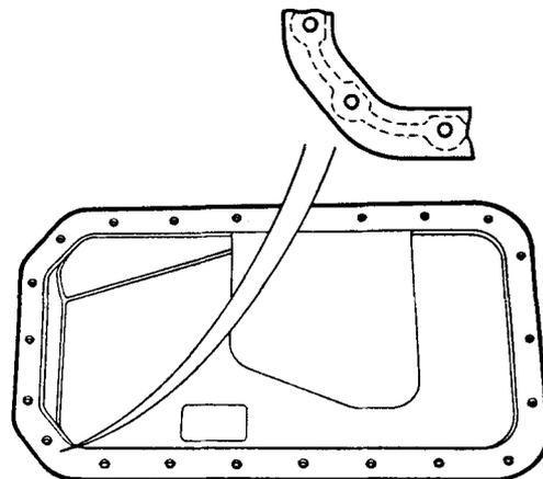
**Fig.34 Applying sealant to sump.**
