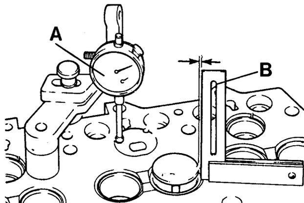
**Fig.8** A. Checking stand-proud of hot plug.
