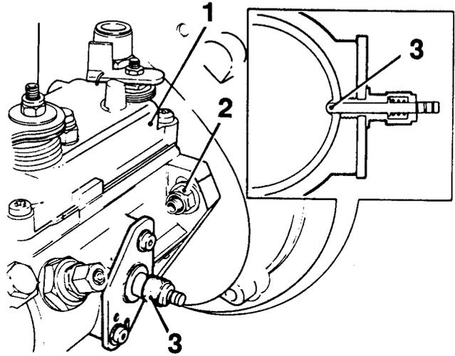
**Fig 5 Tool 18G 1458 in position**
