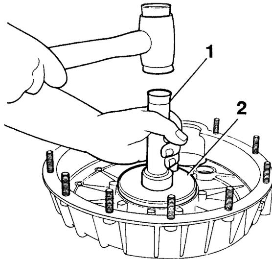
**Fig.5 Fitting crankshaft rear oil seal**
