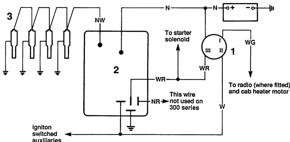
**Fig.6 Micronova System Circuit**
