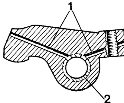
**Fig.21 Cross section through rocker**
