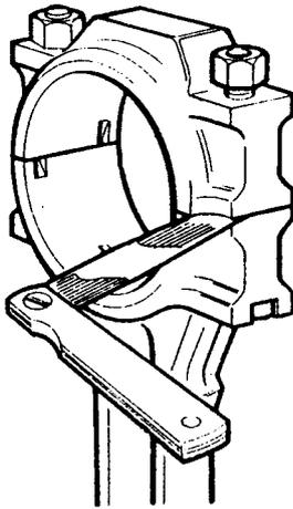
**Fig.16 Checking connecting rod/cap for distortion.**
