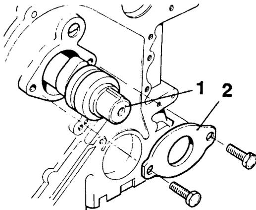
**Fig.31 Fitting camshaft.**
