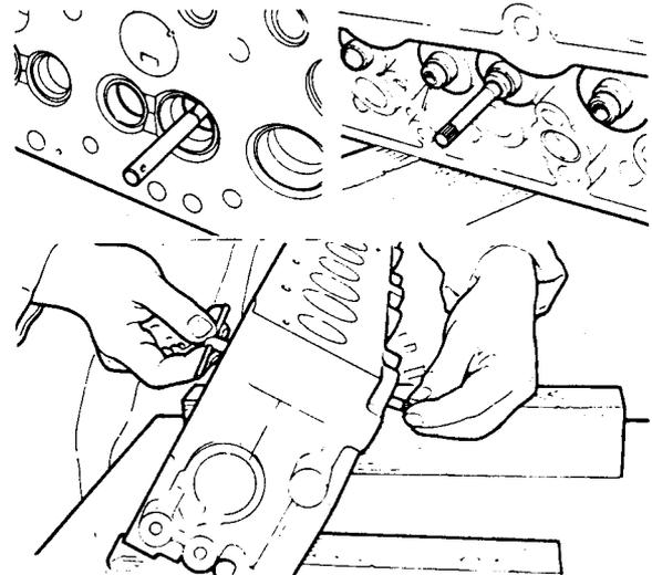
**Fig.13 Fitting valve guide pilot.**
