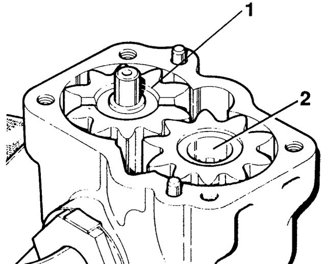
**Fig.9 Oil pump gears**
