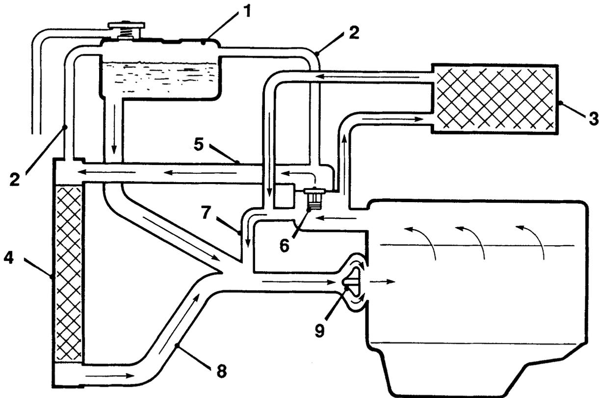
**Fig.1 Coolant circulation**
