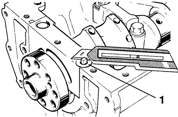
**Fig.28 Trimming cork seal.**
