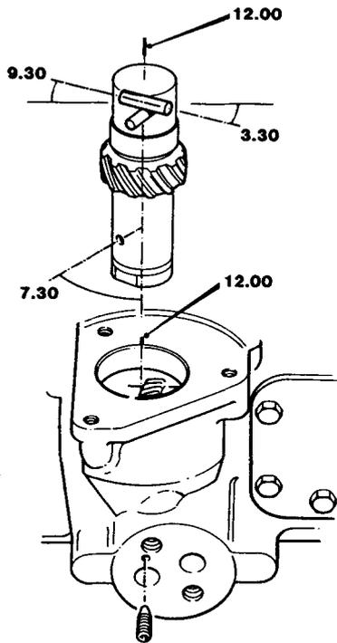
**Fig.33 Fitting the skew gear.**
