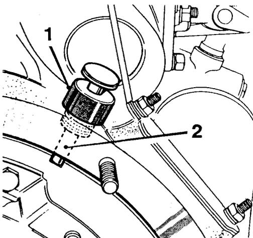
**Fig 3 Timing pin LST 107 fitted to flywheel housing**
