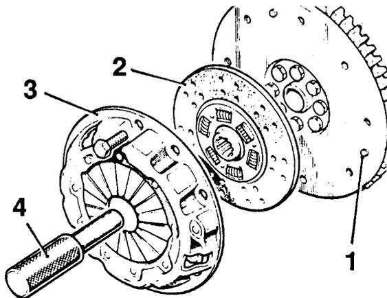
**Fig.3 Centralising the clutch plate**
