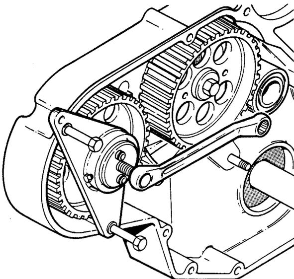
**Fig.4 Injection pump pulley removal with 18G 1457**
