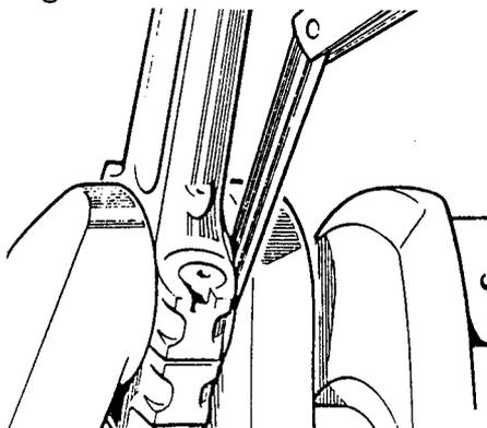
**Fig.18 Measuring connecting rod end-float.**
