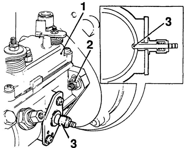
**Fig.12 Injection pump timing**
