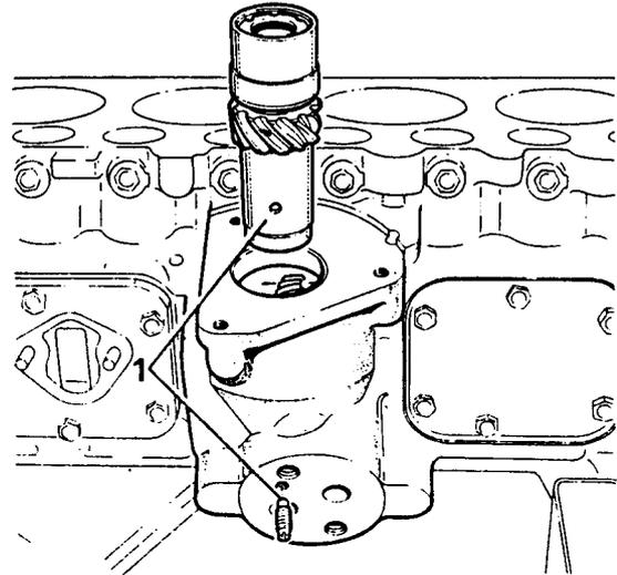
Fig.2 Removing skew gear
