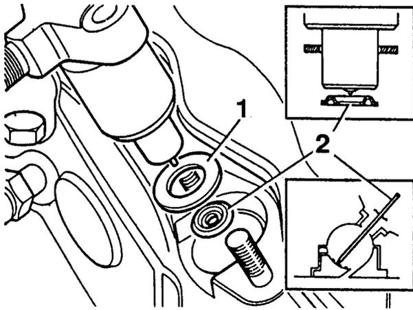
**Fig.19 Injector sealing washers**
