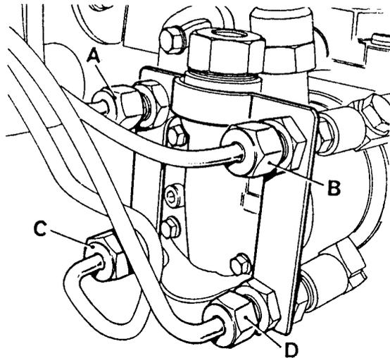
**Fig.26 Injector pipe fitting**
