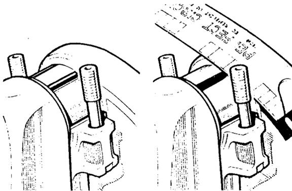
**Fig.17 Using Plastigage to measure bearing clearance**
