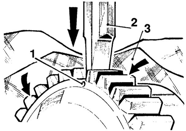
**Fig.2 Removing starter ring gear**
