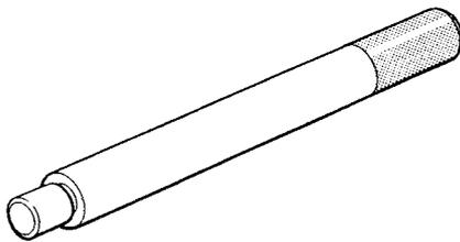
Exhaust valve guide remover
