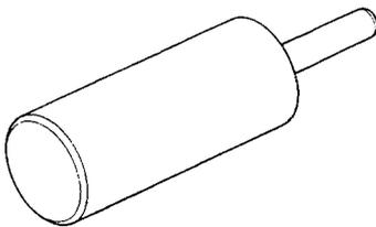
Inlet valve guide replacer
