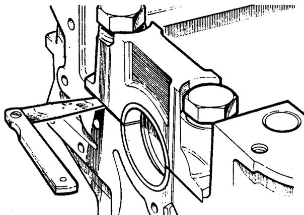
**Fig.22 Checking main bearing cap nip.**
