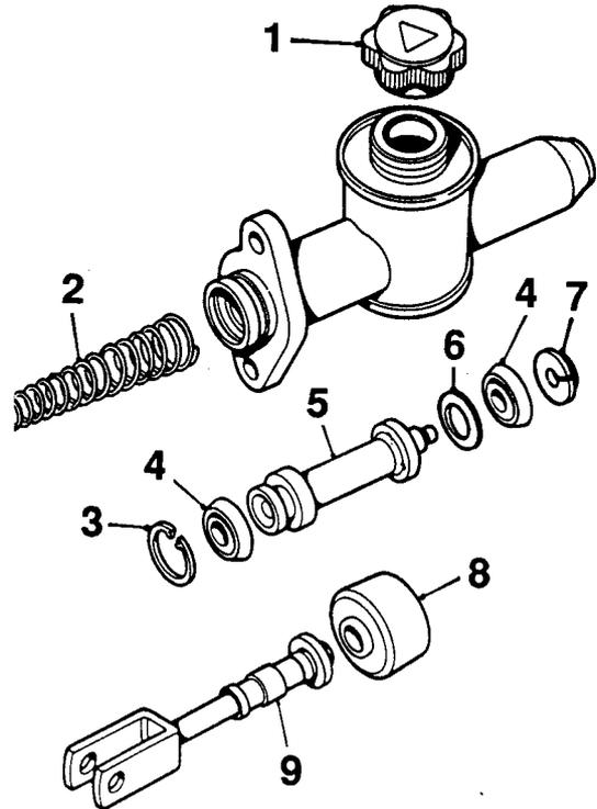
**Fig.4 Clutch master cylinder components**
