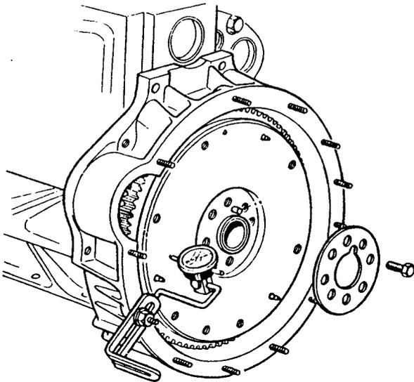
**Fig.4 Measuring flywheel run-out**
