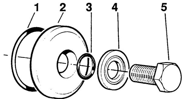
**Fig.8 Camshaft pulley fixing**
