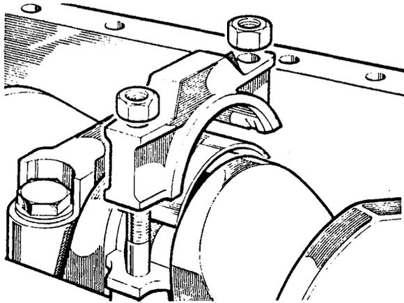
**Fig.30 Fitting connecting rod cap.**
