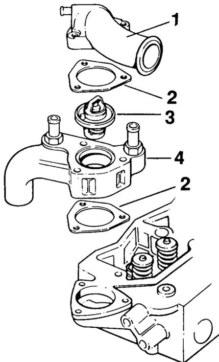
**Fig.3 Thermostat housing**
