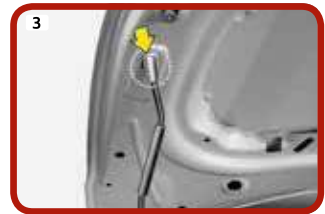
Release the support rod and insert it into the position shown.
