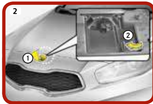
① Raise the bonnet slightly. ② Push the secondary latch inside and lift the bonnet.
