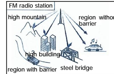
FM radio receives high frequency signals that can not bend with the earth curvature. So, FM radio can on-
