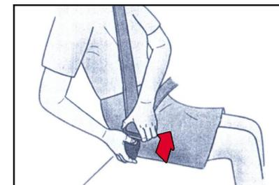
Press down the loosening button on the buckle. After being undone, the safety belt will return to expansion box automatically.
