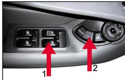
The power window can be operated only when the ignition key is in "ON" position. Each door has a power window switch to control window. Main switch of power window at driver seat can be used to control the passenger power windows. Pressing down switch (1) can open the cab window. The opening degree of window can be adjusted by switch. Lifting the power window
