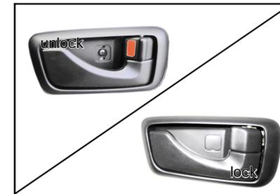
Put the button in the door to "LOCK" and "UNLOCK" position, you can lock and open the door. When the door is locked, the door lock inside and outside the vehicle can both be used.
