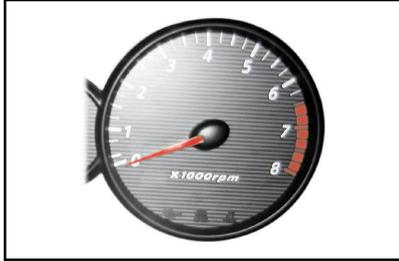
The tachometer indicates engine speed. Use the tachometer to select correct gear, avoiding use low gear or high gear at low speed.
