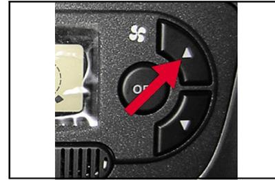
Pressing control button for fan speed can set the fan speed to appropriate value. Faster speed can provide higher air flow. Pressing "OFF" button can close the fan.
