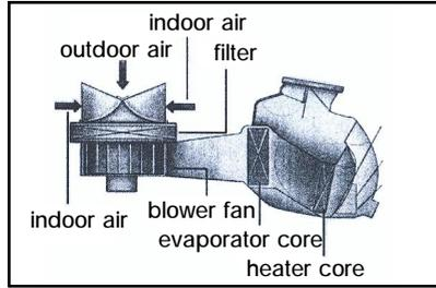
Air conditioner is inside of the evaporator, which is back of the glove box. This unit can reduce foreign materials that come into vehicle and filter with air.
