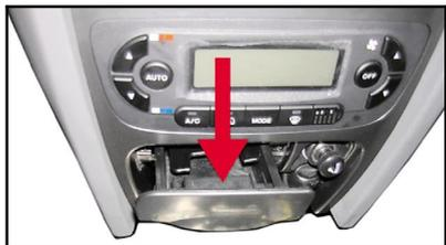
Pulling out catcher to open the ashtray in front seat. When you want to wash the ashtray, please push the storage box and move the ashtray forwards. Then you can take out ashtray. If you want to reinstall it, you should put it in correct position, then press it and move forwards, and align the rear edge of ashtray. Light of ashtray can illuminate only when the room light is on.
