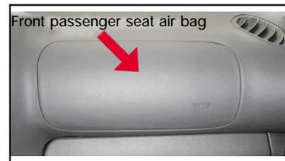
When the air bag expands, if the decorative cover is not open completely, the air bag can not operate normally. So the decorative cover should be open completely. Complete expansion of air bag and the use of safety belt can reduce the forward impacting speed of the driver
