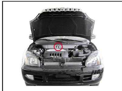
You may use the VIC to register your vehicle and handle legal affairs about it. The VIC is located in the vehicle identification code panel of the fire wall between the engine and driver cab.
