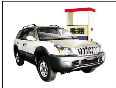
JAC vehicle can only use unleaded gasoline above 93#. If you use leaded gasoline, the catalytic sensor will be damaged and more maintenance cost will occur. To avoid using leaded gasoline by mistake, do not insert nozzle carrying leaded gasoline into the fuel tank.
