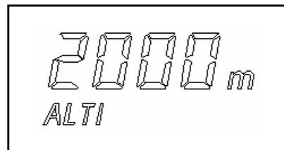
Height measuring gauge is displayed as "ALTI data (m)" in operating mode. Its measuring range is 200~2,800m. With regard to corrected height (displayed in operating
