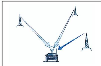
◆ Change service station -- After FM signal becomes weak, the frequency that is near to the vehicle and has stronger signal begins to act. This is because your radio more easily receives clear signal. In such case, please choose other service station with stronger signal.
