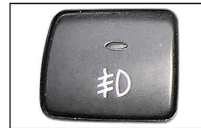
Press the switch to turn on the rear fog lamp. When the headlight switch is in second position and the ignition key is in "ON" position, the rear fog lamp will illuminate.
