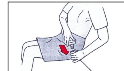
Tie the two-point static safety belt, and insert the tongue into the buckle until you hear a "ka" sound. Check the locking condition and for knot of safety belt.
