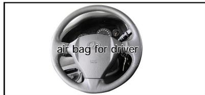
Your vehicle is installed with auxiliary protection (air bag) system. Its name is "SRS AIR BAG", which is written in air bag cover of steering wheel and above the glove box of front passenger seat.
