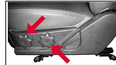
Turning the front adjusting button can adjust the seat cushion facing front of vehicle. Turning the back adjusting button can adjust the seat cushion facing back of vehicle.
