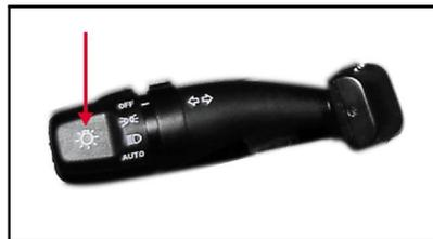
Move the switch to the last position of multifunctional switch to turn on the headlight. First position of the switch is for parking light, side light, tail light and panel light. Second position of the switch is for headlight.
