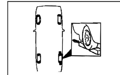
After the vehicle is lifted by the jack, it is necessary to place tire stops in the front and rear side of the tire diagonal to the ruptured tire to prevent it from rotating.
