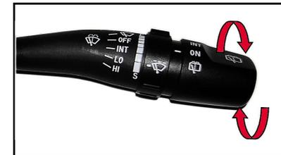
To use the cleaner, pull the control lever towards steering wheel. After operating the control lever, the cleaner will operate automatically. After releasing it, it will stop.
