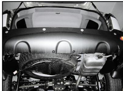
4. Lift the hanger, lower the hanger and remove the spare tire.
