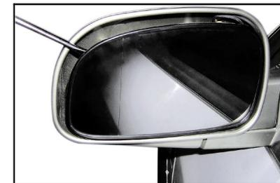
Pushing the mirror towards vehicle can fold the mirror. By that way, the vehicle can be parked in narrow place
