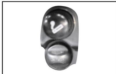
To use the cigarette lighter, press and then release it immediately. When it becomes hot, it will jump up automatically, and then you can use it. If the engine is not started, the cigarette lighter can not be used unless the ignition switch is in "ACC" position. To avoid damaging the socket or fire, do not use counterfeit accessories.
