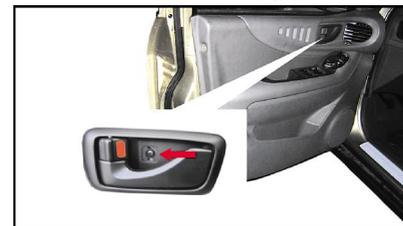
Without using the key, put the button in the door to "LOCK" position (to the rear side of the vehicle), and when the red warning light of switch is off, the door can be closed. Under the condition that front door is closed and the key is in the ignition switch, do not lock the door.
