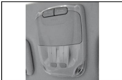
When the ignition key is in "ON" position, you can open or close the skylight. If you want to open or close it, please press and hold the console button at the top. According to the said method, you can adjust to ideal position.
