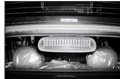
Low rear brake light is installed on both sides of the vehicle, and high brake light is installed in the middle of the vehicle. When you step brake pedal, these lights will illuminate.
