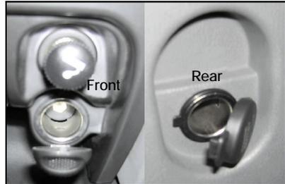
These sockets can supply power of 12V voltage. Thus, all kinds of electrical accessories and equipment can be run.
