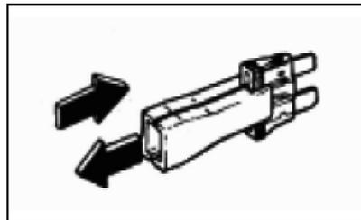
3. It is necessary to check all fuses, regardless whether burnt fuse has been identified.
