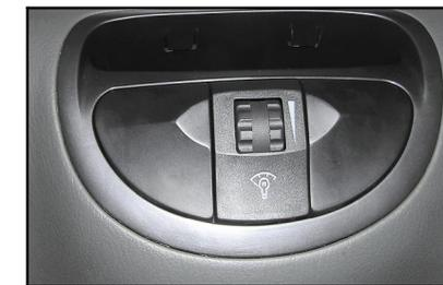
Turning the control button of panel light can adjust its brightness.
