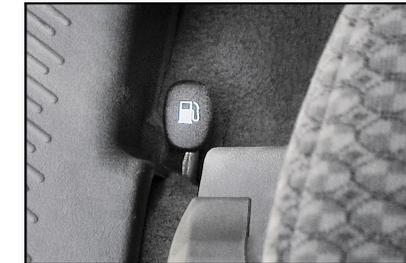
Pull up the release rod (on the floor) in the left front corner of driver seat and open the filler cap.
