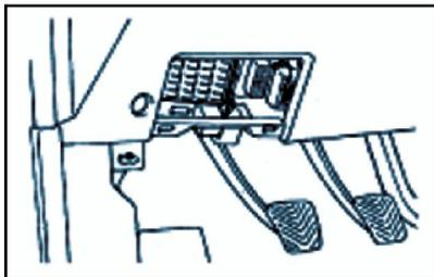
Below the driver position instrument panel are provided the fuse box for
