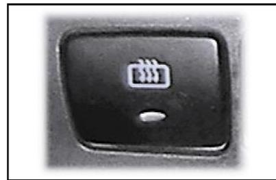
Press the switch to turn on rear window defroster. At the same time, the rear defroster indicator will illuminate.
