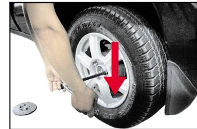
To fit the wheel cover again, place the nuts on studs and tighten them. Swing the wheel gently to confirm if it has been safely fixed, and tighten the nuts with hands again.
