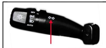
Moving the signal lever up and down to send lane-changing signal. After releasing it, the signal lever will return to middle position.
