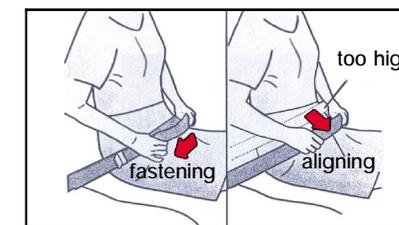
Two-point static safety belt must be manually adjusted to appropriate length. Tie the safety belt. The safety belt should be lowered to buttocks but not haunch. If too high, it will cause hurt during accident
