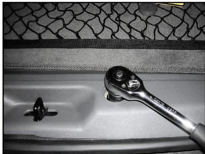
3. Loosen the bolt with the wheel nut spanner
