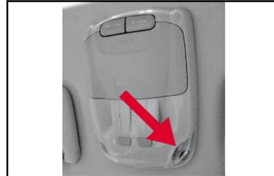
Press the reading light switch to turn it on or off. The reading light can be used to light in night or be used as private light of the driver or passenger.
