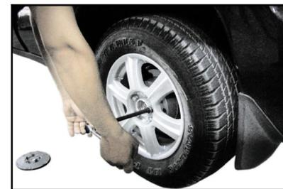
The following is about replacement of a ruptured tire. When it is necessary to replace a ruptured tire, confirm that the transmission is set to the reverse gear (manual transmission), and the parking brake is applied. Af-
