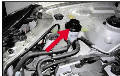
The power steering oil level should be inspected periodically.
