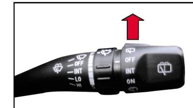
Push the control lever of wind shield wiper and cleaner upwards to operate the defroster.
