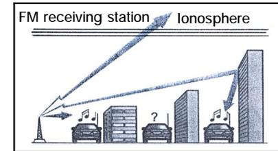
AM and FM signals are sent from transmitting stations around the city. After the antenna of the radio receives the signal, the sound will be sent out from microphone. If high signal touches your vehicle, the radio can operate exactly. If the signal is low or unclear, it may be related to the distance, and related to the building, bridge and other structures that block off signal.
