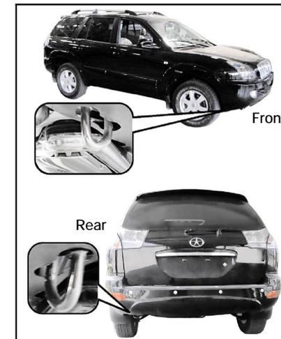
If no professional towing vehicle is available, tie the towing cable chain or lifting lever on the bottom hook at the front of the vehicle, and tow the vehicle in emergency. Operate with
