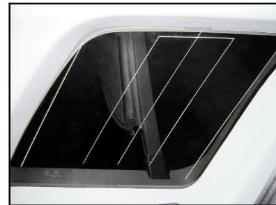
When the ignition key is in "ON" or "ACC" position, if you turn on the radio, the vehicle will receive AM and FM signals from rear side glass.
