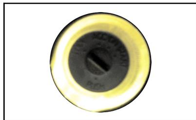
When the door is open, the ignition switch will illuminate to inform you that the ignition switch is not in "ON" position. When the door or the igni-
