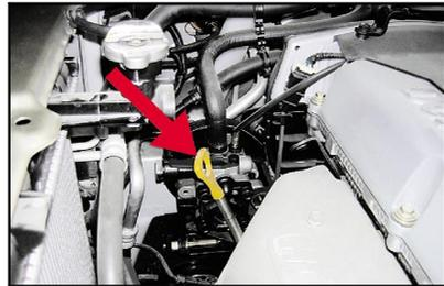
Before check the engine oil, warm up the engine to normal water temperature and park the vehicle on a flat ground. Turn off the engine and wait
