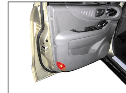
After opening the front door, the red light will illuminate. The aim of this light
