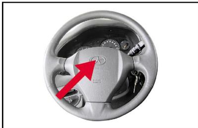
Pressing the steering wheel gasket, you can hear the sound of the horn.
