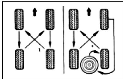
Wheel shifting shall be performed every 10,000km. If uneven wearing is found after shifting, have the JAC dealer check the vehicle for timely correction.
