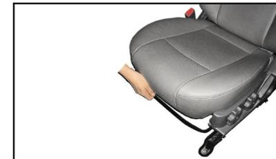
If you want to move the seat back and forth, please lift the adjusting lever of seat and hold it. Slide it to the desired position, then release the lever and confirm locking of the seat.
