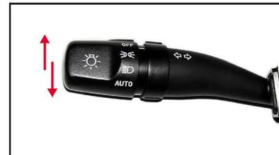
To change headlight beams, pull the switch control lever towards yourself and then release it. Even with the
