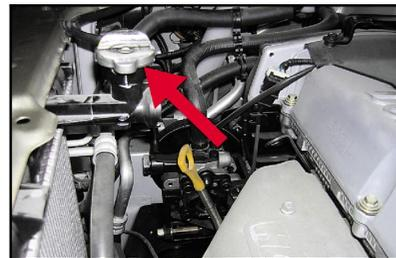
Use an ethylene or ethylene glycol cooling liquid with water at a mixture ratio of 50/50. The engine cooling liquid should be compatible with the parts of aluminum alloy engine. Never use additional inhibitor or additive. The cooling system should use engine cooling liquid with correct concentration and anti-freezing and anti-corrosion performance. Do not use a cooling liquid solution
