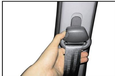
Adjust the shoulder harness to appropriate position. If the safety belt is near your neck, you can not be protected safely. The safety belt should be across the middle section between chest and shoulder.
