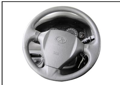
To inspect the free travel of steering wheel, park the vehicle with four wheels straight to the front, and lightly turn the steering wheel to the rear and outward. Hold the steering wheel with hands lightly and operate the steering wheel flexibly according to the resistance marked on the free travel range. If the free travel has exceeded the normal range, have it checked by the JAC dealer, and adjust or repair the steering wheel when necessary.
