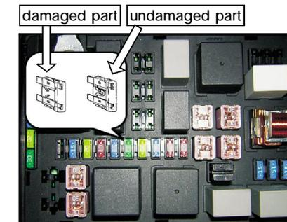
The fuse will be blown when the system current exceeds the specified range. Therefore, it is necessary to prevent damage to wires. (The cause is normally system short-circuiting or excessive high load). If this is not the cause, ask the JAC dealer to determine the cause.
