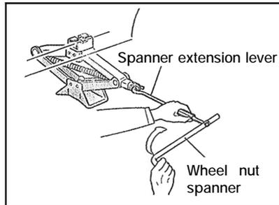
Fit the jack handle at the position shown. To raise the vehicle, turn the handle clockwise. Confirm the position of the jack when jacking the vehicle to avoid it sliding down. If the jack is placed on a soft ground or beach, a suitable plate is needed and should be placed at the bottom
