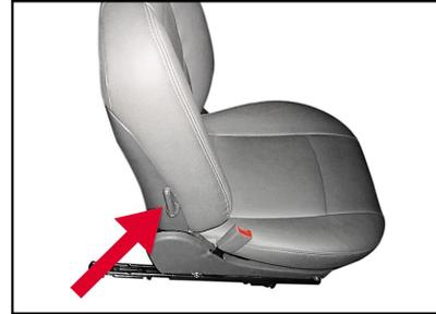
Adjusting the seat back control, in order to increase weight of seat back, put the adjusting rod to rear position.
