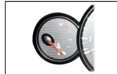
If the engine overheats, do not open the water tank cover; otherwise serious scald will occur. So, you can not open the water tank cover until the engine returns to normal temperature.
