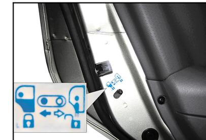
Your vehicle is equipped with child safety lock in rear door. You should lock the rear door, to ensure that it can not be opened from inside. This manual recommends using this device with child in the rear seat. To ensure that it can not be opened from inside, you must press the child safety lock in the rear door to "🔒" position. If you want to open the
