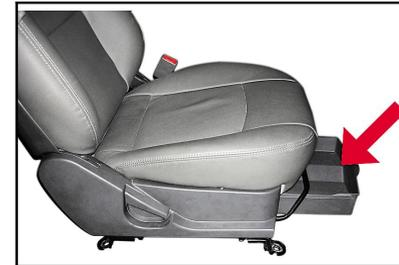
Storage tank is installed under the co-driver seat. Pulling forward can open the storage tank.
