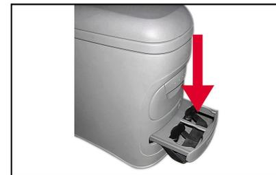
In order to fix water cup or drink tin, the cup holder in rear seat is installed on the main console of rear seat. You can use it by pressing the
