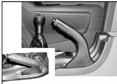
After parking the vehicle, you must use hand brake. When the ignition key is in "ON" or "START" position, hand brake indicator will illuminate. Before driving, you must release hand brake and confirm if the indicator extinguishes.
