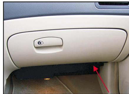
The glove compartment is equipped with locking core. You can lock and unlock the glove compartment by the ignition key. To open the glove compartment, just pull upward the glove compartment handle when the compartment is at unlocking position.
