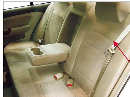
The rear seat is equipped with three-point type safety belt.
