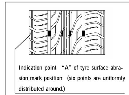
You can determine when to replace the tyre according to the abrasion indication mark on the tyre surface. When the tyre surface is worn and its thickness is 1.6mm or below, the abrasion indication mark on the tyre surface will appear.
