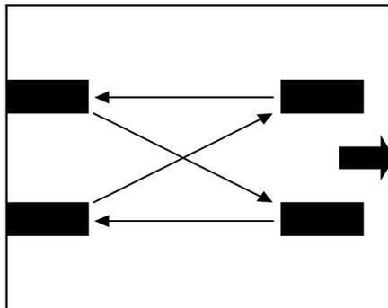
When rearranging the tyre, make sure that rearrange the tyre in proper mode shown in the figure.
