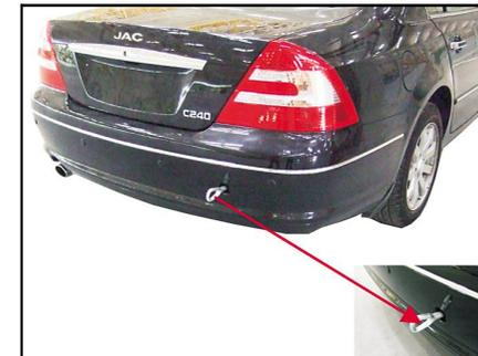
Tow the other vehicle with rear towing hook. The rear towing hook can be used in emergency only (for example, tow the vehicle trapped in the ravine, snow or slough).
