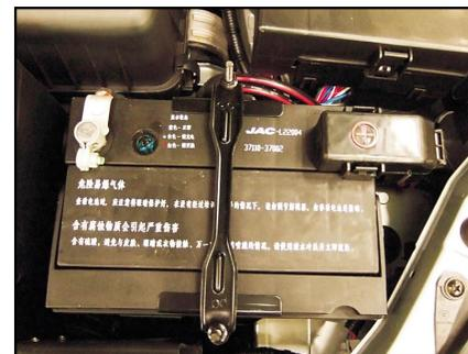
There is maintenance free storage battery installed in your vehicle. If you want to replace the storage battery, the part number on volume of all the storage battery shall be the same with that of the original storage battery. See “General Drawing of Engine Cabin” in this section to confirm the position of the storage battery.
