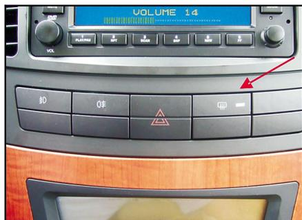
Your vehicle is equipped with a rear window and exterior view mirror defroster, which can operate only when the ignition switch is switched on.
