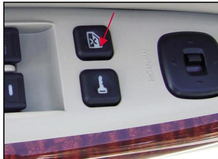
The electric window control device of the driver's also includes a locking button. When the locking button is pressed down, the front and rear passengers cannot use their window switches. The driver can still operate all the windows at locking condition. Press the locking button once again and the normal operation of windows will be resumed.
