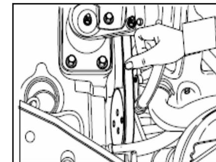
Inspecting the rate of tension of the transmission belt:
