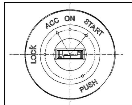
Insert the key into ignition switch, you can turn the key to four different positions.
