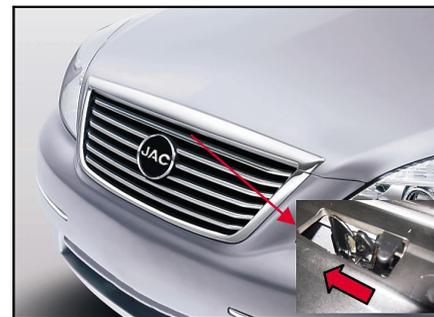
2. Extend your hands to the front lower side of the engine cover and turn the engine cover release bar leftward.
