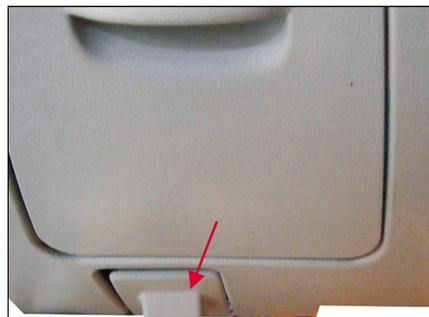
1. Pull the engine cover release bar at left lower side of console.
