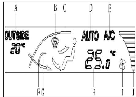
Your vehicle is equipped with automatic temperature control system. This system allows you to control the refrigeration, heating and ventilation of vehicle.
