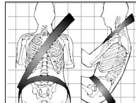
The position of the hip belt part should be downward as much as possible and stick closely to the rump; it should just contact the thigh, in such a case, the acting force will be applied onto the firm pelvis when collision accident happens. Besides, the possibility of the slide under the hip belt can also be reduced. If you slide under the hip belt, the hip belt will put force to your abdomen, which may
