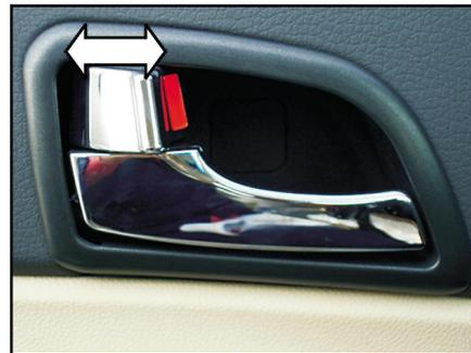
To lock any door inside the car, you should toggle the door lock control button right inward.
