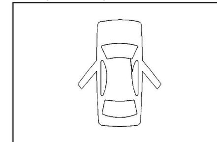
If one of the doors is not properly closed, the door ajar warning light on the combined device will light on until the door is well closed.
