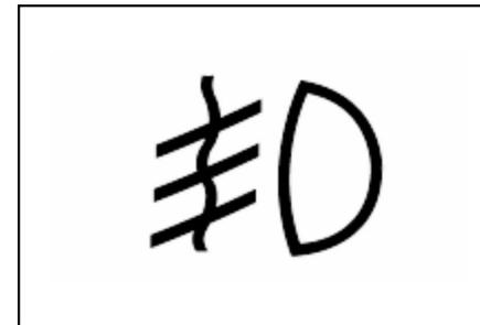
Press the front fog lamp button on the mid switch group assembly of instrument desk, the front fog lamp will be connected and the indicator light on the button will light on. At the same time, the front fog lamp indicator light on the combined device will light on. Press the button once again and the front fog lamp will distinguish.
