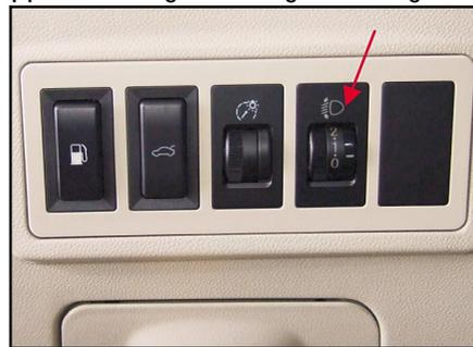
The fourth switch on the left switch group assembly on the instrument desk is the dimming switch of headlight which could adjust the illumination angle of the dipped beam light and high beam light. Toggle the thumbwheel switch of the dimming switch upward to upper the beam of dipped beam light and high beam light and vice versa.
