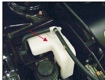
The engine coolant expansion pot is located in the engine cabin beside the vehicle passengers. The detailed position, see “General Drawing of Engine Cabin”.
