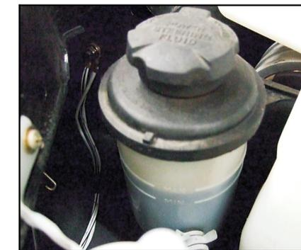
The level shall be between the upper limit MAX mark and lower limit of the stock solution tank.
