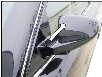
Push the exterior rearview mirror backward to the car and you can fold the mirror and put it flatly on the side surface of the car.
