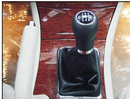
To shift the gear, please depress the clutch pedal completely, turn the gear shift lever to required gear and release the clutch slowly.
