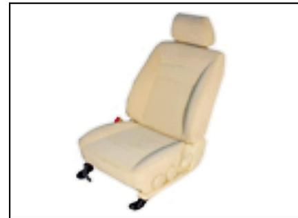
Pull up and fix the operating lever in the front below the seat, you can cancel the locking condition of the seat.
