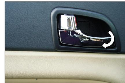
To open the door from inside of the car, pull the door handle inwards.
