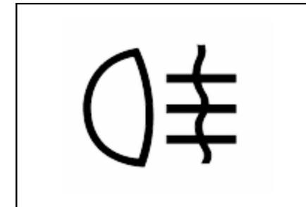
When the front fog lamp is on, press the rear fog lamp button on the mid switch group assembly of instrument desk, the front fog lamp will be connected and the rear fog lamp indicator light on the combined device will light on. The indicator light on the button will light on.
