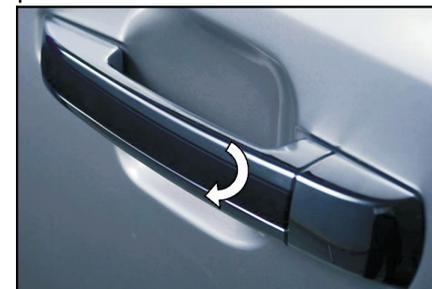
To open the door from outside of the car, pull up the door handle outwards.
