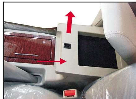
The central control console has two independent storage areas and the upper storage hatch is also an armrest. To open the upper storage hatch, just pull up the armrest cover plate at the upper layer. To open the lower part storage hatch, just lift the lower starting wrench and raise the hatch cover. To close the
