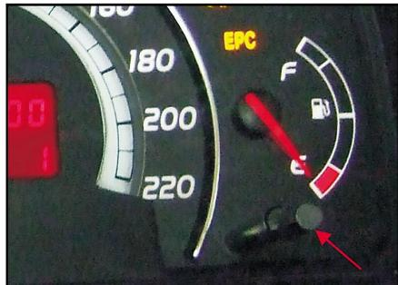
The reset lever can be used to shift among modes, adjust time and reset the odometer. When operating the shift display modes, one must press it in short time (>300ms and <2s).
