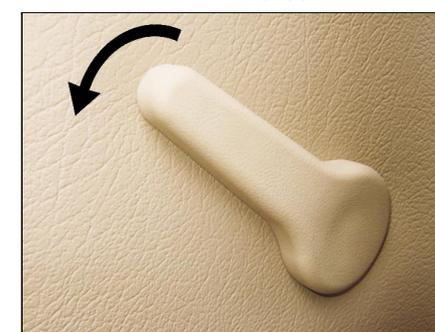
To adjust the waist rest of the driver's seat, please use the control lever at exterior side of the seat backrest.
