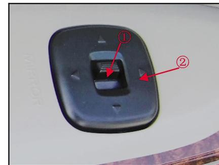
The control switch of electric back mirror locates at the front door switch panel at the driver's side.
