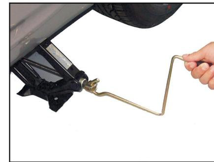
7. Rotate the jack handle clockwise to raise the vehicle until the lifting head is inserted into corresponding notch firmly and the tyres are about 3cm above the ground.
