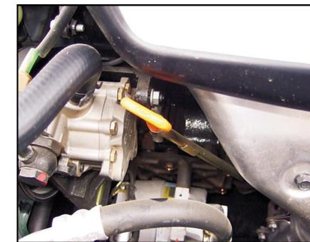
You’d better check the engine oil when filling oil. The oil should be cooled in order to get accurate reading.
