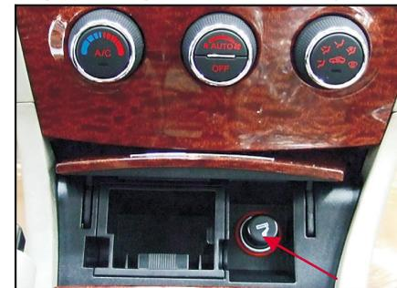
The front cigarette lighter and ash tray locate at the lower part of the central console with an integrated protective cover. Press at the bright stripe ornament part on the cover and then release, the protective cover will open automatically. To take out the front ash tray for cleaning, pull out the ash tray and pour the ash. When reassembling, just push the ash tray back.
