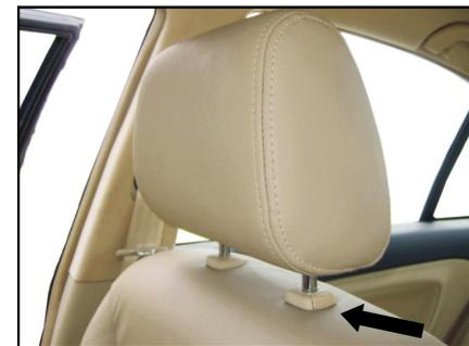
Descend: While pressing down the lock-release button, press the pillow down. To dismount the pillow, please fully pull up the pillow, and then press the release button and lift the pillow from inside the guiding sleeve.
