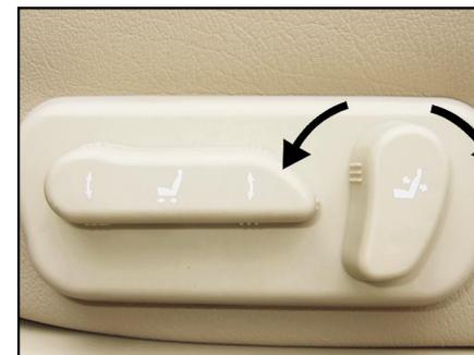
Push the switch on the upper side forward or backward, you can adjust the inclination of the seat backrest.
