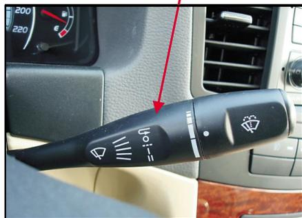
Operate the front windshield wiper by using the control lever at the right side of the steering column. The ignition switch must be connected to operate the wiper. Clearance: turn the handle downward to the 1st shift and select one cycle of delayed wiping and washing. Low: turn the handle downward to the 2nd shift and you can conduct stable
