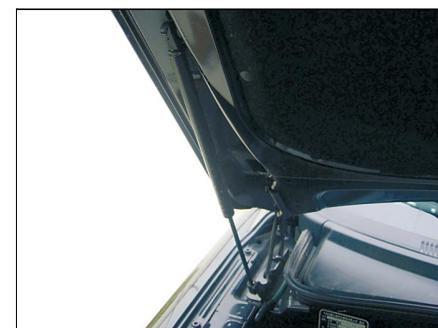
3. Lift the engine cover to the highest point (air operated outrigger support).
