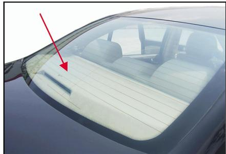
It's located at the rear window defroster and equipped with AM-FM antenna. Ensure there is no scratch on the internal surface of rear window and the grid line on the rear windscreen is not damaged. If the internal surface of rear window is damaged, it may interfere with radio receiving signal. In addition, to ensure normal receiving signal of radio, the antenna signal amplifier in rear right C pil-
