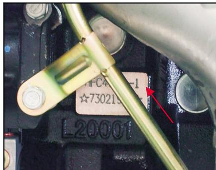
Engine No. is printed on the cylinder block at the upper position of the engine.
