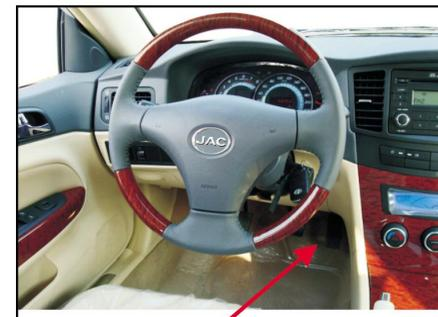
There is an interior temperature sensor in the lower left side plate of instrument desk, which reads the interior air temperature and helps to establish ventilation system demand under AUTO mode.
