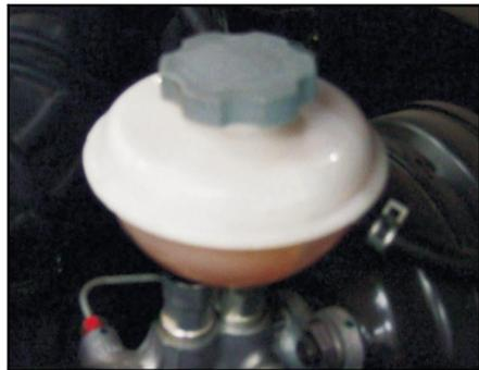
When it is required to add brake fluid, you can only use JG4 brake fluid and can only use new brake fluid in unopened container. See “Main Fluid Parameters” in section II.
