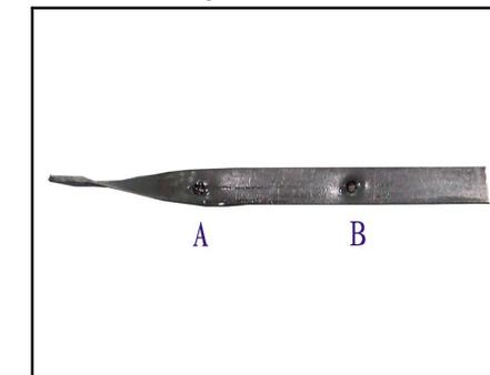
4. If the oil level is at the position of mark hole (A) at the lower part of the oil rule or lower than this position, you should fill oil. In this section, we will show which oil type shall be used.
