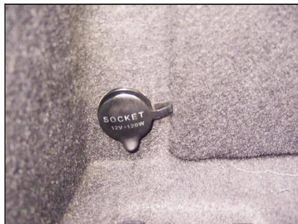
Your vehicle is equipped with an accessory power supply socket. You can connect the accessory electrical equipment through accessory power supply socket. The accessory power supply socket is in the trunk. To use the power supply socket, remove the protective cover first. When the socket is not used, make sure to close the protective cover. The
