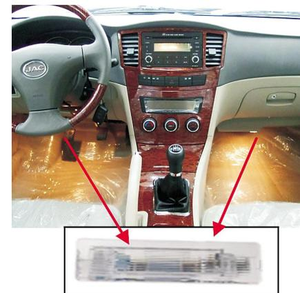
It's located at the driver and copilot feet position for feet lighting.
