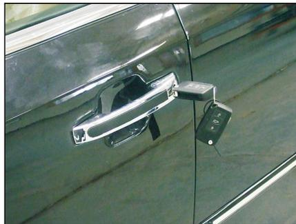
To lock the door with key outside the car, you should insert the key and turn it clockwise.
