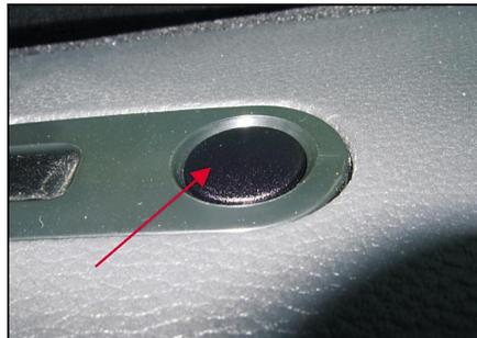
The sunshine sensor monitors the quantity of sunshine radiation and performs necessary adjustment on temperature, fan speed and air delivery system basing on this information to maintain the selected temperature.
