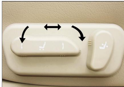
If your car is equipped with this device, there will be a multi-direction adjustment electric seat control device at the exterior side of driver's seat.
