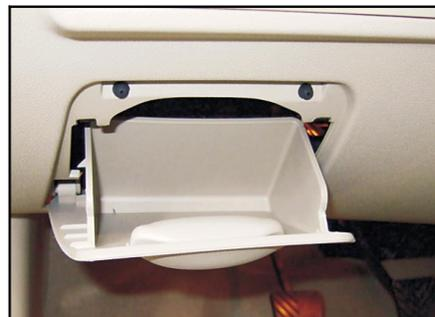
The storage box at driver’s side locates at the console at the left side of steering wheel. It is used as the interior fuse check mouth as well. To use it, just pull out the storage box or take it out.
