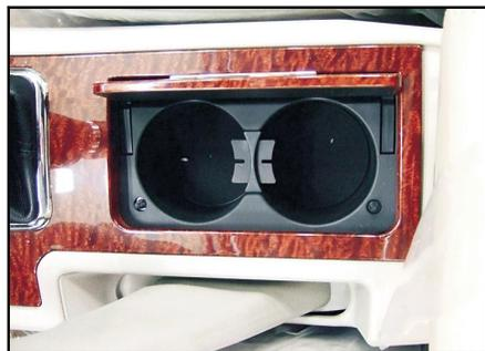
The cup support locates at the auxiliary fascia console and rear seat armrest. To use the front cup support, press the bright stripe ornament part of the cup support protective cover and then loosen, the cover will open automatically. To use the rear cup support, pull down the central handle at rear seat (refer to the next page “Rear Seat Armrest”).
