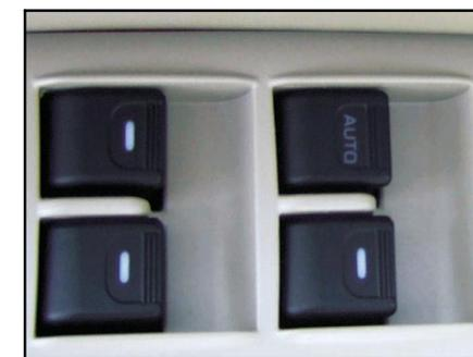
The switch of electric window locates at the door handle at the driver's side. In addition, each passenger door is equipped with their individual window switch.
