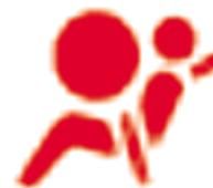
There is an airbag ready indicator lamp on the combined meter of instrument panel, which displays the airbag symbol. The system will check whether airbag system has fault. For details, refer to Airbag Ready Indicator Lamp in Chapter Three.
