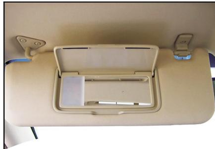
Each sunroof is equipped with a vanity mirror, which contains a small light for your lighting. You can turn the mirror upward to use the vanity mirror. When you close the cover, the small light will be off automatically.
