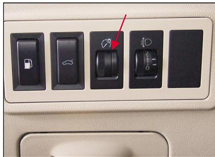
The third switch on the left switch group assembly of instrument desk is the dimming switch which can adjust the brightness of the light on the console. Toggle the thumbwheel switch of the dimming switch upward to increase the brightness of the light, and vice versa.
