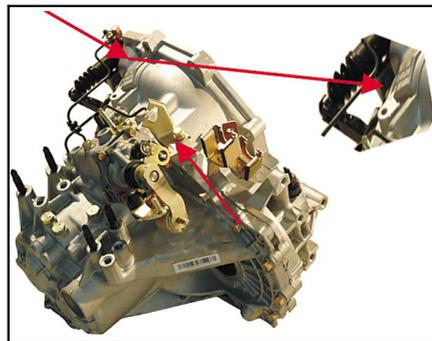
MT Identification No. is at the connection end between the transmission and clutch.
