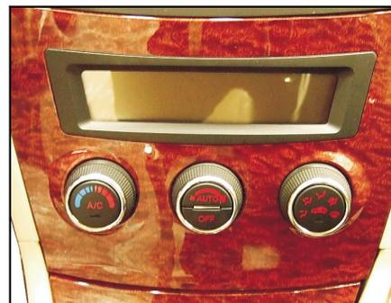
**AUTO** (automatic): press AUTO button to enable automatic control over internal air temperature, air delivery mode and fan speed. Then, the AUTO mode indicator will present on the display.
