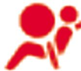
There are two airbag ready indicator lights on the combined device of the console, the airbag signs display on the lights.
