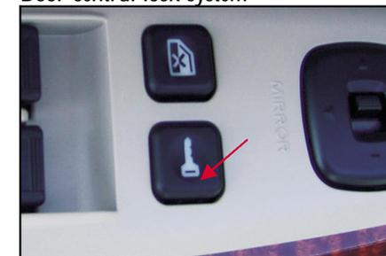
The electric door lock buttons on the door switch of driver's side can control the opening and closing of all the four doors. By pressing the electric door lock's central switch button, the four doors will be locked. Press down the central control electric door lock switch button, the four doors will be opened. If the car speed exceeds 40km/h, the door lock will be automatically locked.
