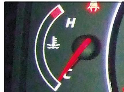
Indicating the water temperature of the engine. When the pointer reaches the red area, the car must be stopped for overhaul, preventing the engine damage. It should not be restarted until the water temperature decreases. If such similar fault still exists, please promptly contact with the special service center of Jianghuai Automobile Company.
