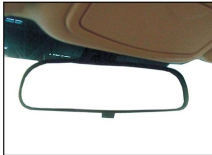
The inner back mirror can be adjusted upward, downward, leftward and rightward. Adjust the daily and night vision of the mirror by using the inner rearview mirror adjust rod. This adjustment will reduce the glare of the headlight at the back of your car.
