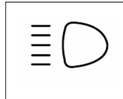
When you want to change the headlight from dipped beam to high beam, you should push the turning signal/multi -function control lever opposite you.
