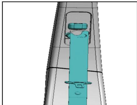
Before you drive the vehicle, move the adjuster of the shoulder belt to the proper height. Adjust the height to have the shoulder belt part be in the middle of your shoulder. The shoulder belt should be away from your face and neck but can not slide under the shoulder. Lower the shoulder belt, press down the
