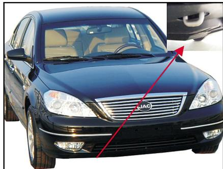
The front towing hole is located under the front guard. There shall be a driver in the vehicle to control steering and braking.
