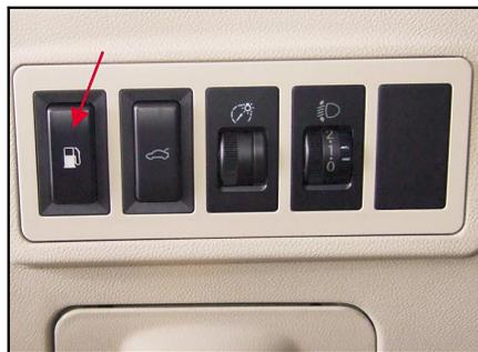
Press the oil tank cover switch on the left switch group assembly of instrument desk, and you can open the oil tank cover.
