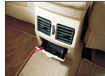
The rear ash tray locates at the rear part of auxiliary fascia console. Pull out the rear ash tray for cleaning. When re-assembling, just first clamp it on the bottom tongue and then push it back.
