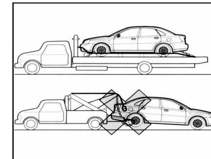
5. The front wheels must be off the ground during vehicle towing.
