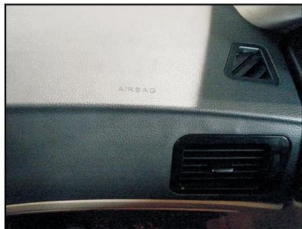
Your vehicle has been equipped with two airbags, one is the frontal airbag for the driver, and the other one is the frontal airbag for the right front passenger.
