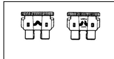
In the figure above, the LH fuse is operative and the RH is defective. Use a fuse piler to replace the defective fuse with the same sized one.
