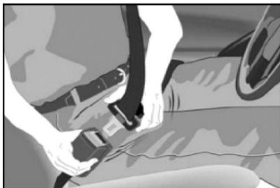
Pull the webbing attached to the latch plate over the chest and pelvis. Lock the latch plate in the buckle and examine it manually, where an expected "click" sound means successful engagement.
