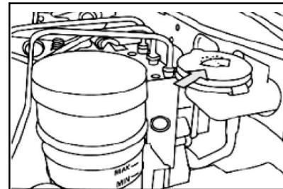
A partially highlighted engine bay layout is shown in the figure. The washing reservoir is fitted at the left of the engine bay. Make sure there is adequate liquid in the washing reservoir and the windscreen washing unit shall be examined for its performance.
