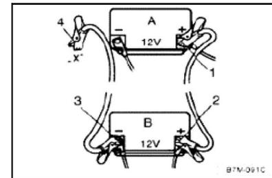
When it is impossible to start your engine due to a low battery, you can use another battery from the other vehicle through auxiliary wire to start it. Follow the points described below:
