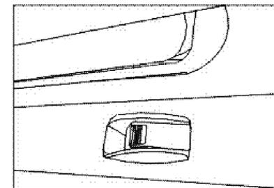
Individual switches are provided additionally at the occupant's door and rear doors (See figure above).
