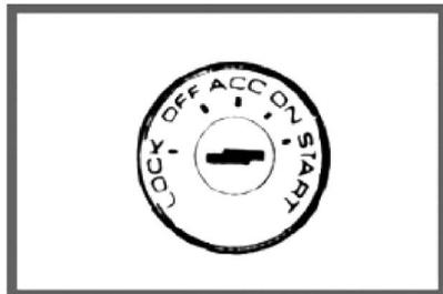
"LOCK": this position allows the key to be inserted or removed from the ignition switch.
