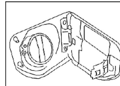
The filling pipe is attached to rear RH cover.
