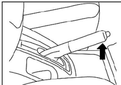
Lifting up handbrake forcibly while parking. The first gear may be selected if parking on a steep surface. The braking light will illuminate when the handbrake is engaged and the ignition switch is on. To release the handbrake, gently lift the lever and push the lock button inward (as shown in figure) and press the handle fully to its rest position.
