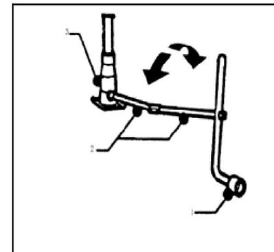
Lock the component 3 as indicated and then connect the components 2 and 1. Rotate as indicated direction to raise or lower the jack to fulfill desired operations. When the jack has been lowered to its lowest point, component 3 can be released and take away easily.
