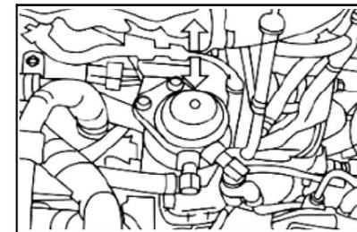
Push the upper button on the oil-water separator up and down to discharge air trapped in the circuit, which is a crucial operation.
