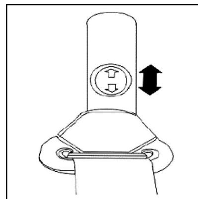
Use belt height-adjusting device to adjust and get your desired frontal sash height. Jerk the belt to examine whether belt elements are operative.
