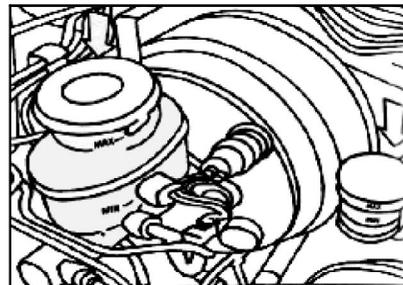
Examine the brake performance and whether there is any leakage at joints and whether the level of oil cup meets requirements. Examine the clutch performance and any leakages.
