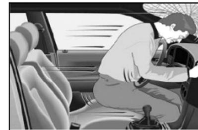
In case of frontal collisions, an occupant without a seat belt could be thrown forward, totally uncontrolled and being hit by interior parts such as steering wheel, instrument panel and windshield. A thrown-out may be possible in some cases, which could be fatal!
