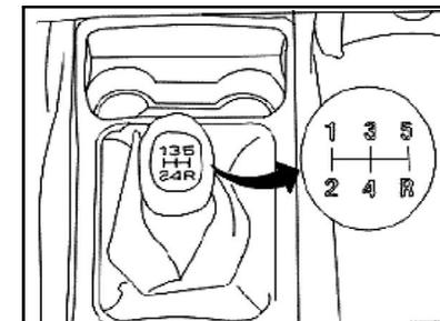
Do not select the reverse gear until the vehicle comes to a full stop. Fully press the clutch pedal when the engine is running, wait a moment to avoid abnormal noises from gear shifting. The reverse light will illuminate when the reverse gear is selected and the ignition switch is turned to ON Position. Do not rest your hand on the gear
