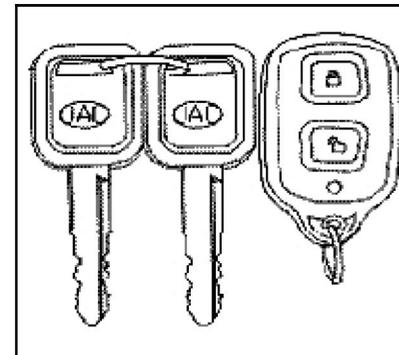
Each pick-up comes with three keys, two for mechanical operation and one for remote control. Also the key number and pin are provided at back of the RC key.
