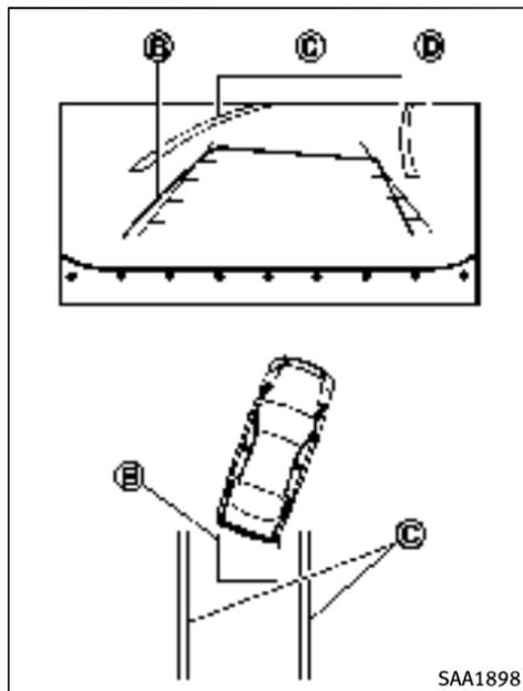
3. Slowly back up the vehicle adjusting the steering wheel so that the predictive course lines (B) enter the parking space (C).
