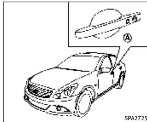
When you carry the Intelligent Key with you, you can lock or unlock all doors by pushing the door handle request switch (driver's or front passenger's) (A) within the range of operation.
