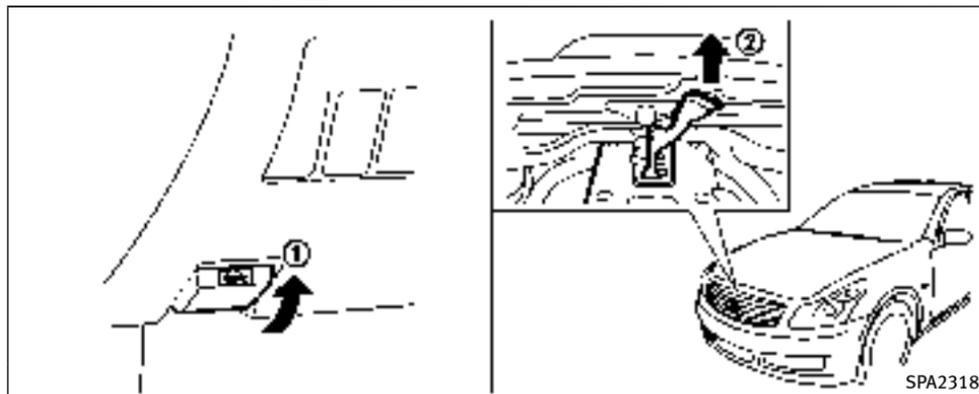
1. Pull the hood lock release handle ① located below the instrument panel; the hood will then spring up slightly.
