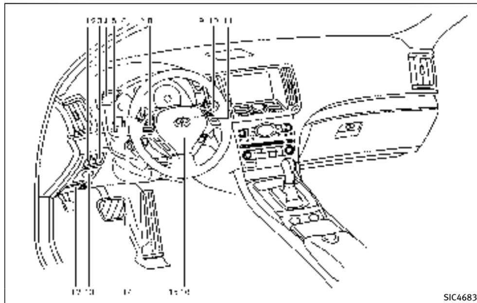
1. Vehicle Dynamic Control (VDC) OFF switch (P.5-58)
