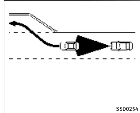
When driving on the freeway at a set speed and approaching a slower traveling vehicle ahead, the ICC will adjust the speed to maintain the distance, selected by the driver, from the vehicle ahead. If the vehicle ahead changes lanes or exits the freeway, the ICC system will accelerate and maintain the speed up to the set speed. Pay attention to the driving operation to maintain control of the vehicle as it accelerates to the set speed.
