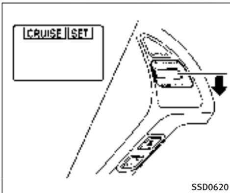
**To set cruising speed**, accelerate your vehicle to the desired speed, push the COAST/SET switch and release it. (The SET indicator will come on in the display.) Take your foot off the accelerator pedal. Your vehicle will maintain the set speed.
