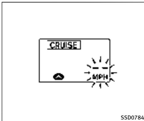
When the COAST/SET switch is pushed under the following conditions, the system cannot be set and the ICC indicators will blink for approximately 2 seconds:
