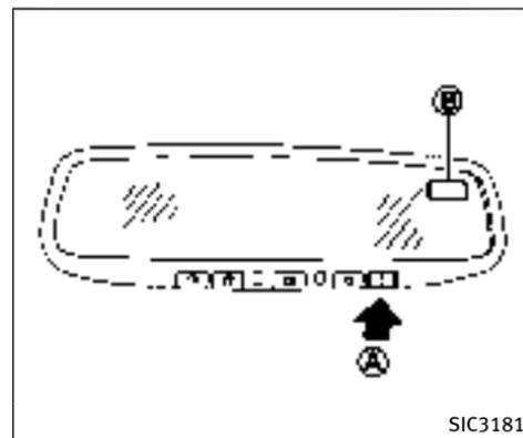
When the ignition switch is pushed to the ON position, the compass display
