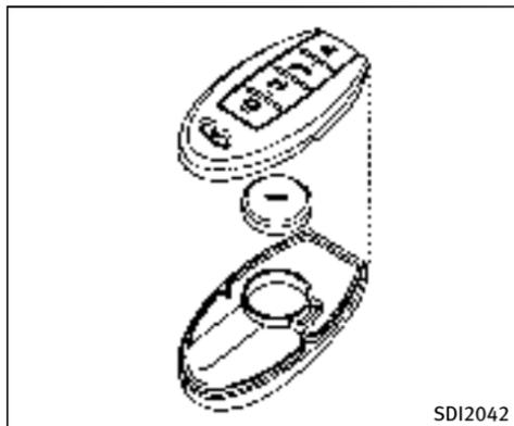
3. Replace the battery with a new one.
