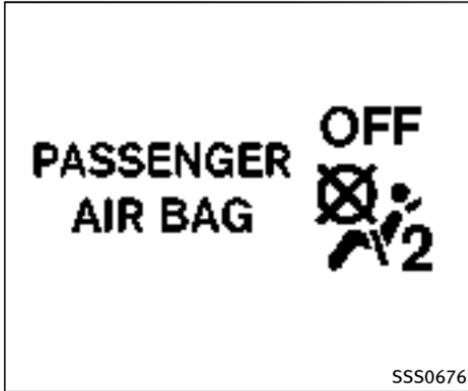
7. If the booster seat is installed in the front passenger seat, push the ignition switch to the ON position. The front passenger air bag status light
