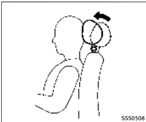
Active Head Restraints operate only in certain rear-end collisions. After the collision, the head restraints return to their original positions.
