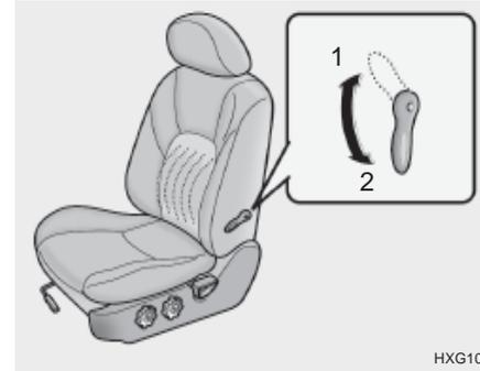
To adjust the lumbar support, turn the handle on the outboard or left side of the seat. To increase the amount of lumbar support, pull the lever forward. To decrease it, push the lever toward the rear.
