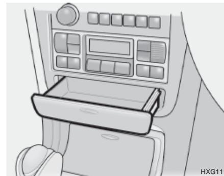
The accessory box may be opened by pushing at its top edge. It is used for storing small commodities.
