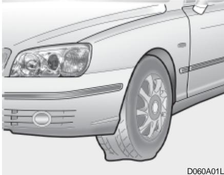
The procedure described on the following pages can be used to rotate tires as well as to change a flat tire. When preparing to change a flat tire, check to be sure the gear selector lever is in "P" (automatic) or reverse gear (manual transaxle) and that the parking brake is set, then:
