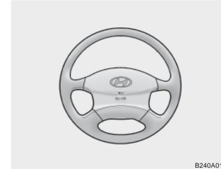
Your Hyundai is equipped with a Supplemental Restraint (Airbag) System. The indications of the system's presence are the letters "SRS AIR BAG" embossed on the airbag pad cover in the steering wheel and the passenger's side front panel pad above the glove box.
