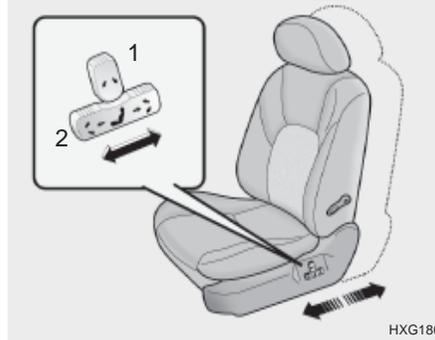
Pull the control knob forward or backward to move the seat forward or backward to the desired position. Release the knob and then the seat will remain at that position.
