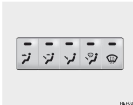
This is used to direct the flow of air. Air can be directed to the floor, dashboard outlets, or windshield. Five symbols are used to represent Face, Bi-Level, Floor, Floor-Defrost and Defrost air position.
