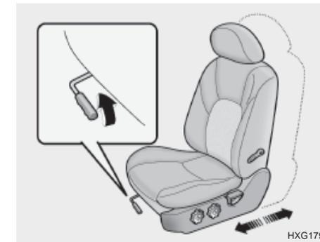
To move the seat toward the front or rear, pull the lock release lever upward. This will release the seat on its track so you can move it forward or rearward to the desired position. When you find the position you want, release the lever and slide the seat forward or rearward on its track until it locks into the desired position and cannot be moved further.
