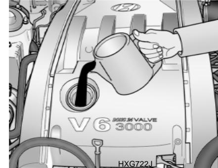
If the oil level is close to or below the "L" mark, add oil until it reaches the "F" mark. To add oil:
