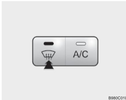
When the "Defrost" button is pressed, the "☃" mode will be automatically selected and the air will be discharged through the windshield defrost vents. To assist in defrosting the air conditioning will operate if ambient temperature is higher than 3.5°C and automatically turns off if the ambient temperature drops below 3.5°C.
