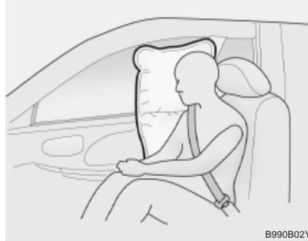
Your Hyundai is equipped with a side airbag in each front seat. The purpose of the airbag is to provide the vehicle's driver and/or the front passenger with additional protection than that offered by the seatbelt alone. The side impact airbags are designed to deploy only during certain side impact collisions, depending on the crash severity, angle, speed and point of impact. The airbags are not designed to deploy in all side impact situations.
