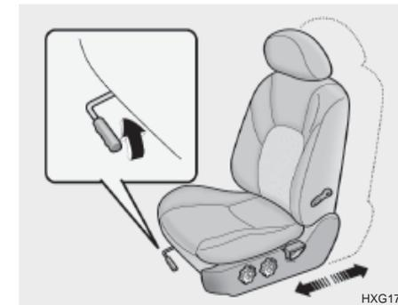
To move the seat toward the front or rear, pull the lock release lever upward. This will release the seat on its track so you can move it forward or rearward to the desired position. When you find the position you want, release the lever and slide the seat forward or rearward on its track until it locks into the desired position and cannot be moved further.
