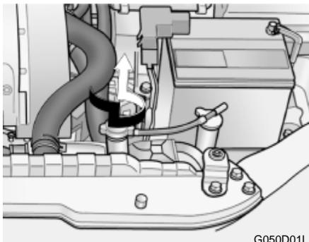
4. Turn the radiator cap counterclockwise without pressing down on it, until it stops. This relieves any pressure remaining in the cooling system. And remove the radiator cap by pushing down and turning counterclockwise. Now fill the radiator with clean demineralized or distilled water. Continue to add clean demineralized or distilled water in small quantities until the fluid level stays up in the radiator neck.
