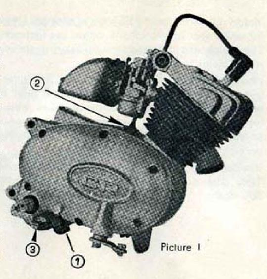
Motor: it is lubrificated by oil mixed with gas. Apart from the running-in period, for which special instructions follow, use fuel mixture with 5% oil SAE 30. The clutch and the inner transmission gears are lubrificated by the shaking of the motor housing oil (18 oz.).
