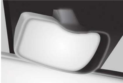
This mirror, placed on top of the central mirror, enables the driver or front passenger to observe all the rear seats. Fitted on its own ball joint, its manual adjustment is simple and provides a view of the rear interior of the vehicle. It can also be adjusted for improved visibility during manoeuvres or when overtaking.
