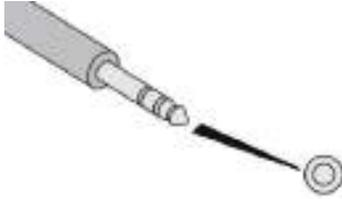
Connect a portable device (MP3 player, etc.) to the auxiliary Jack socket using an audio cable (not supplied).
