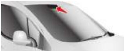
Using a laser sensor located at the top of the windscreen, this system detects a vehicle running in the same direction or stationary ahead of your vehicle.
