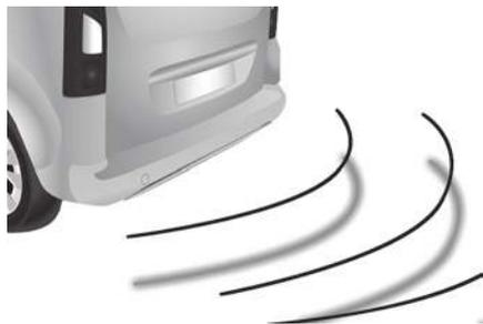
An audible signal confirms the activation of the system by engaging reverse gear.
