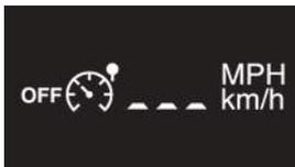
☞ Turn the knob to the **LIMIT** position. The speed limiter is selected but is not yet active. The display shows the last programmed speed.
