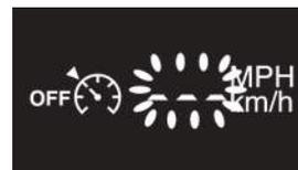
The programmed speed is cleared, then replaced by three dashes. Contact a CITROËN dealer or a qualified workshop to have the system checked.
