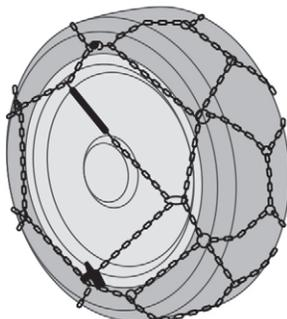
**!** The snow chains must be fitted only to the driving wheels. They must never be fitted to "space-saver" type spare wheels.
