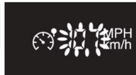
Pressing the accelerator pedal in order to exceed the programmed speed will have no effect unless you press the pedal **firmly** beyond the **point of resistance**.
