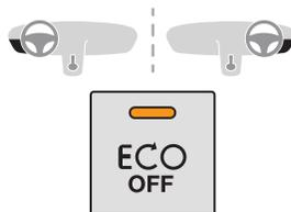
In the event of a malfunction with the system, the **ECO OFF** switch indicator lamp flashes, then comes on continuously.
