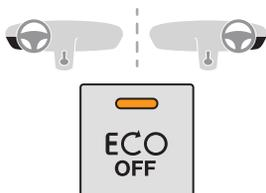
☞ At any time, press the "ECO OFF" switch to deactivate the system.
