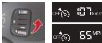
☞ Place the knob at the **0** position or switch off the ignition to switch the function off.
