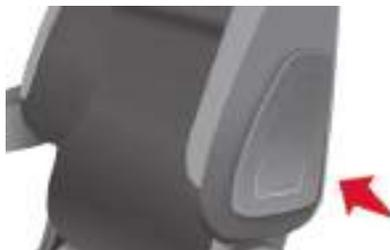
Each lateral airbag is fitted in the front seat's backrest frame, door side.
