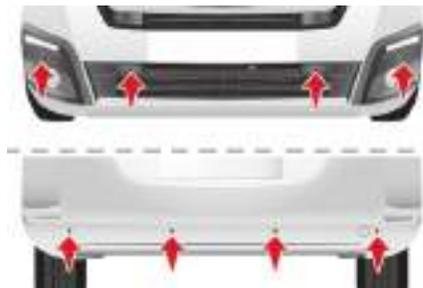
The audible (front and rear) and/or visual (rear) parking sensor system consists of proximity sensors installed in the bumpers. They detect any obstacle which enters the field of vision (person, vehicle, tree, fence, etc.) behind the vehicle during the manoeuvre.
