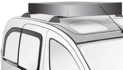
In all cases, the load must rest on the non-slip bands provided for this purpose, and must not touch the roof or the glazing on the roof.
