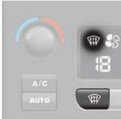
In this case, select the visibility program. The visibility program indicator comes on. It activates the air conditioning, the air flow, and provides optimum distribution of the ventilation towards the windscreen and side windows. It deactivates the air recirculation.
