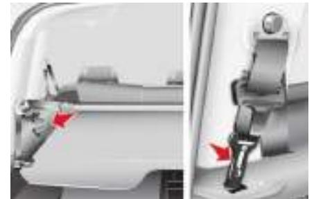
The row 3 seat belts which are not in use can be stored to clear the load space and to make use of the load space cover easier. Hook the spring hook into the location provided on the rear pillar trim.
