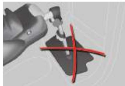
**!** Do not place the support leg on the storage compartment cover, as it could break during a violent impact. Where the adjustments of the support leg allow it, we suggest two other installation options.
