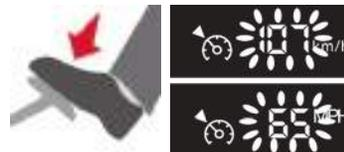
It is possible to **accelerate** and drive momentarily at a speed faster than the programmed speed. The programmed value flashes.
