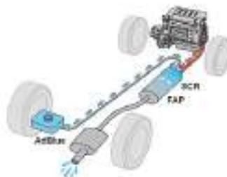
To respect the environment and ensure compliance with the Euro 6 standard, without adversely affecting the performance or fuel consumption of diesel engines, CITROËN has taken the decision to equip its vehicles with a system that associates SCR (Selective Catalytic Reduction) with a diesel particle filter (DPF) for the treatment of exhaust gases.
