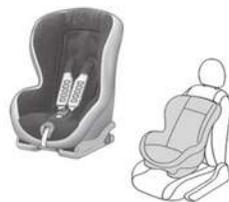
Installed only in the "forward facing" position. Attaches to rings **A** and ring **B**, referred to as the Top Tether, using an upper strap.
