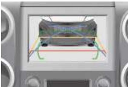
The representation with overlaid lines helps with the manoeuvre. They are represented as lines marked "on the ground" and do not indicate the position of tall obstacles (for example: other vehicles, etc.) relative to the vehicle. Some distortion of the image is normal.
