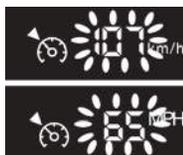
If the vehicle speed is higher, the programmed speed is displayed flashing.
