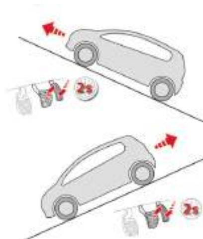
With the brake pedal and clutch pedal pressed, from the time you release the brake pedal, without using the parking brake, you have approximately 2 seconds to move off before the vehicle starts to roll back.
