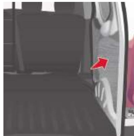
The interior parts of the sides are fitted with load protection trims.
