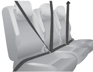
The three seats are fitted with three-point inertia reel seat belts.
