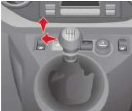
☞ In 6-speed configuration, lift the collar under the knob.
