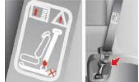
The two seats are fitted with three-point inertia reel seat belts.
