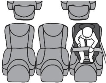
When a "rearward facing" child seat is installed **on a rear passenger seat**, move the vehicle's front seat forward and straighten the backrest so that the "rearward facing" child seat does not touch the vehicle's front seat.
