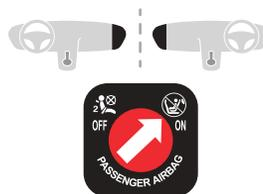
As soon as you remove the child seat, turn the passenger's front airbag switch to the **ON** position to reactivate the airbag and therefore ensure the safety of your passenger in the event of an impact.
