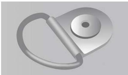
Use the stowing rings on the rear floor to attach your loads.
