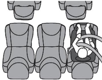
When a "forward facing" child seat is installed **on a rear passenger seat**, move the vehicle's front seat forward and the backrest to an upright position so that the legs of the child in the "forward facing" child seat do not touch the vehicle's front seat.
