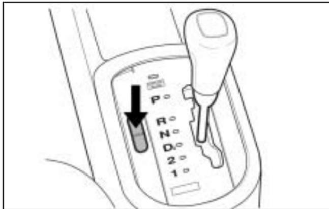
Press the HOLD button on the shift lever console to turn on hold mode. Press the button again to turn off hold mode, and return to normal automatic transaxle operation.
