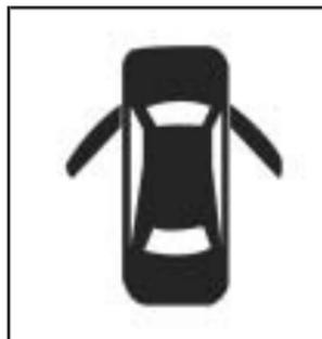
If one of the doors on your vehicle is not closed properly while the ignition is on, the door ajar light on the secondary information center will come on and stay on until the doors are closed.
