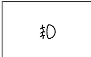
If your vehicle has this feature, the fog lamps light will come on when the fog lamps are in use.
