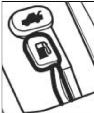
Open the trunk on your sedan from inside your vehicle by pulling up the release lever located to the left side of the driver's seat.
