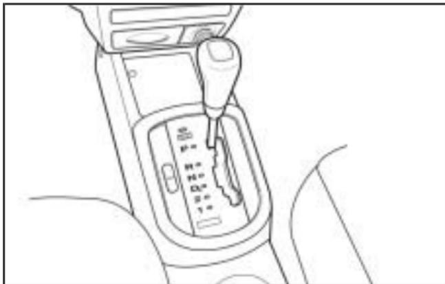
If your vehicle has an automatic transaxle, the shift lever is located on the console between the seats.
