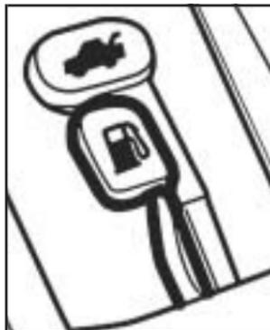
To open the fuel filler door, pull up on the fuel filler door release lever located on the floor to the left of the driver's seat.
