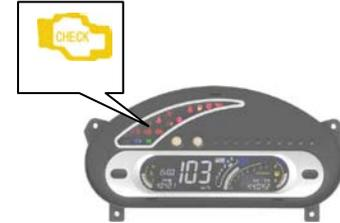
If the engine trouble indicator lamp lights in a short time and then extinguishes, it is a normal phenomenon and doesn't show that the system has any trouble..
