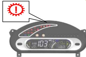
The indicator lamp lights after turning on the ignition switch, and, waiting for approx. 4 s, then extinguishes.
