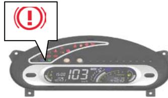
Before driving, completely release the hand brake. If the indicator lamp still lights after the completely releasing of hand brake, it shows that there is short of brake fluid. In this case, you shall:
