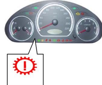
The light ON after the ignition switch turns on, and then off after about 4 s.
