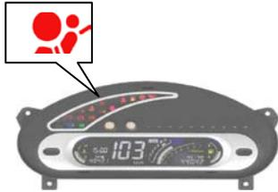
The indicator lamp lights after turning on the ignition switch, and, waiting for approx. 4 s, then extinguishes. It illustrates that the airbag system is normal.
