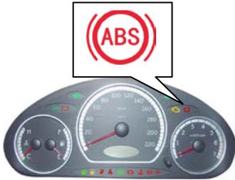
If ABS light is lit up during driving, there is a fault in ABS system. With ABS not working, if the brake system functions properly, go to the nearest CHERY AUTO authorized service station for inspection.
