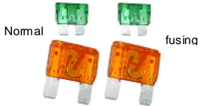
Dismount fuse box cover and take out blowing fuse when replacing fuse. View the face of the fuse to judge whether the fuse is damaged. Only the fuses with the same specification can be used with the specification on them.
