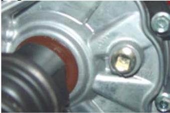
Use transmission fluid specified lubrication table. After installing filler lid, inspect if leakage or damage exists.
