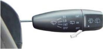
3 / 4 of its capacity. Turning control lever in the reverse direction of steering wheel may operate luggage compartment cover wiper and washer.
