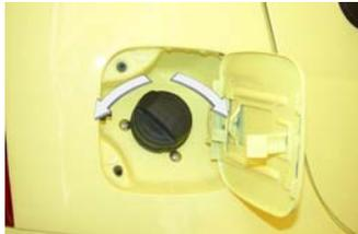
Do not use plumbic gasoline to the non-plumbic gas cars to avoid any damage to the engine and exhaust system. Gasoline will damage the painting. If the gasoline spatters on to the painting, wash it with cold water immediately. The gasoline in the fuel tank might be compressed. You can screw loose the fuel tank cap slowly. In cold weather, the fuel fill door may not be opened easily; you can open it by pushing or knocking it.
