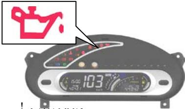
In case that the engine oil pressure alarm indicator lamp lights for a long time, it indicates that the engine has some one trouble, please immediately stop your vehicle to check whether there is short of engine oil when the vehicle is traveling, and, if necessary, refill the oil; if the
