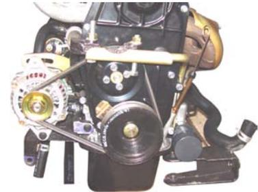
Install belt properly and ensure appropriate belt tension, otherwise generator, A/C and other system operating may be affected. If drive belt is worn, cracked or swelled, replace it. Check belt tension: apply appropriate thumb pressure at the middle and measure if belt displacement is about 10mm. If belt is too loose, adjust and repair at nearest CSSS.
