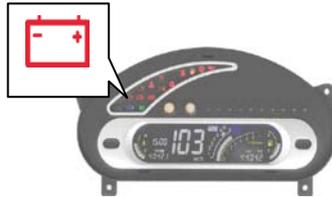
This alarm indicator lamp indicates that the battery is discharging.
