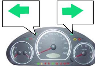
When turn signal light switch or hazard warning lamp switch is turned on, indicator light's blinking indicates the working condition of outer signal lamp or hazard warning lamp. A smaller frequency of blinking indicates a fault in turn signal indicator light bulb.
