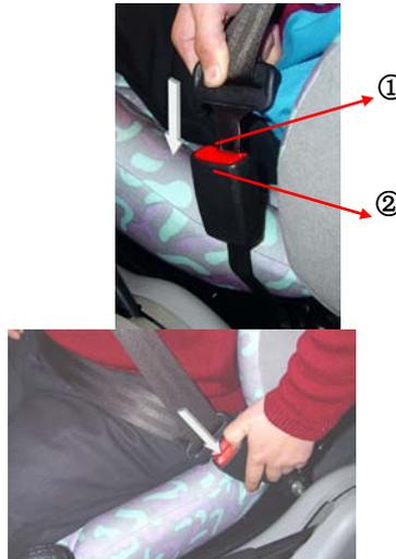
If you want to offload the seat belt, just press the red button on the ouch, the belt
