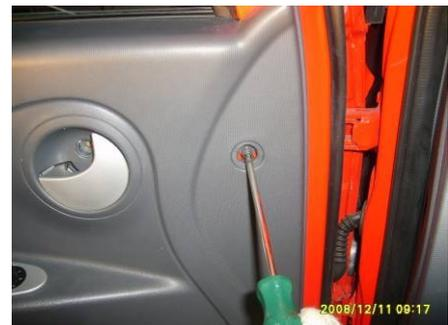
3.6. Pry out the protective cover of door inner armrest groove with slotted screwdriver.
