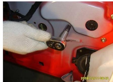
3.17. Pull off the window regulator connector and take out the window glass regulator assembly.
