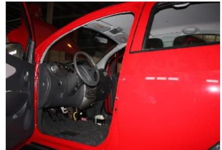
3.2. Pry out the front doorsill pressure plate with plastic screwdriver.
