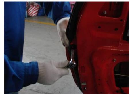
3.11. Connect the battery and lower the window glass at a proper position (let the glass fixing screws be exposed on the two installation holes as shown in figure) and remove the two screws that fix the glass with cross screwdriver, remove the glass carefully.
