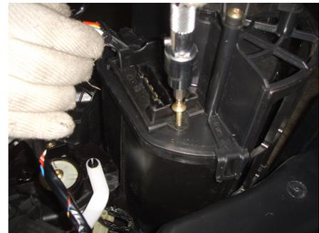
3.1.3. Pull out the speed regulation module.
