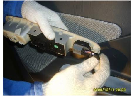
3.10. Pry out the door inner panel from edge with the plastic screwdriver.
