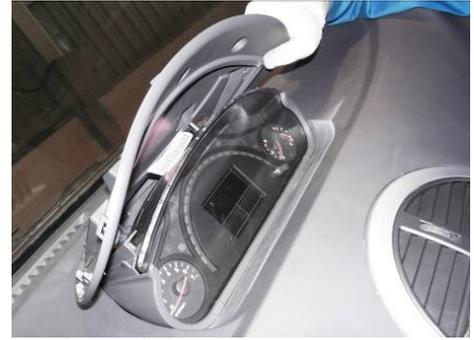
1.5. Remove the two fixing screws connecting the dashboard and instrument panel body with cross screwdriver.
