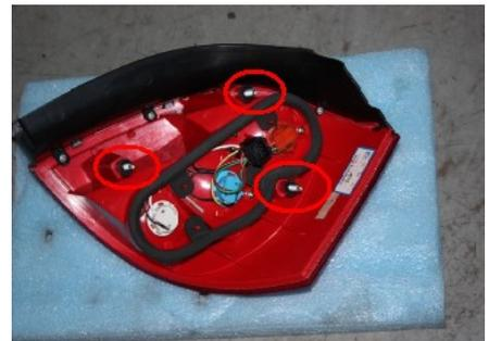
6.3. Pull off the tail lamp wiring harness connector and remove the tail lamp assembly.
