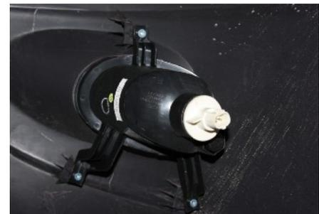
5.3. Rotate the rear fog lamp holder in anti-clockwise direction to remove the rear fog lamp bulb.
