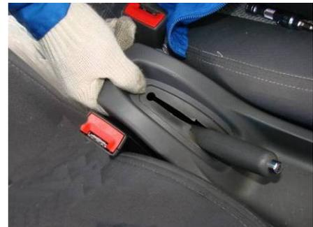
2.2. Use cross screwdriver to remove the front fixing screws of the central console assembly.
