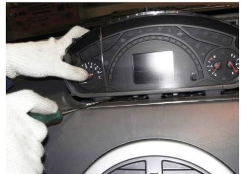
1.7. Pull off the harness connector on instrument panel body and remove it.
