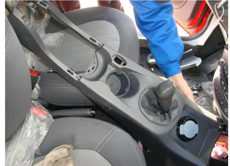
1.2. Remove the three fixing screws of instrument panel with cross screwdriver, remove the top cover of instrument panel.
