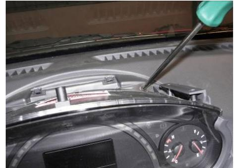
1.6. Pry out the dashboard body with slotted screwdriver.
