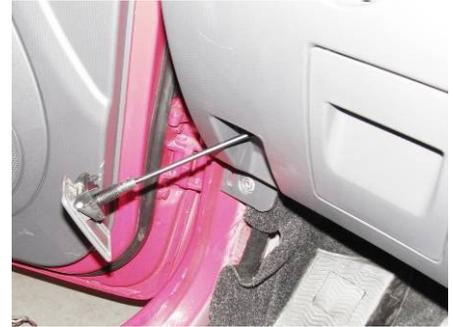
1.10. Pry out the central control panel shield with slotted screwdriver.
