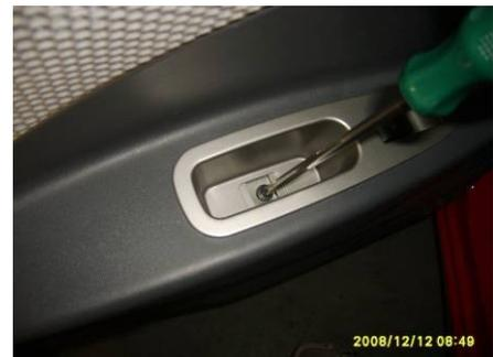
3.4. Pry out the window regulator switch with slotted screwdriver, pull off the connector of window regulator and remove it.
