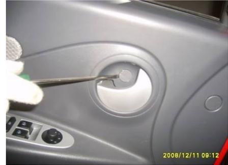
3.5. Remove the five fixing screws of door inner panel with cross screwdriver (two screws on panel front surface and three screws on panel side surface).
