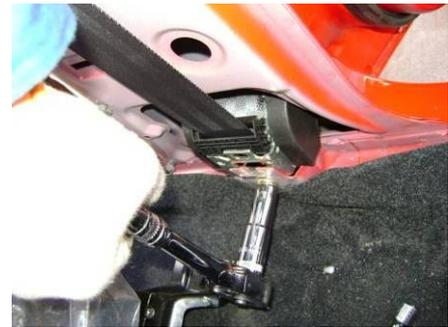
3.8. Remove the seat belt guide plate with cross screwdriver.
