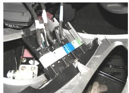
1.12. Remove the fixing screw of radio cassette player.
