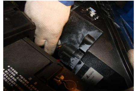
3.2. Remove the three headlamp fixing screws on the engine compartment cross beam and fender with 10# socket wrench and remove the headlamp.
