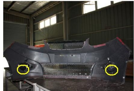
3.6. Remove the two fixing bolts of upper air intake grille with cross screwdriver to remove the air intake grille.
