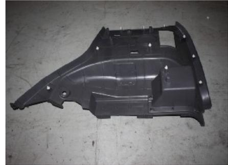
4.5. Pry out the pillar C upper panel with plastic screwdriver.
