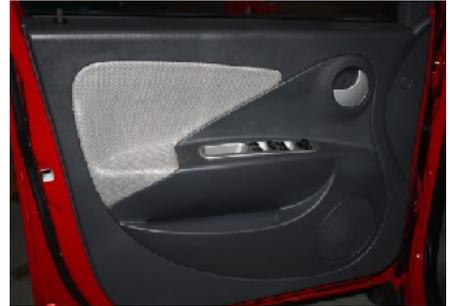
3.9. Pull out the exterior rear view mirror adjusting switch (only driver side) and window regulator control switch connector.
