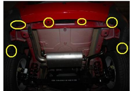
3.3. Use a 7# socket wrench to loosen the screws connecting the fender and the bumper.
