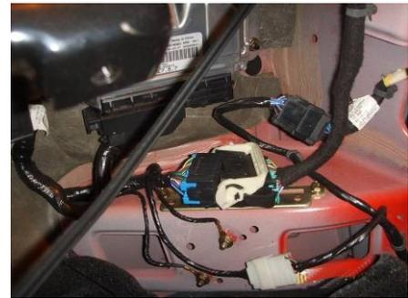
1.4. Remove the connector of instrument panel wiring harness and engine wiring harness.
