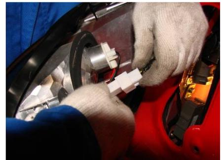
6.4. Rotate the bulb seat anti-clockwise by hand to remove the bulb.
