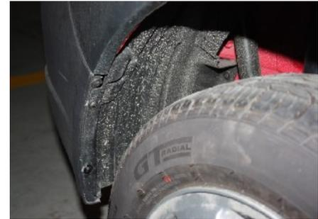
3.4. Apply the force vertical to fender surface to outwards to separate the bumper and fender clips and remove the bumper.
