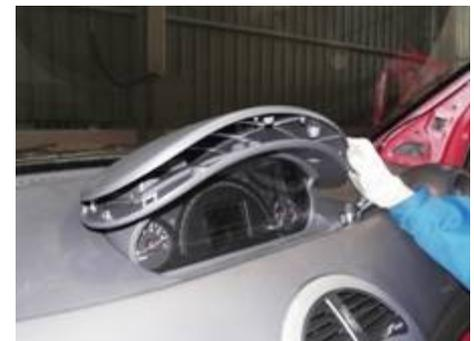
1.3. Loosen the five screws on lower cover of instrument panel with cross screwdriver.
