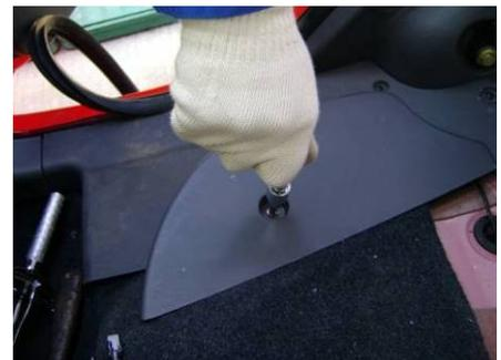
3.4. Remove the seat belt lower fixing bolt with 17# socket wrench.
