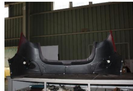
3.7. Push the reverse radar from inside of bumper towards outside to remove the reverse radar.
