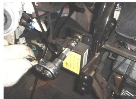
1.7. Remove the fixing bolt on two ends of instrument panel crossbeam with 10# socket wrench.
