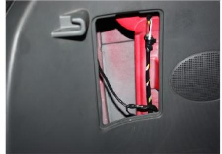
6.2. Remove the three nuts fixing tail lamp in luggage boot compartment with 10\$ socket wrench.
