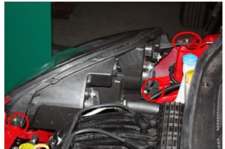
3.3. Open the headlamp high beam holder shield by hand.
