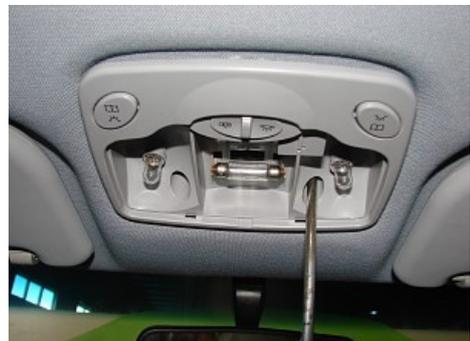
1.3. Disconnect the harness connector and remove the front ceiling lamp assembly.
