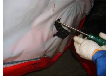
3.9. Remove the anti-water protective layer.
