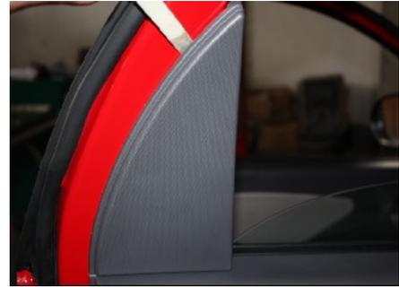
3.2. Pry out the protective cover of door inner armrest groove with slotted screwdriver, expose the fixing screw.
