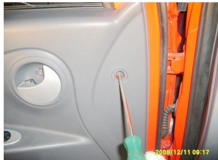
3.6. Pry out the door inner panel from edge with the plastic screwdriver.
