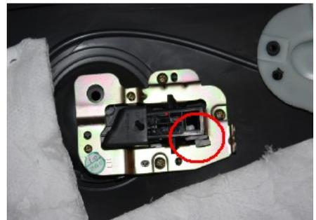
3.12. Remove the two screws of front door armrest fixing bracket with cross screwdriver.
