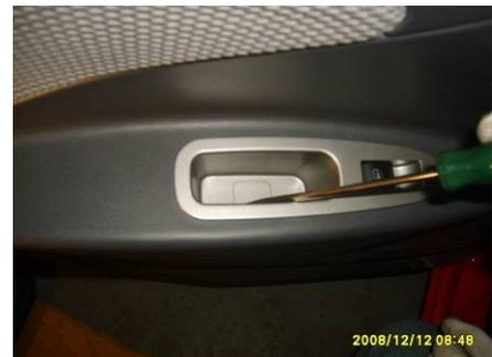
3.3. Remove the fixing screw of the door inner armrest with cross screwdriver.o
