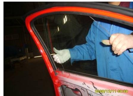
3.16. Remove the five screws that fix the window regulator with 10# socket wrench.
