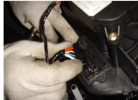
3.1.2. Use a cross screwdriver to remove the fixing screws on speed regulation module.
