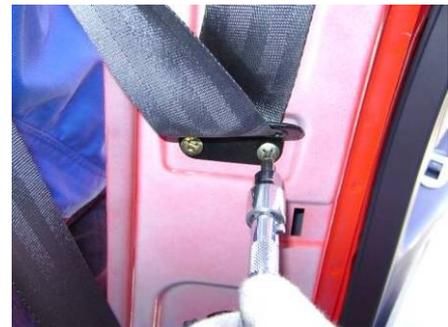
3.9. Remove the seat belt upper fixing point bolt with 17# socket wrench.
