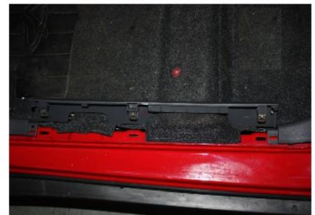
3.3. Remove the fixing bolts of rear doorsill with cross screwdriver and remove the rear doorsill pressure plate.
