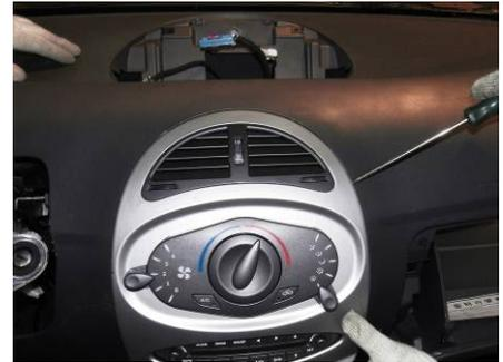
1.11. Pull off the A/C regulating switch harness and central control panel switch harness.
