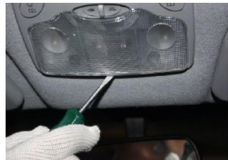
1.2. Remove the three fixing screws of the front ceiling lamp.
