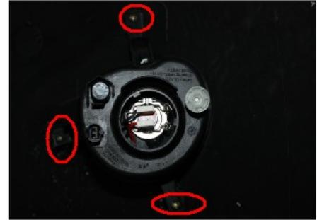
4.3. Press down the bulb fixing clip by hand and turn the clip over to take out the high/low beam bulb.
