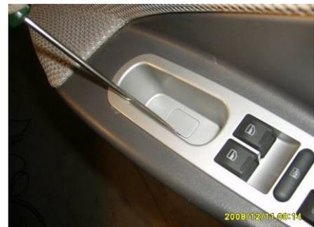
3.7. Remove the screw that fix the door inner armrest with cross screwdriver.
