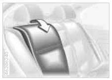
The rear backrest is divided into two sections (one-third and two-thirds of the width of the seat). For carrying longer objects, you can fold down either section of the backrest separately.
