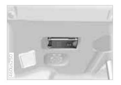
The OBD interface socket for onboard diagnostics is located on the driver's side, on the left-hand bottom of the instrument panel and under a cover panel. The cover has the letters "OBD" on it.
