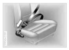
The safety belt tensioner makes sure that the belt tightens during a head-on collision to ensure that occupants remain firmly positioned in their seats. A gas-pressure system retracts the buckle assembly to tension the shoulder and lap belts within fractions of a second. This reduces the tendency to slide under the lap belt.
