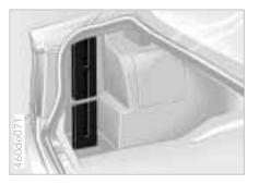
The warning triangle is stored in a recess on the left-hand side of the luggage compartment where it is quickly available.
