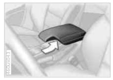
To open the storage compartment in the front center armrest: press the button (arrow) and lift upward.
