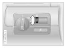
Turn the rotary dial to adjust the illumination intensity.
