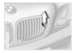
**To open** Pull the release handle and open the hood.
