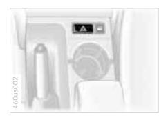
The button flashes on and off when the hazard warning flashers are on.
