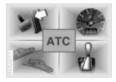
In order to include driving conditions in its calculations, ATC registers curves and both uphill and downhill gradients. For example, if you maintain speed through a curve, the transmission does not shift up. On uphill gradients, it shifts up only when the engine speed increases in order to make more efficient use of power reserves. On downhill gradients, ATC shifts down when the speed of the vehicle increases and the driver must apply the brakes.
