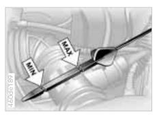
The oil volume between the two marks on the dipstick corresponds to approx. 1.1 US quarts (1 liter). Do not fill beyond the upper mark on the dipstick. Excess oil will damage the engine.
