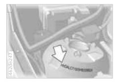
In the engine compartment, on the right-hand strut dome (arrow).
