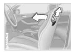
Pull up on the lever and flip the backrest toward the front.
