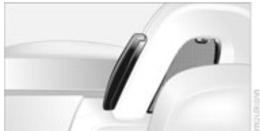
The illustration shows the wind deflector guide and the wind deflector panel on the passenger side.
