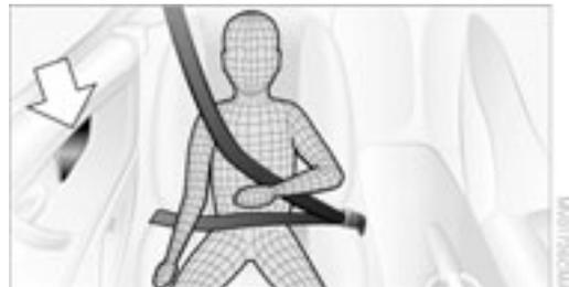
This is the correct way a larger child no longer using a child-restraint system should sit wearing the safety belt, when the airbag system is activated.
