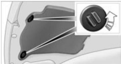
1. Open the caps with a suitable object – coin or screwdriver
