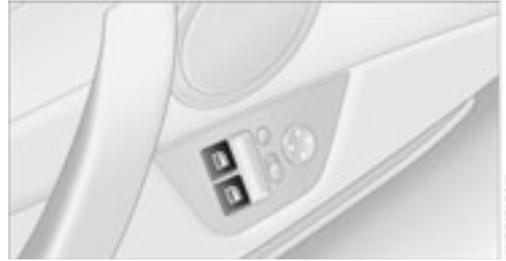
The illustration shows the power window switches in the trim of the passenger door.
