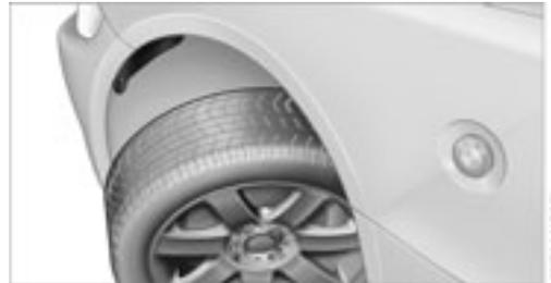
To gain access to the headlamp covers, turn the front wheels in the required direction.
