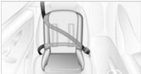
Commercially available child seats complying with the legal standard are designed to be secured with a seat belt or with the seat belt portion of a combination lap/shoulder belt.
