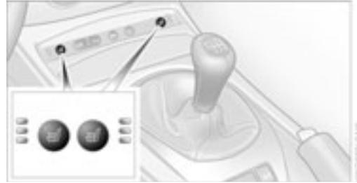
The seat cushion and backrest can be heated with the ignition key in position **2**. You can call up different heating modes by repeatedly pressing the buttons.
