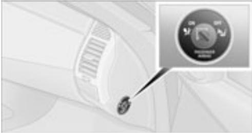
Deactivation of the passenger airbags system deactivates the passenger front, knee and side airbag. The airbags on the driver side remain active.
