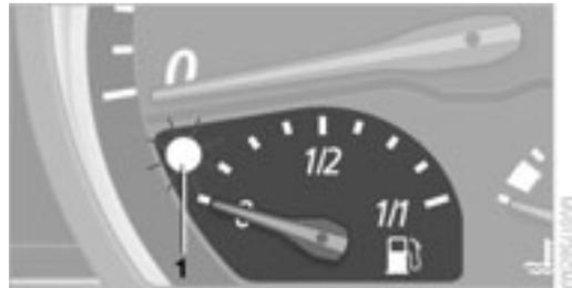
Once indicator lamp **1** stays on continuously, there are still approx. 2 gallons / 8 liters of fuel in the fuel tank.
