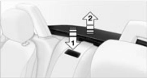
4. Press button; see arrow 1. The convertible top is released and moves up slightly; see arrow 2
