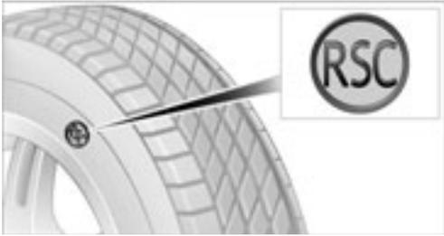
Run Flat tires are labeled on the sidewall with a circular symbol containing the letters RSC.
