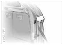
From the cargo area: the switches are located on both sides of the cargo area.
