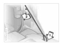
6 Insert support rod in tailgate lock and press down until it engages (arrow 1); then lock hook of rod in striker (arrow 2).
