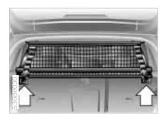
6 Attach the hooks on the bottom of the partition net into the eyes on both sides.
