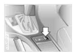
You can operate the central locking system with this button (arrow) when the driver's door is closed. The doors and liftgate are unlocked or locked only. However, the antitheft alarm system is not activated. Also, the fuel filler door remains unlocked to allow refueling.
