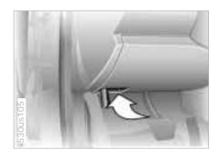
The Onboard Diagnostic (OBD) interface socket is located on the left of the driver's side at the bottom of the instrument panel and under a cover. The cover has the letters "OBD" on it.
