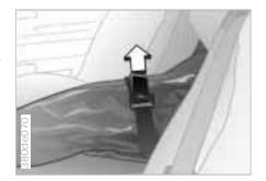
Secure the bag's contents by tightening down the retaining strap at the buckle.
