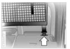
7 When the seatbacks are folded over, you can open the Velcro strips, completely unroll the partition net, insert it in the front brackets on the roof and attach the three hooks into the eyes. The illustration shows securing at the bottom right as an example.
