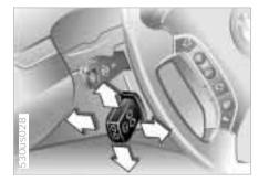
The steering wheel can be moved in any of four directions. Adjust the wheel by moving the control lever in the desired direction.
