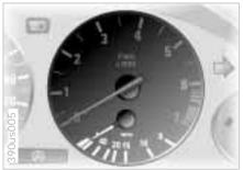
Indicates the current fuel consumption in mpg (in liters/100 km on Canadian vehicles). This allows you to see whether your current driving style is conducive to fuel economy with minimum exhaust emissions.
