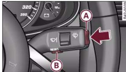
Fig. 14 Windscreen wiper lever: Controls for menu display
