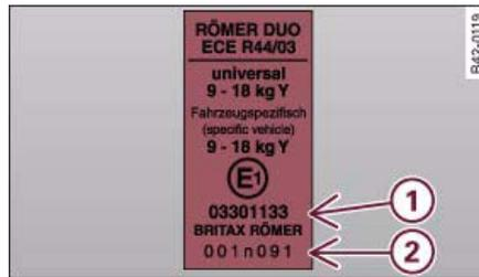
Fig. 107 Example of an approval number on a child safety seat
