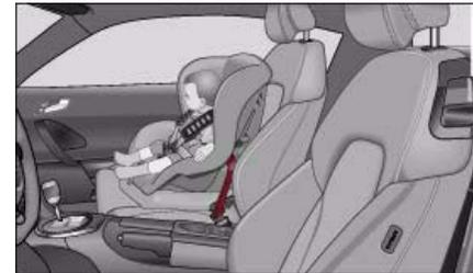
Fig. 104 A category 1 forward-facing child seat fitted on the passenger seat
