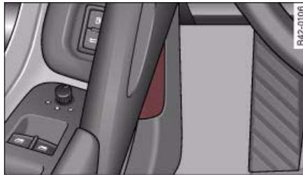
Fig. 115 Detail of footwell on driver's side: Release lever
