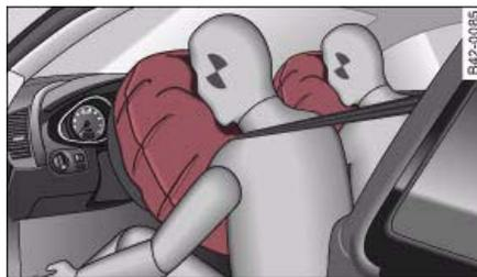
**Fig. 97** Front airbags in inflated condition
