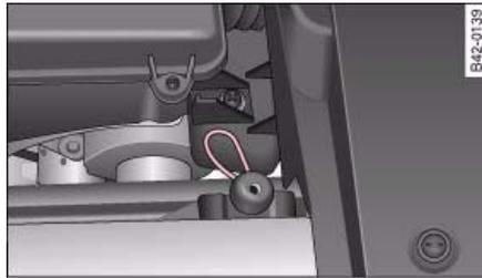
**Fig. 114 Engine compartment: Manual release**
