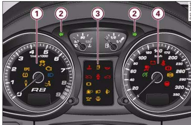
Fig. 6 Instrument cluster with warning and indicator lamps
