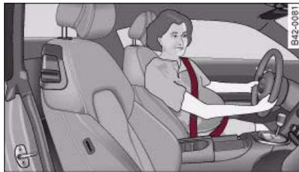
Fig. 93 Positioning seat belts during pregnancy
