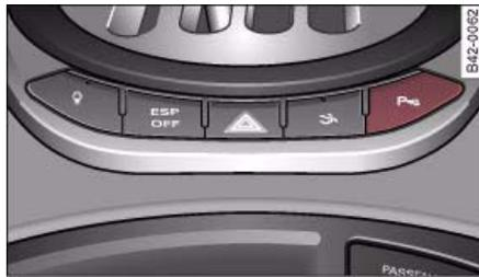
Fig. 74 Parking aid switch in centre console
