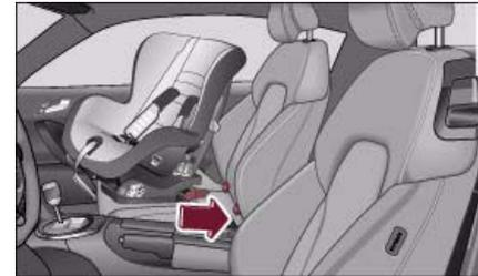
Fig. 109 The ISOFIX child safety seat can be secured after fitting the protective sleeves.
