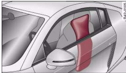
Fig. 100 Side airbag in inflated condition
