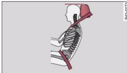
Fig. 85 Correctly adjusted head restraint (seen from the side)
