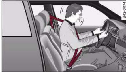
**Fig. 86 Driver with properly positioned seat belt – good protection if the brakes are applied suddenly**
