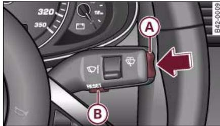
Fig. 12 Windscreen wiper lever: Controls for menu display
