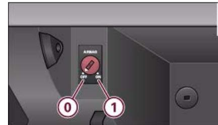
**Fig. 101** Key-operated switch for deactivating front passenger's airbag ▶
