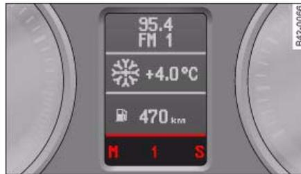
Fig. 78 Display: Engaged gears
