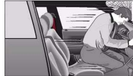
**Fig. 89** A driver not wearing a seat belt can be thrown forwards
