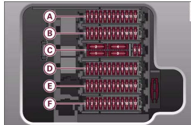
Fig. 134 Fuse layout in passenger's footwell, rows A to F
