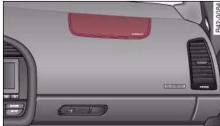
**Fig. 96** Front passenger's airbag in dashboard
