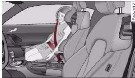
Fig. 105 A category 2/3 forward-facing child seat (with backrest) fitted on the passenger seat
