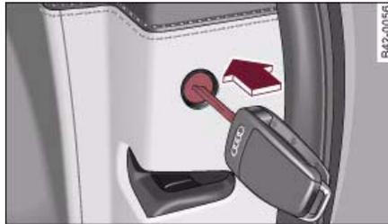
Fig. 39 Locking the door manually
