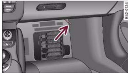
Fig. 42 Detail: Manual release
