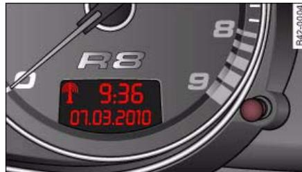
Fig. 3 Detail of the instrument cluster: Display with signal reception symbol, time and date
