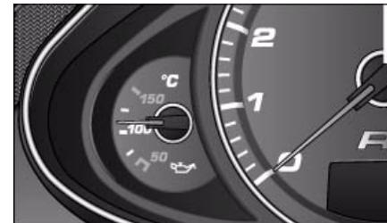
Fig. 117 Instrument cluster: Engine oil temperature display
