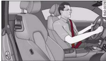
Fig. 90 Positioning of head restraints and seat belts
