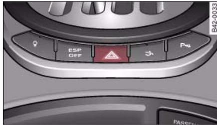
Fig. 50 Centre console: Switch for hazard warning lights
