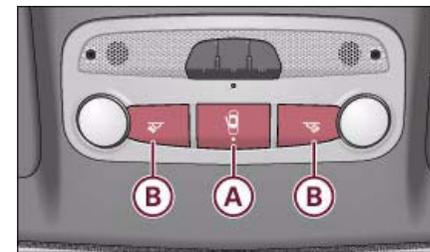
Fig. 52 Detail of headliner: Interior lights
