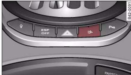
Fig. 111 Switch for rear spoiler
