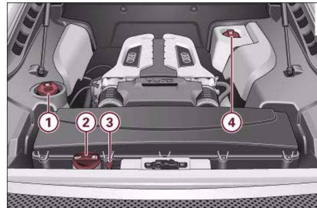
Fig. 116 Typical locations of fluid containers, engine oil dipstick and engine oil filler cap
