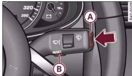
Fig. 11 Windscreen wiper lever: On-board computer controls
