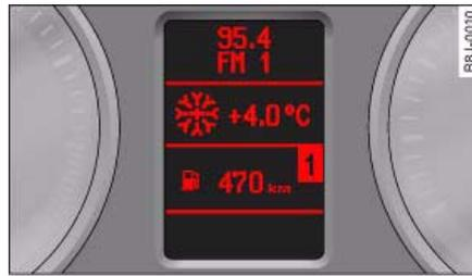
Fig. 7 Display: Standard display
