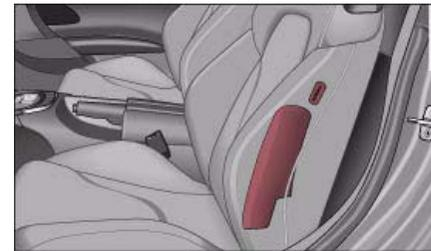
**Fig. 99** Location of side airbag in driver's seat
