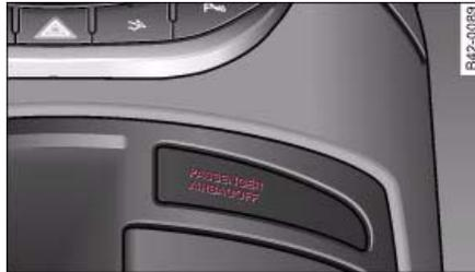
Fig. 102 Lamp indicates that front passenger's airbag has been deactivated via key-operated switch
