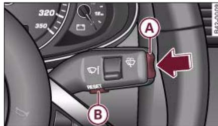
Fig. 8 Windscreen wiper lever: Reset button and rocker switch
