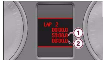
Fig. 24 Display: Lap 1 recorded; lap 2 started
