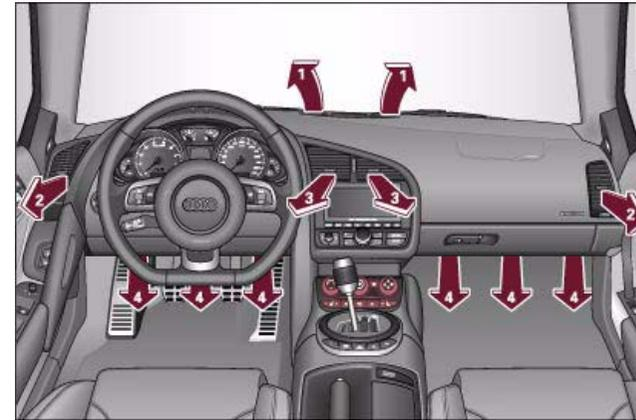
Fig. 70 Dashboard: Location of air outlets
