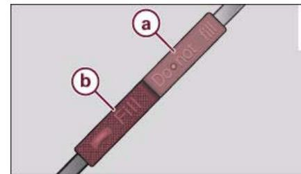
Fig. 118 Markings on oil dipstick
