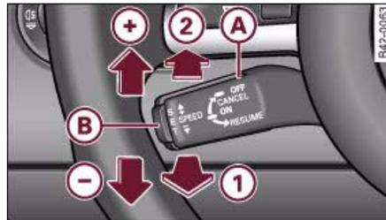
Fig. 75 Controls for the cruise control system
