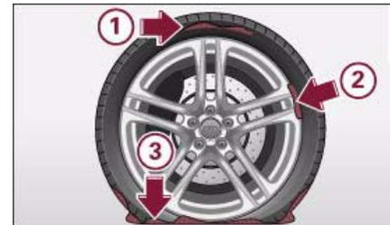
Fig. 124 The Tyre Mobility System is NOT suitable for repairing this type of damage to tyres.
