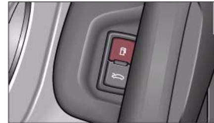
Fig. 112 Tank flap release button in the driver's door trim
