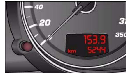
**Fig. 5** Detail of the instrument cluster: Mileage recorder with reset button
