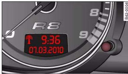
Fig. 29 Detail of the instrument cluster: Adjuster/test button
