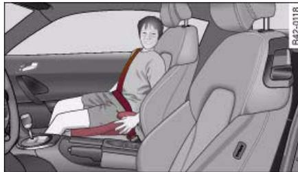
Fig. 106 A category 3 forward-facing child seat (without backrest) fitted on the passenger seat
