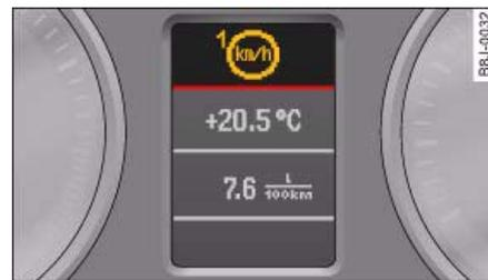
Fig. 28 Display: Speed warning
