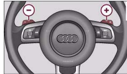
Fig. 79 Sports steering wheel with Paddle levers
