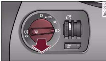
Fig. 46 Detail of the dashboard: Light switch
