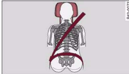
Fig. 84 Correctly adjusted head restraint (seen from the front)
