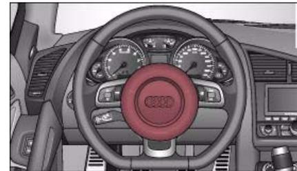
**Fig. 95** Driver's airbag in steering wheel ▶
