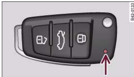
Fig. 33 Remote control key: Indicator lamp
