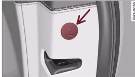
Fig. 38 Manual locking device on the passenger's door pillar
