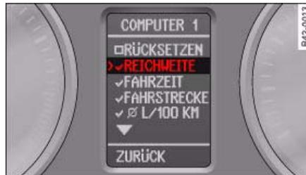
Fig. 19 Display: "Computer 1" menu, "Fuel range" (Reichweite) selected
