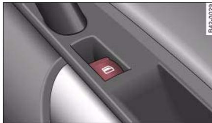
Fig. 45 Switch on front passenger's door
