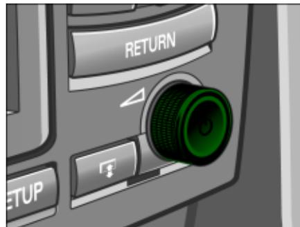
Fig. 15 Navigation System ON/OFF knob
