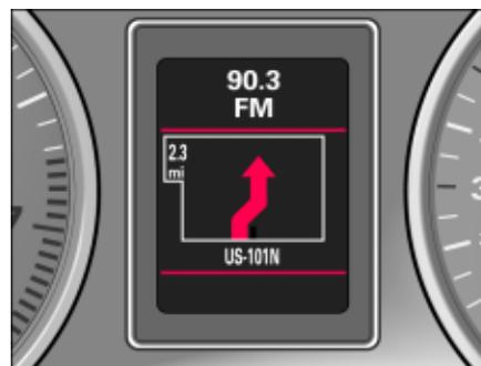
Fig. 114 Navigation: Example of display in the instrument cluster
