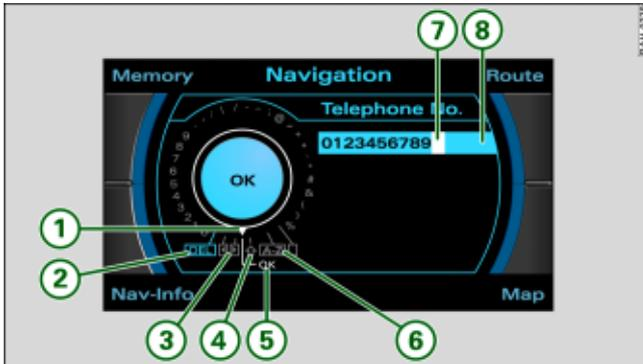
Fig. 25 Display: Number entry in the speller, e.g. entering special destination using telephone number
