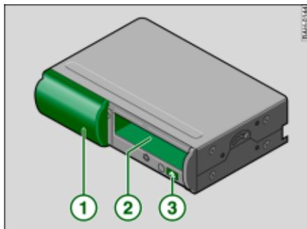
Fig. 44 CD changer with magazine
