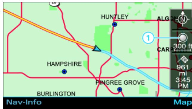
Fig. 154 Navigation: Adjusting zoom with inactive side menu
