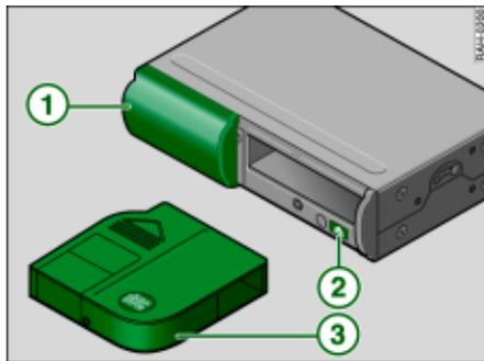
Fig. 46 CD changer with magazine
