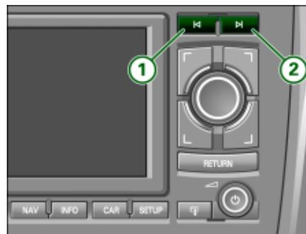
**Fig. 13** Navigation System Forward/reverse button
