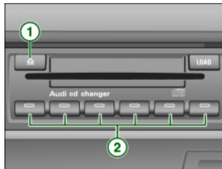
Fig. 43 Audi cd changer: Ejecting CDs
