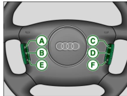
Fig. 16 Multi-function steering wheel with audio operation
