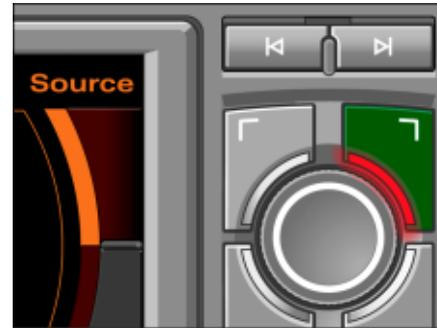
Fig. 11 Navigation System: Assignment of control buttons and button symbols to the screen corners. ►
