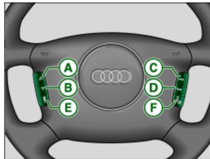
Fig. 17 Multi-function steering wheel with audio operation (version A)
