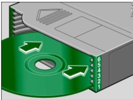
Fig. 48 Inserting the CD in the magazine
