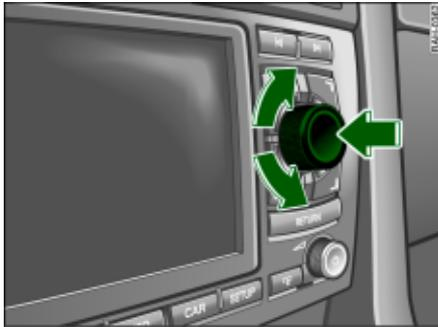
Fig. 9 Navigation System: Control knob
