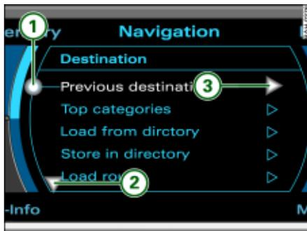
Fig. 23 Section of display: Orientation symbols
