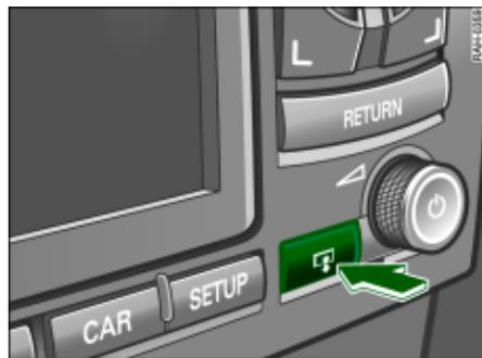
**Fig. 4 Navigation System: Button for opening and closing the display**
