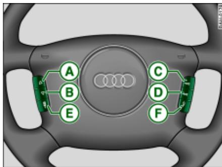
Fig. 19 Multi-function steering wheel with audio operation - version C
