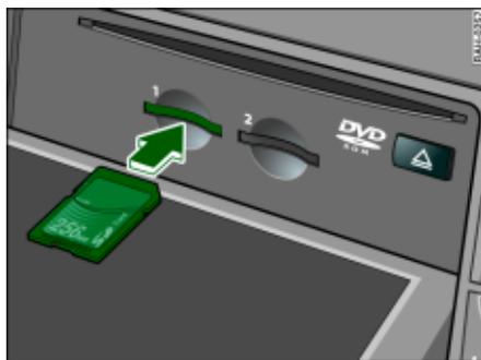
Fig. 39 Display open: Inserting a memory card.
