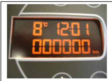
Displaying the outside temperature is possible only on models with two LCD. It appears in the right-hand LCD.
