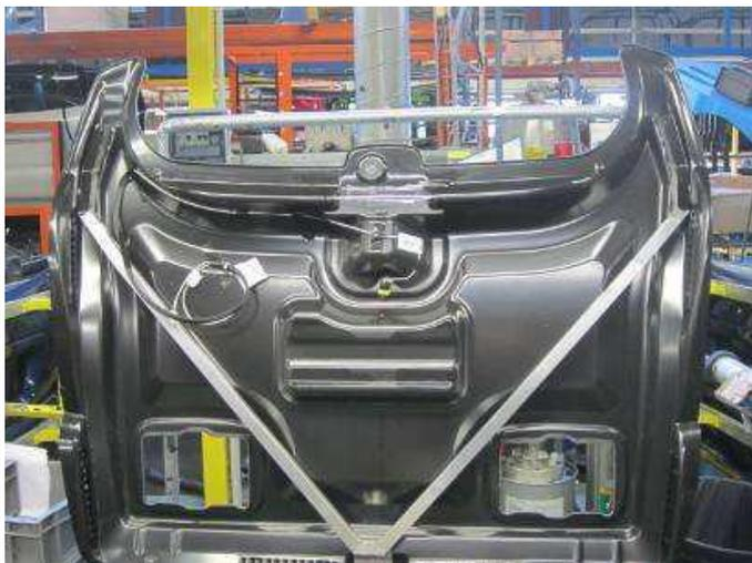
Rivet the tailgate hook with the frame
