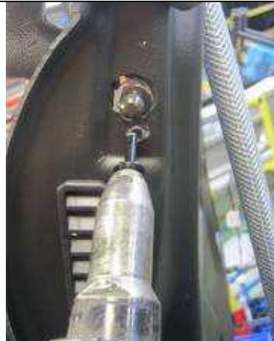
Apply glue on the frame for gluing the tailgate glass
