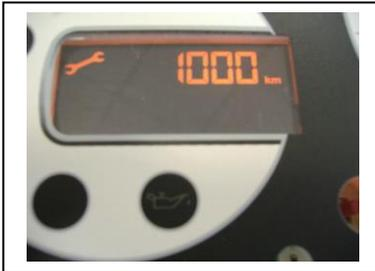
If the mileage exceeds 200 km before maintenance, the LCD displays the mileage remaining + the « key » symbol for 5 seconds. If the mileage is less than 200 km before maintenance, the LCD displays the mileage remaining flashing + the « key » symbol for 5 seconds.
