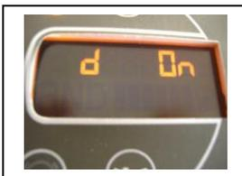
This message means the diesel preheating function is activated.
