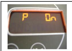
This message means the dome light control function is activated.
