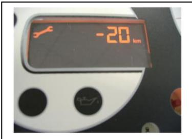
If the total mileage before maintenance has been exceeded, the LCD displays the mileage in negative flashing + the « key » symbol for 5 seconds.
