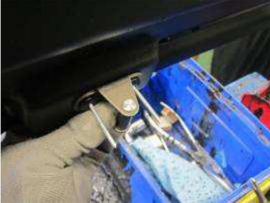
Step 4: Assemble joints head 7K102A
