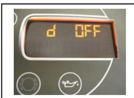
This message means the diesel preheating function is inhibited.
