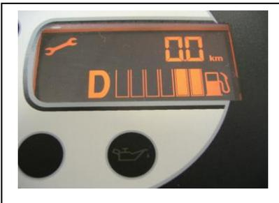
If the mileage for maintenance is exceeded, the LCD displays the « key » symbol on the left-hand display, permanently.
