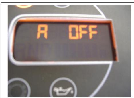
This message means the automatic warning lights function is inhibited.
