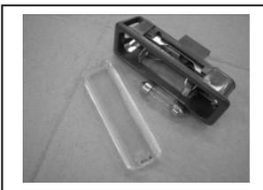
Unclip the interior lighting from the dome light to change the lamp.
