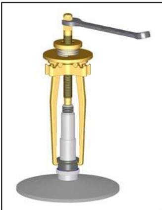
Removing the tightening ring (1b)
