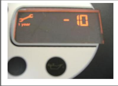
If the total time (days) before maintenance has been exceeded, the LCD displays the mileage in negative flashing + the « key » symbol and « 1 year » for 5 seconds.
