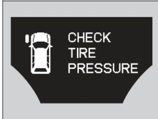
**CHECK TIRE PRESSURE** is displayed when a tire has significantly low pressure. The specific tire is displayed on the screen.
