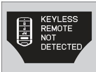
Warning buzzers may sound from inside or/ and outside the vehicle to remind you that the keyless access remote is out of the vehicle. If the buzzer continues even after the remote is put back inside, place it within its operational range.
