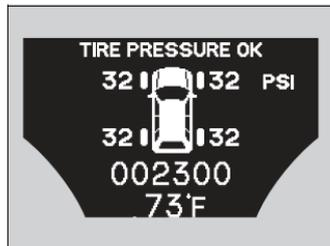
To select the tire pressure monitor, set the power mode to ON and press the
