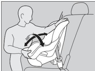
6. Make sure the child restraint system is firmly secured by rocking it forward and back and side to side; little movement should be felt.
