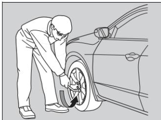
**9.** Loosen each wheel nut about one turn using the wheel nut wrench.
