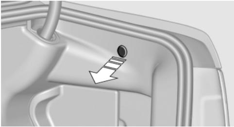
Pull the green knob with the fuel pump symbol. This releases the fuel filler flap.
