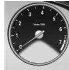
Always avoid engine speeds in the red warning field. In this range, the fuel supply is interrupted to protect the engine.
