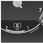
Displays the state of the high-voltage battery's charge on a scale from 0 to 1 when drive readiness is active. If the scale indicates 1, the high-voltage battery is fully charged.
