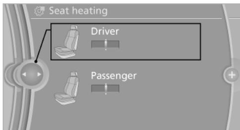
4. Turn the controller to set the temperature distribution.
