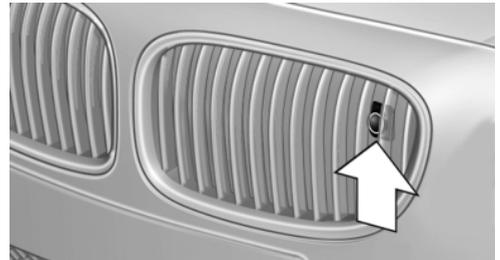
Rain, dirt, snow, or ice can impair camera operation.
