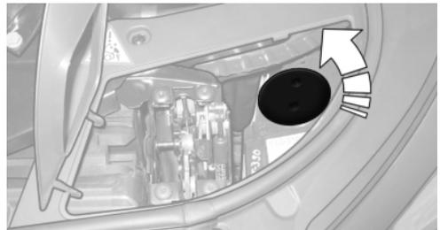
3. Unscrew the bulb holder counterclockwise.
