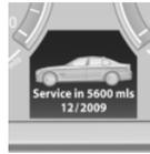
The driving distance or the time to the next service is displayed briefly after the ignition is switched on.
