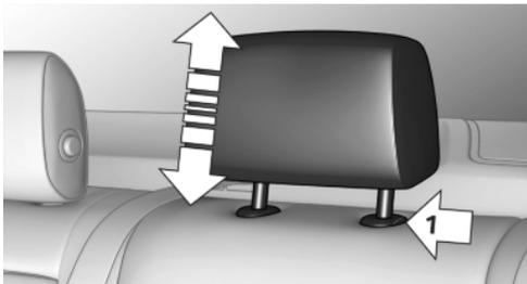
1. Pull the head restraint upward as far as possible.
