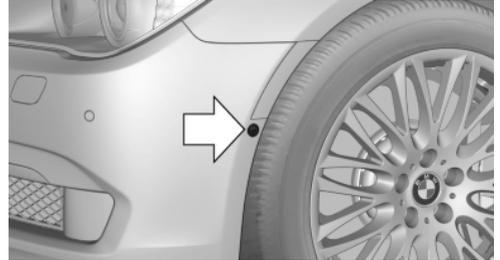
The two camera lenses are located on the sides of the bumper.
