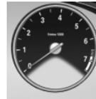
Always avoid engine speeds in the red warning field. In this range, the fuel supply is interrupted to protect the engine.
