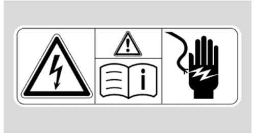
Indicate, on certain parts or assemblies, that incorrect use of high-voltage equipment or high-voltage components results in the risk of fatal injury from electric shock.
