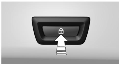
Press the button on the inside of the trunk lid. When the driver's door is closed, the vehicle is completely locked.
