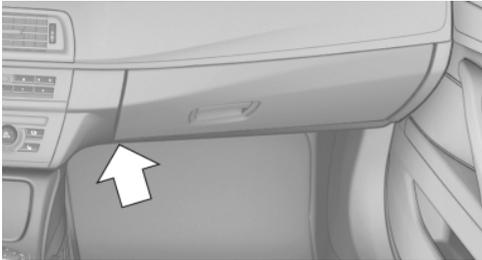
Socket is located below the glove compartment.
