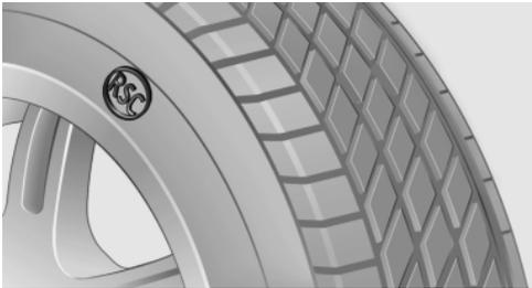
RSC label on the tire sidewall.
