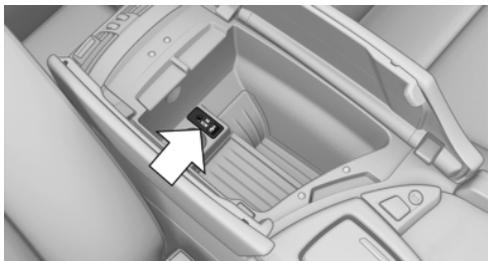
This can be used to connect an external audio device, such as an MP3 player.
