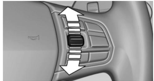
On the right side of the steering wheel, turn the thumbwheel to activate the corresponding list. Using the thumbwheel, select the desired setting and confirm it by pressing the thumbwheel.
