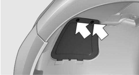
Remove the screws and fold down the cap.
