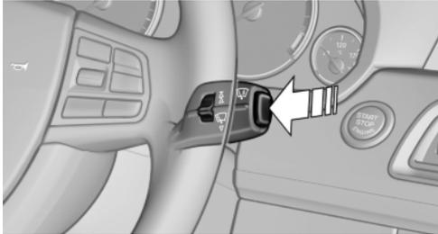
Press the button on the wiper lever.
