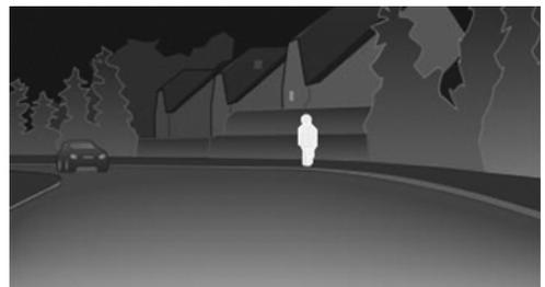
The pedestrian detection and warning system only operates in darkness and only when a heat image is displayed.
