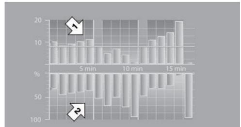
The gray bars show the fuel consumption by the combustion engine, arrow 1. The blue bars show
