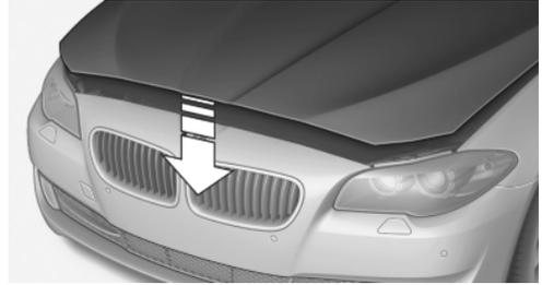
Let the hood drop from a height of approx. 16 in/40 cm and push down on it to lock it fully. The hood must audibly engage on both sides.
