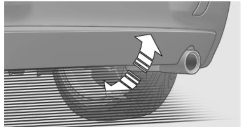
The trunk lid opens, regardless of whether it was previously locked or unlocked.
