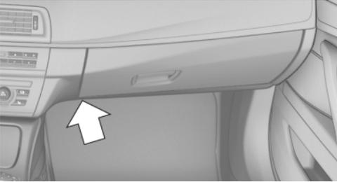
Socket is located below the glove compartment.
