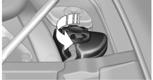
3. The coolant level is correct if it lies between the minimum and maximum marks in the filler neck.
