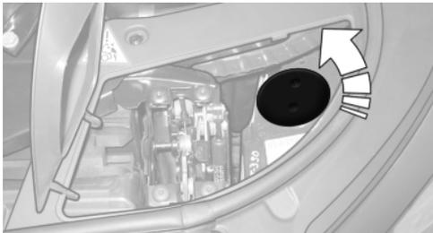
3. Unscrew the bulb holder counterclockwise.
