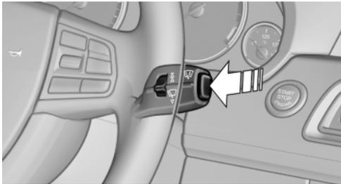
Press the button on the wiper lever.
