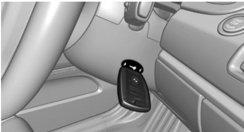
Automatic transmission: if a corresponding Check Control message appears, hold the remote control, as shown, against the marked area on the steering column and press the Start/Stop
