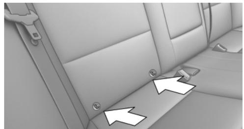
Mounts for the lower LATCH anchors are located in the gap between the seat and backrest.
