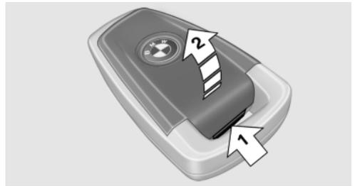
1. Use a suitable object to unclip the battery compartment, arrow 1.
