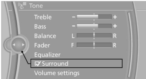
When surround is activated, multi-channel playback is simulated when a stereo audio track is played.
