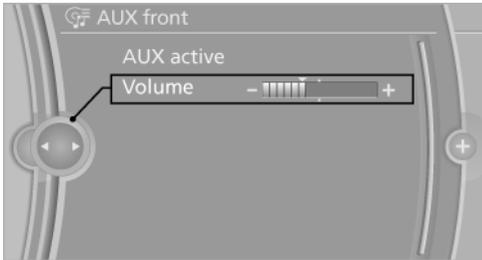
5. Turn the controller until the desired volume is set and press the controller.
