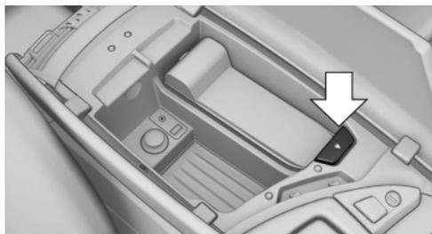
2. Insert the snap-in adapter in the direction of the arrow, arrow 1, and press down, arrow 2, until it engages.
