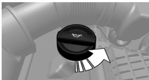
Only replenish the maximum oil amount of 1 US quart/liter if the message is displayed in the instrument cluster or the oil level has dropped to just at the lower mark of the dipstick.
