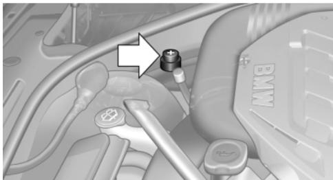
The so-called starting aid terminal in the engine compartment acts as the battery's positive terminal.
