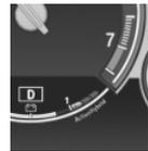
The energy recovered is displayed in the tachometer as an arrow with the symbol +. The high-voltage battery is charging.
