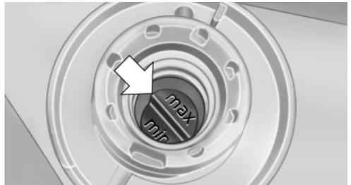
4. If the coolant is low, slowly add coolant up to the specified level; do not overfill.
