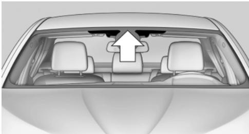
The marked area is not covered with heat reflective coating.
