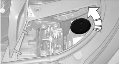
3. Unscrew the bulb holder counterclockwise.
