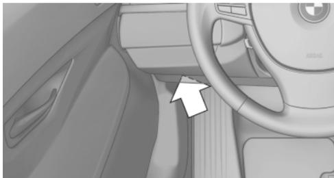
There is an OBD socket on the driver's side for checking the primary components in the vehicle emissions.
