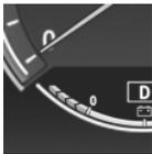
When driving with electric power, the power output of the electric motor is indicated by arrows.
