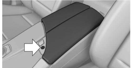
The storage compartment in the armrest can be locked with an integrated key to separately secure the trunk lid, refer to page 41, for example.
