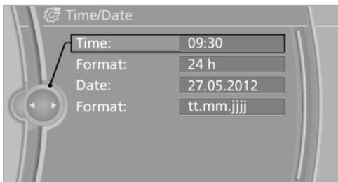
6. Turn the controller to set the hours and press the controller.
