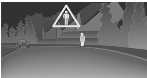
If the system detects a person in a defined area in front of the vehicle and if there is the danger of collision with this person, a warning symbol appears on the Control Display and in the Head-up Display.
