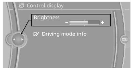
4. Turn the controller until the desired brightness is set.
