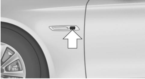
The ultrasound sensors used to measure parking spaces are located in the side turn signals.
