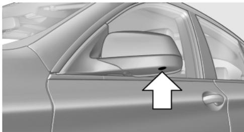
The lenses of the Top View cameras are located at the bottom of the exterior mirror housings. The image quality may be impaired by dirt. Clean the lens, refer to page 292.
