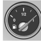
The vehicle inclination may cause the display to vary.
