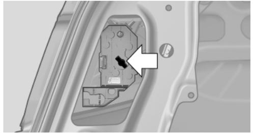
The illustration shows the position of the bulb in the installed bulb holder.
