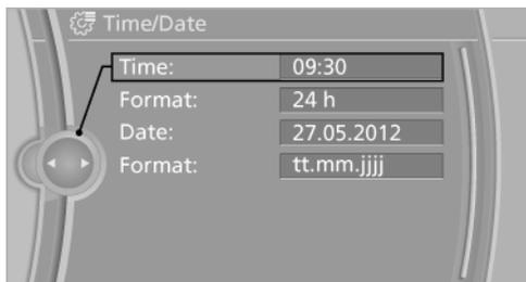
4. Turn the controller until the desired hours are displayed.
