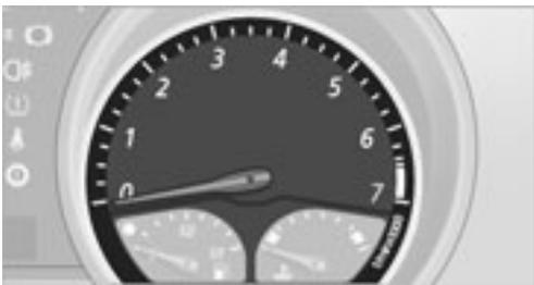
Never allow the engine to operate with the needle in the red overspeed sector of the gauge.
