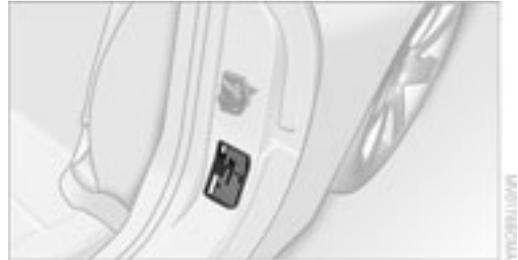
The specified inflation pressures are provided on a sticker attached to the B-pillar and are visible when the driver's door is open.
