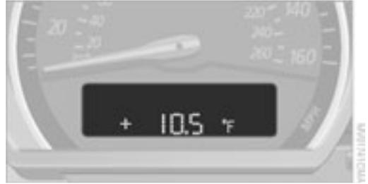
If the vehicle is not equipped with a computer, the display in the instrument cluster always shows the outside temperature.
