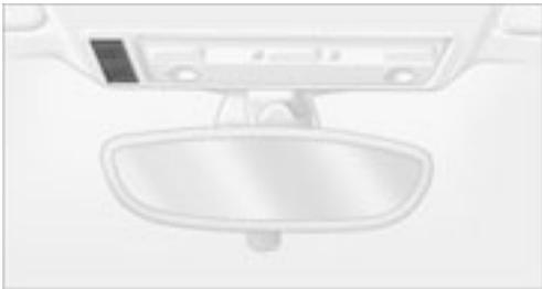
In vehicles that are wired for a telephone\*, the cover of the hands-free microphone is located in the headliner close to the interior lamps.
