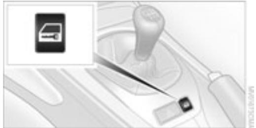
You can use this button to control the central locking system whenever the doors are closed. The doors and luggage compartment lid are unlocked or locked only. The anti-theft system is not activated.
