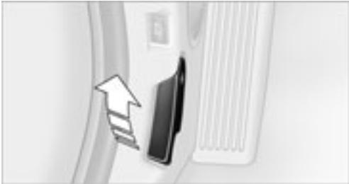
Pull the lever located under the left-hand side of the instrument panel.
