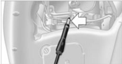
3. Use the screwdriver to pull out the entire bulb holder
