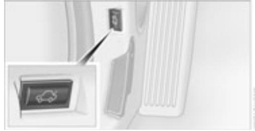
If the luggage compartment lid has not been locked separately, you can open it with this button in the footwell on the driver's side when the vehicle is stationary.
