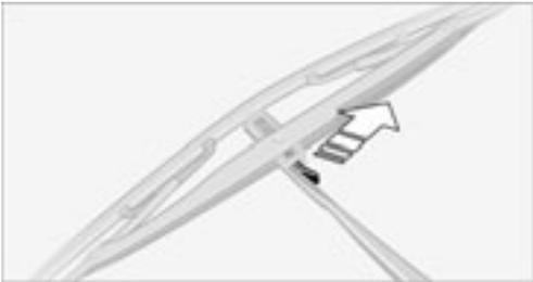
1. Fold the wiper arm completely out from the windshield
