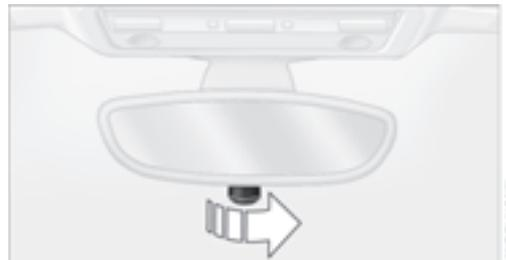
To reduce the glare from vehicles behind you when driving at night, turn the rotary knob.
