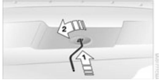
7. Insert the Allen wrench into the hex slot
