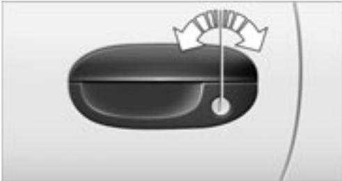
One turn of the key in the driver's door lock to unlock the driver's door only and the fuel gas door.
