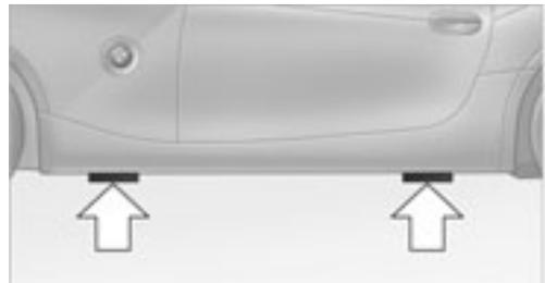
The jacking points are located at the positions indicated in the illustration.
