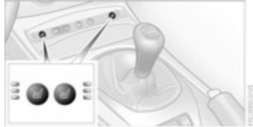
The seat cushion and backrest can be heated with the ignition key in position **2**. You can call up different heating modes by repeatedly pressing the buttons.
