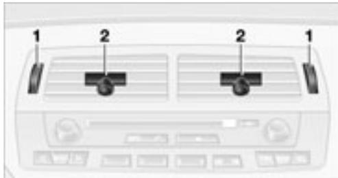
You can adjust the blower controls for the upper body area to obtain the optimum airflow rates and directions for your personal requirements:
