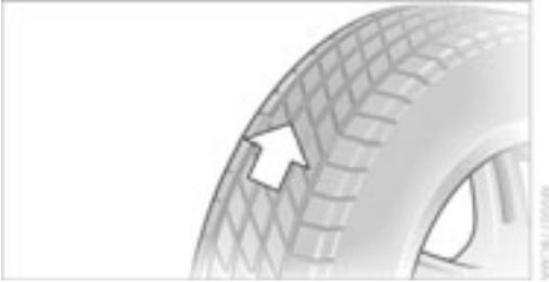
Inspect your tires frequently for tread wear, signs of damage and for foreign objects lodged in the tread. Check the tread depth.
