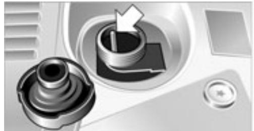
Correct coolant level when the engine is cold – at approx. 68 °F / 20 °C:
