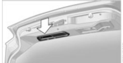
The handle recess in the interior trim panel of the luggage compartment lid makes it easier to pull the lid down.
