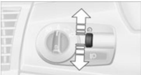
Turn the rotary dial to adjust the illumination intensity.
