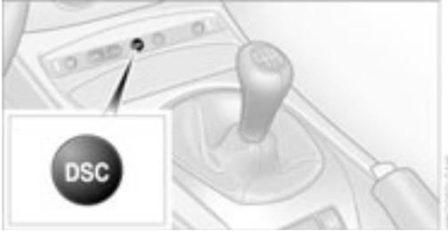
Press the DSC button briefly. The DTC indicator lamp comes on and stays on.
