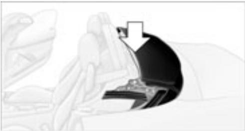
5. Grab the convertible top at its frame and pull it up to the windshield frame
