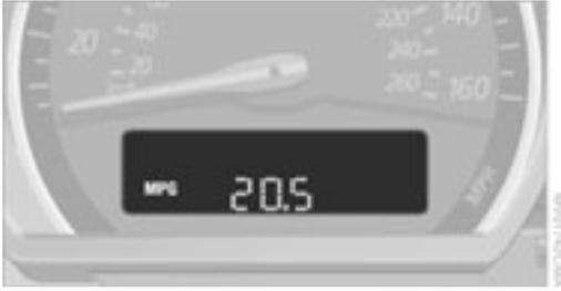
If you continue to press the button on the turn signal lever, the average fuel consumption last displayed is recalculated from that point in time.
