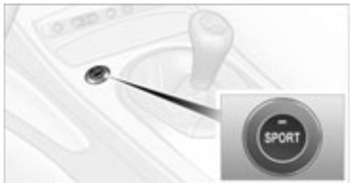
The Drivelogic feature lets you select between the standard and sport program. The sport program is recommended for performance-oriented driving.
