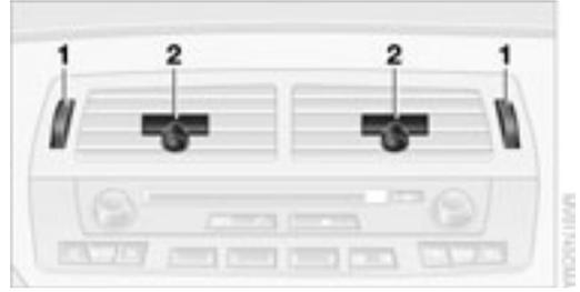
You can adjust the blower controls for the upper body area to obtain the optimum air-flow rates and directions for your personal requirements:
