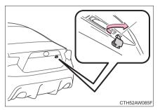
Turn the mechanical key clockwise to open.
