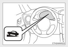
When the system is enabled, the hill start assist ON indicator will be illuminated.
