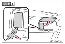
Open the cover and remove the lens.
