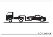
Never tow a vehicle from the front with the rear wheels on the ground. Use a towing dolly under the rear wheels.
