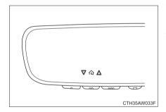
Within five seconds after programming a new HomeLink button, both of HomeLink's garage door status indicators will flash rapidly green indicating that the garage door two-way communication has been enabled. If your garage door status indicators flashed, two-way communication programming is complete.
