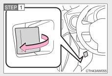
Pull the engine hood release lever.
