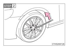
Slightly loosen the wheel nuts (one turn).
