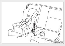
Seatbelts equipped with a child restraint locking mechanism (ALR/ELR belts except driver's seatbelt) (→P. 60)
