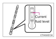
The washer fluid level can be checked by observing the position of the level on the liquid-covered holes in the gauge.
