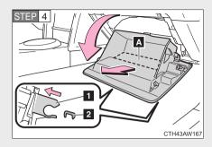
Lower the glove box slowly until surface is horizontal with the floor, then pull it out. (Simply pulling with gentle force will disengage the lower claws.)
