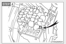
Remove the fuse with the pullout tool.
