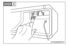
At the garage door opener motor. (security gate motor. the "Learn". locate etc...) "Smart", or "Program" button. This can usually be found where the hanging antenna wire is attached to the motor-head unit (see the device's manual to identify this button). The name and color of the button may vary by manufacturer
