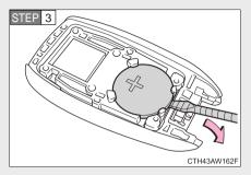
Remove the depleted battery.
