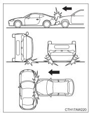
The driver's and front passenger's SRS frontal airbags are designed not to deploy in most cases if the vehicle is struck from the side or from behind, or if it rolls onto its side or roof, or if it is involved in a low-speed frontal collision.
