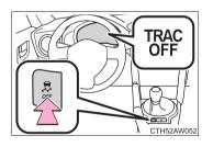
Press  $\left[\begin{array}{c} ? \\ ? \\ ? \end{array}\right]$  to turn off TRAC. ( $\rightarrow$ P. 258)
