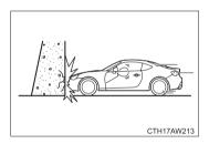
A head-on collision against a thick concrete wall at a vehicle speeds of 12 to 19 mph (20 to 30 km/h) or higher activates only the driver's SRS frontal airbag or both driver's and front passenger's SRS frontal airbags. The airbag(s) will also be activated when the vehicle is exposed to a frontal impact similar in fashion and magnitude to the collision described above.
