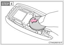
Install a new battery with the "+" terminal facing up, as shown in the illustration.
