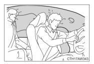
The SRS side airbag and SRS curtain airbag can function only when the ignition switch is in the "ON" position.
