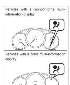
A diagnostic system continually monitors the readiness of the SRS airbag system (including front seatbelt pretensioners) while the vehicle is being driven. The SRS airbag system warning light will show normal system operation by illuminating for approximately 6 seconds when the ignition switch is turned to the "ON" position.
