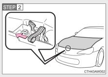
Push the auxiliary catch lever to the left and lift the engine hood.
