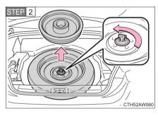
Remove the cover and loosen the center fastener that secures the spare tire.
