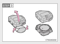
Open the case cover using a coin protected with tape and remove the depleted battery.
