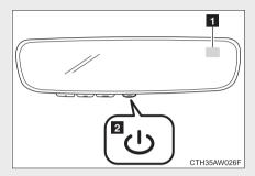
To turn the compass feature on/off, press and hold the Uswitch for more than 3 seconds or until the display turns on/off. The compass feature will default to on with each ignition cycle.
