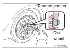
Vehicles with a spare tire of the same wheel type as the installed tires: Tighten the wheel nuts until the tapered portion comes into loose contact with the disc wheel
