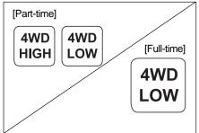
When '4L' operation is no longer needed, rotate the transfer switch from '4L' to 4H'. To shift from '4L' to '4H', stop the vehicle and depress the clutch pedal (on manual transmission) or move the selector lever to 'N' position (on automatic transmission) and rotate the 4WD switch to '4H'.
