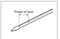
go. Pull it out again and check that the oil level is between the lower mark (Min) and the upper mark (Max) on the oil dipstick. Also check the oil on the dipstick rod for contamination.
