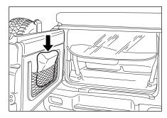
After covering the canvas assembly with boot, latch the fixing device of the boot securely to the rounding parts of the C-pillar molding hook.  Fix the both end parts of the boot by sticking the fasteners(Velcro patch).
