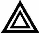
Push the switch once to turn the hazard warning flasher on. When the switch is activated, all directional turn signals will flash on and off to warn oncoming traffic
