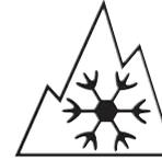
If you need snow tires, select tires equivalent in size and type to the original equipment tires. Use snow tires only in sets of four; failure to do so may
