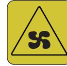
COMPONENT CAN START AUTOMATICALLY ALSO WHEN ENGINE IS OFF
