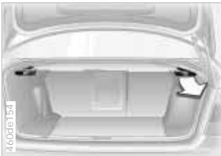
The rear backrest is divided into two sections (one-third and two-thirds of the width of the seat). For carrying longer objects, you can fold down either section of the backrest separately. To unlock, pull the lever corresponding to the section (arrow).
