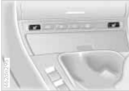
The seat cushion and backrest can be heated with ignition key in position 2.
