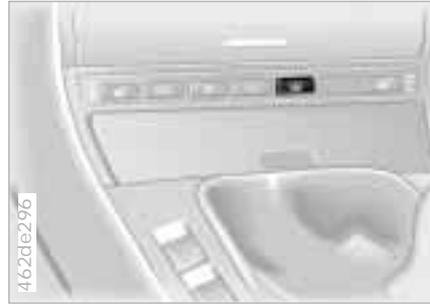
To actuate, press the button briefly with the ignition key in position 1.
