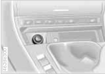
Press the lighter in. Remove the lighter as soon as it pops back out.
