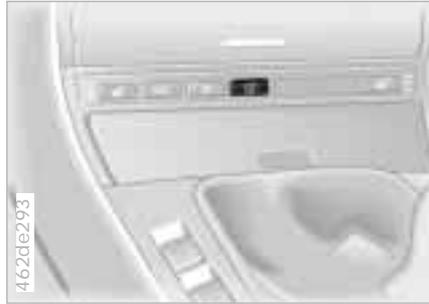
Depending on the type of equipment, the switch either has the letters RDC on it or the RDC-symbol.
