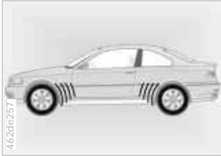
Located near each wheel and embedded in the vehicle body is an antenna that receives signals from the wheel. A central electronics system evaluates the quadruple signals and forwards any changes. The RDC provides an important contribution to driving safety.
