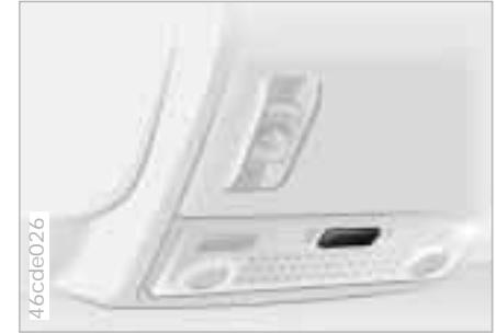
The interior lamps operate automatically.
