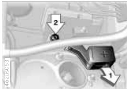
cover of the positive terminal connector is marked with a "+" sign. Refer to the illustration. Remove by pulling the tab (arrow 1).
