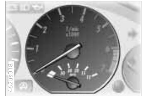
Indicates current fuel consumption in mpg (in l/100 km on Canadian vehicles). You can check your current driving style to see whether it is conducive to economy and minimum exhaust emissions.
