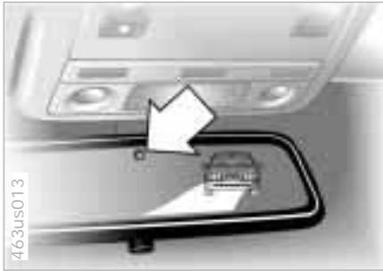
The semisolid reacts chemically to this electrical current, thus providing dimming of the mirror through an infinitely-variable range (electrochromic technology).
