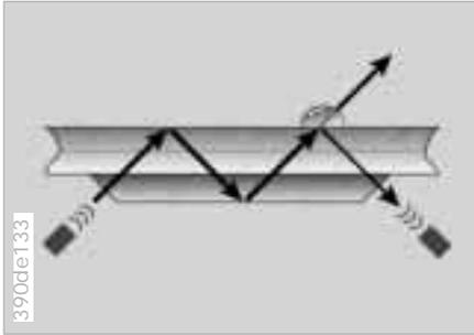
When the system is set to the "Intermittent" wiper speed, the wipers react immediately – if water is splashed onto the windshield by vehicles traveling ahead of you, for example. As a result, the rain sensor provides a contribution to driving safety and comfort.
