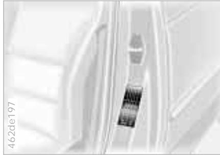
Proper inflation pressures are on a sticker attached to the B-pillar and visible with the driver's door open.
