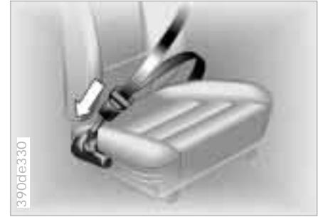
The safety belt tensioner makes sure that the belt tightens during a head-on collision to ensure that occupants remain firmly positioned in their seats. A gas-pressure system retracts the buckle assembly to tension the shoulder and lap belts within fractions of a second. This reduces the tendency to slide under the lap belt.
