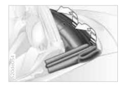
4 Pull the convertible top on the convertible top frame forward and sideways (arrows) and, using a little effort, swing it forward over the window frame
