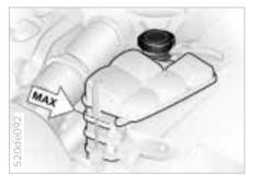
Adjust coolant level when the engine is cold (approx. 68 °F/20 °C):
