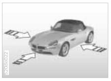
The illustration depicts schematically the primary directions of vehicle impact that initiate airbag deployment.
