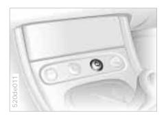
Use this button to operate the central locking system when the doors are closed. The doors and luggage compartment lid are unlocked or locked only. The anti-theft alarm system is not activated.
