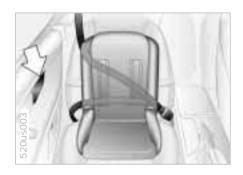
The safety belt on the passenger side can be locked for mounting and securing child restraint systems.
