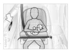
The illustration shows the correct seating position for a child in a child restraint system\* with sufficient distance between him and the side airbag (arrow).
