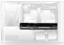
The warning triangle is stored under the luggage compartment's floor panel for easy access.
