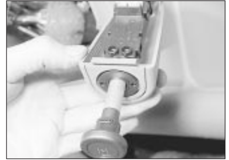
18.8 Choke control unit removal
