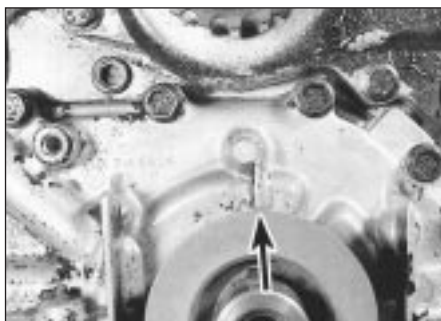
4.7b Align the crankshaft sprocket with its timing mark
