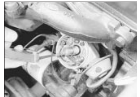
15.4 Checking the contact breaker points gap using a feeler blade
