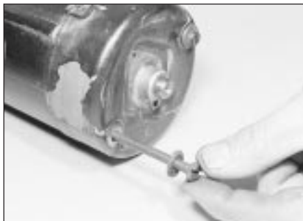
10.4a Remove the commutator end housing securing screws
