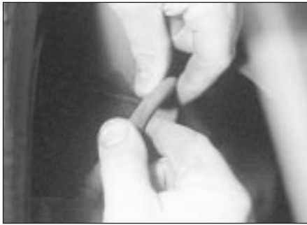
26.1 Bend flexible brake hoses to check for splitting and decay
