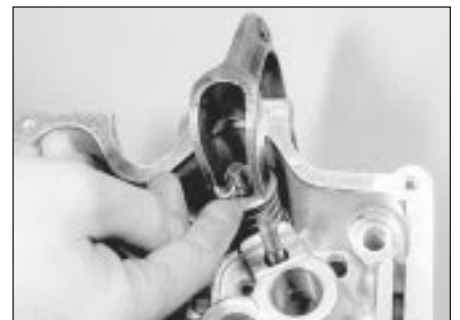
15.44 Compress the spring and insert the split collet
