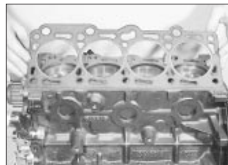
7.21a Locate the new cylinder head gasket
