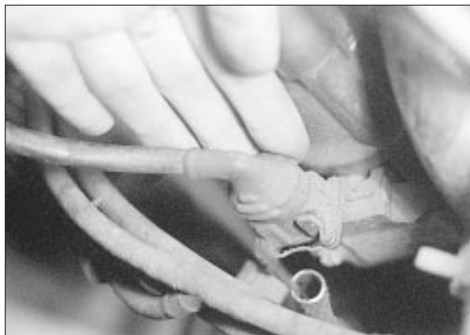
3.21 The distributor LT wiring multi-plug
