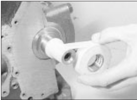
17.11 Tape the front end of the crankshaft to protect the oil pump seal when fitting
