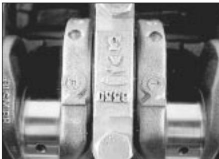
17.5c . . . ensuring that they are positioned correctly according to their markings
