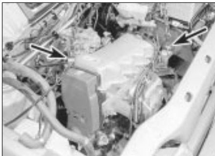
13.6a Attach engine support sling to points indicated (arrowed)
