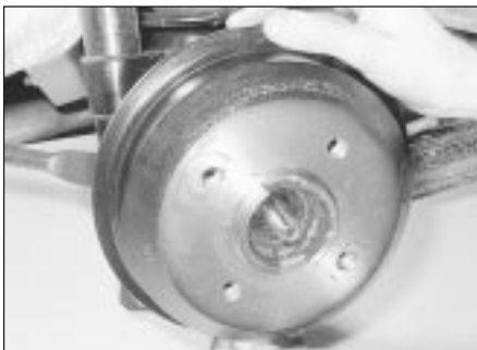
6.9 Withdrawing the brake drum
