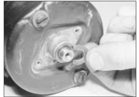
10.3a Remove the C-clip . . .
