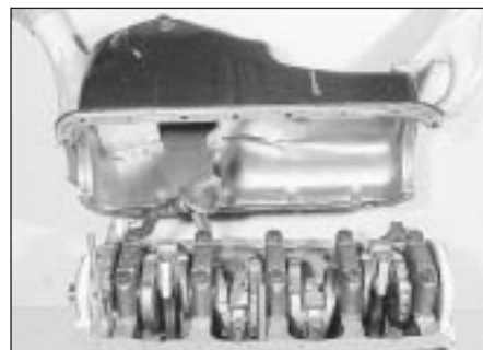
9.8c Fitting the sump over a 4-piece gasket
