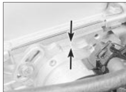
3.1 Distributor and cylinder head alignment marks (arrowed)
