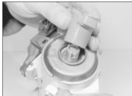
4.9 Removing the rotor arm from the distributor
