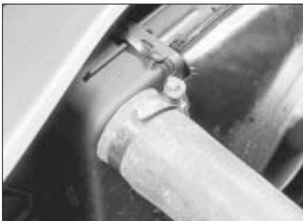
5.2a Disconnect the radiator top hose . . .
