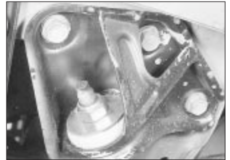
10.2 Tie-bar and mounting bracket Note that the XR2 differs slightly from that fitted to other models
