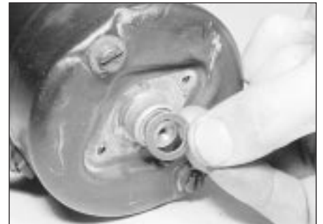
10.3b . . . and shims from the end of the armature shaft
