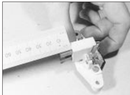
7.2b Compare the brush length with that shown in the Specifications - Bosch alternator
