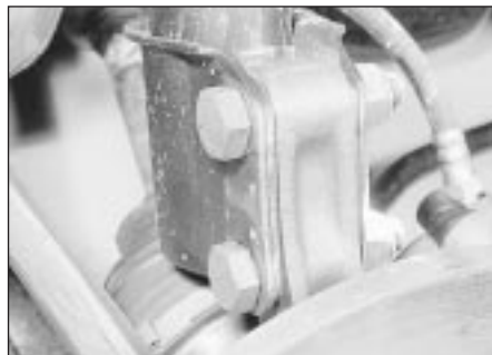
11.3 Suspension strut-to-stub axle carrier retaining bolts
