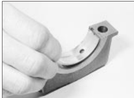
17.5a Fit the bearing shells to the main bearing caps . . .
