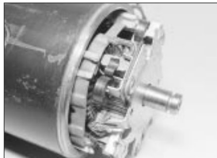
10.4b Commutator end housing removed to expose brush plate
