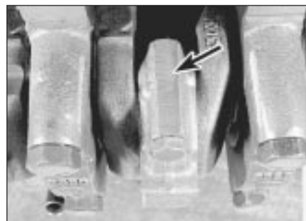
10.2 Connecting rod and big-end cap matching numbers (arrowed)
