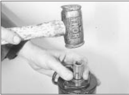
10.29 Using a soft faced hammer and socket to fit a new star clip to the end of the armature shaft - Lucas starter motor
