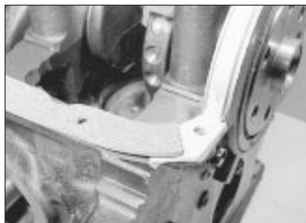
9.8b Sump gasket to overlap sealing strip - 4-piece type
