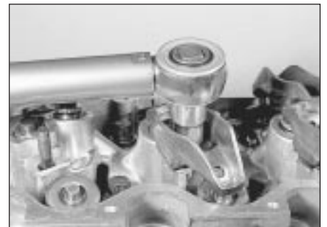
15.49c Tighten the rocker arm nut
