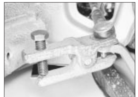
8.14 Separate the balljoint
