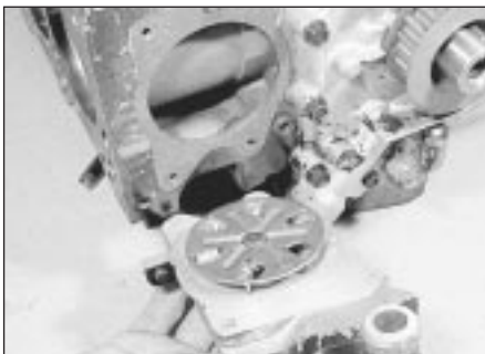
17.18 Fit the coolant pump
