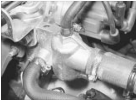
3.7 Thermostat refitted (CVH) with new hoses and clips
