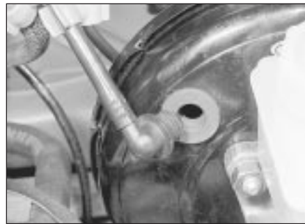
12.1 Vacuum servo pipe removal
