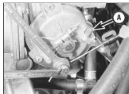
9.10b . . . and tighten retaining screw. Also shown is the fuel choke stop (A)
