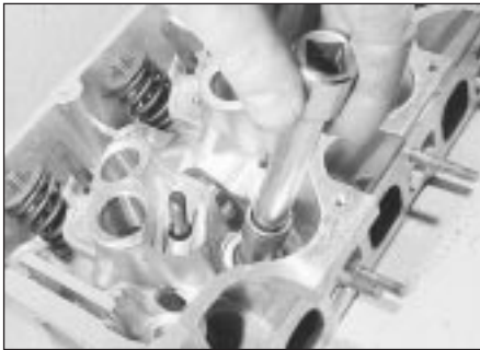
15.41a Using a socket to install a valve stem oil seal
