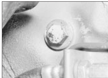
11.2 Right-hand engine mounting side retaining bolt
