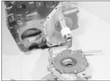
17.13 Oil pump ready for fitting
