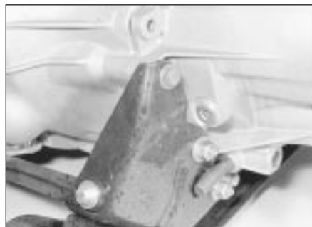
18.5a Engine/gearbox bearer mounting bracket and stay rod
