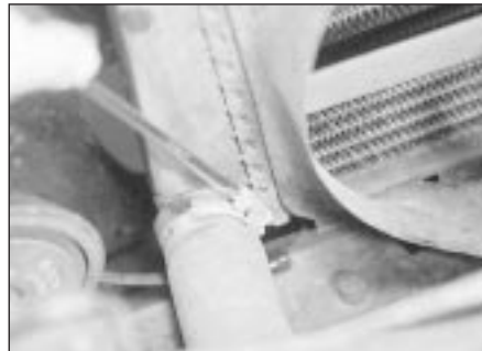
36.3b The radiator bottom hose clamp
