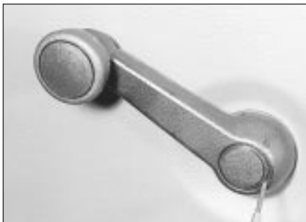
11.7a Remove cover pad from the window regulator handle . . .
