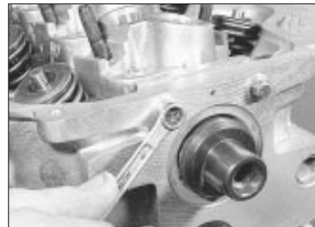
6.17a Unscrewing the camshaft thrust plate bolts
