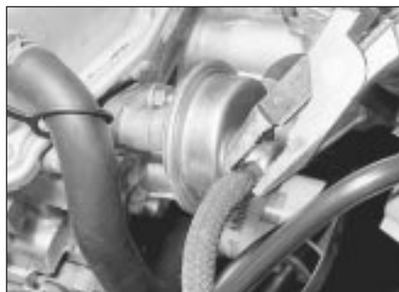
4.7a Detaching hoses from fuel pump - CVH
