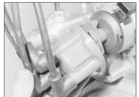
3.4 Distributor cap removal
