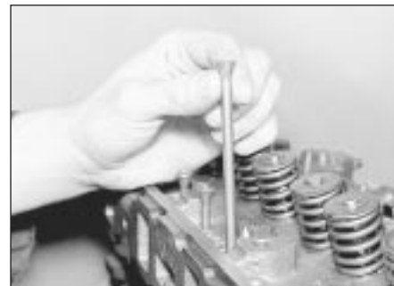
4.19 Withdraw the pushrods
