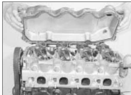
6.10 Remove the rocker cover
