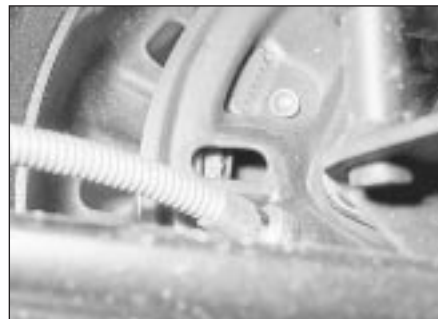
4.4b . . . to check the rear brake linings for wear
