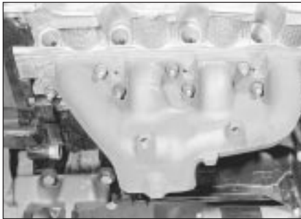
17.24a Refit the exhaust manifold . . .
