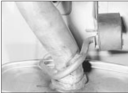
27.3 Exhaust system flexible hanger
