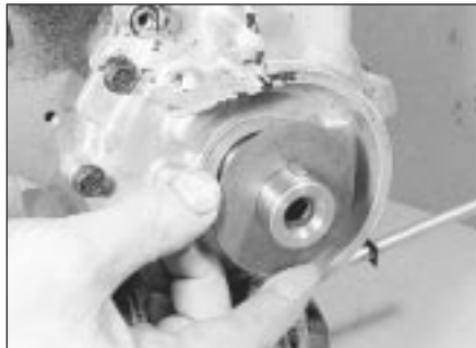
17.16 Locate the thrustwasher . . .
