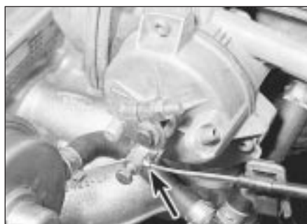
9.10a Locate the ferrule against clamp (arrowed) . . .
