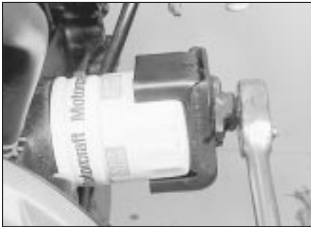
3.7 Removing the engine oil filter with a clamp wrench
