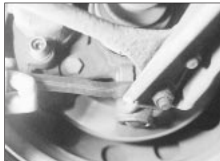
24.4 Apply leverage to check for excessive balljoint wear
