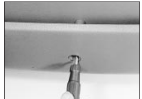
11.8c Remove the trim panel retaining screws
