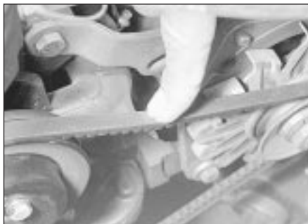
5.4 Check drivebelt tension is correct
