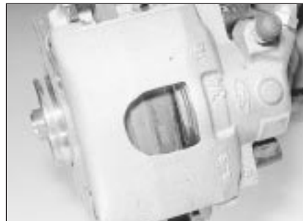
4.2b Inspect the disc brake pads through the caliper housing aperture
