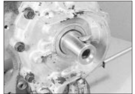
17.14 Insert the crankshaft Woodruff key
