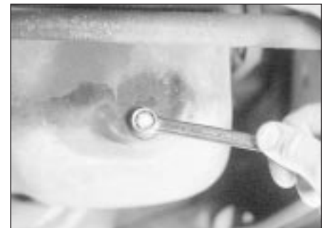
3.3 Removing the sump drain plug
