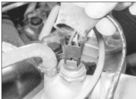
3.3 Disconnect the fan thermal switch lead - OHV
