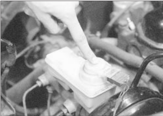
16.6 Depress the brake warning light switch plunger to test
