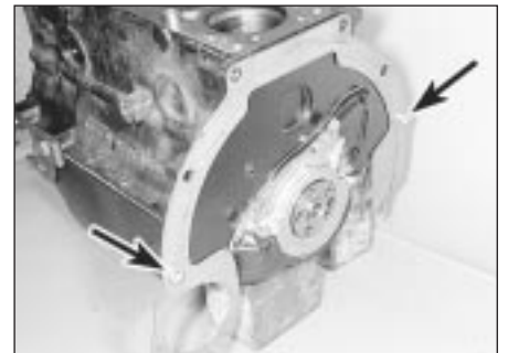
16.17 Locate the engine backplate over the two dowels (arrowed)
