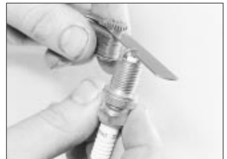
12.2a Measuring a spark plug electrode gap with a feeler blade
