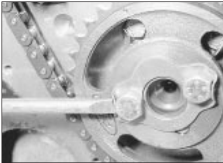
16.12 Secure the camshaft sprocket retaining bolts with the tab washer
