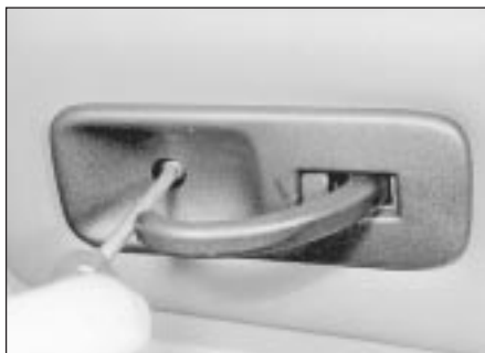
11.9 Remove the door control handle bezel screw
