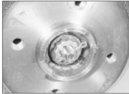
6.7b . . . the split pin and nut lock . . .
