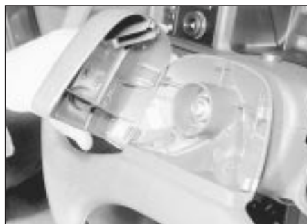
2.1 Removing the steering wheel trim to reveal the steering wheel retaining nut
