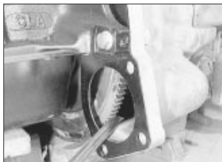
4.7c One method of jamming the flywheel ring gear . . .
