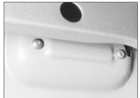
11.32 Door exterior handle retaining screws viewed from within the door
