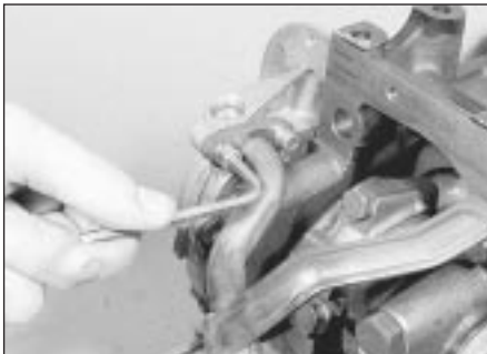
17.15 Fit the oil pump pick-up tube retaining bolts
