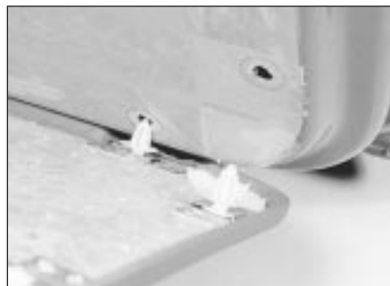
11.11 Prise free the door panel and locating clips
