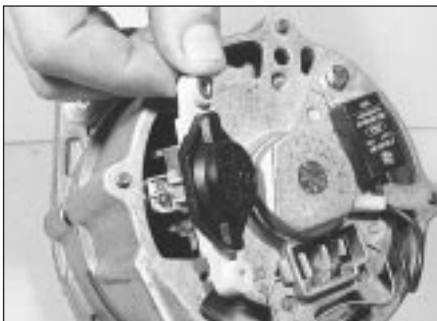
7.2a Withdrawing the regulator/brush box - Bosch alternator
