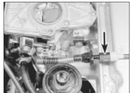
7.10 Throttle cable adjusting sleeve (arrowed)
