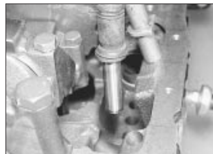
13.34 Lift out the cam followers (tappets), using a valve grinding tool
