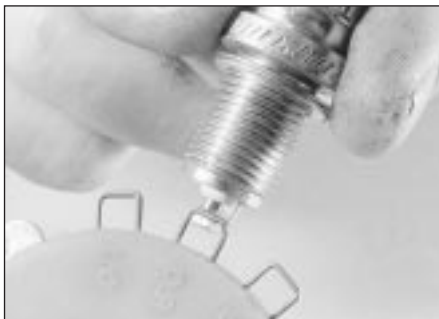
12.2b Measuring a spark plug electrode gap with a wire gauge
