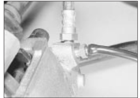
2.5 Bleed tube attached to bleed screw on front brake
