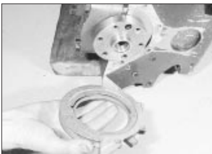
17.20 Locate the crankshaft rear oil seal and retainer
