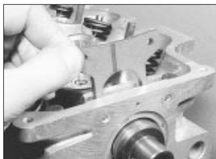
6.17b Lifting out the camshaft thrust plate
