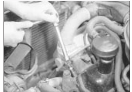
12.1b . . . before using a socket to remove the spark plugs
