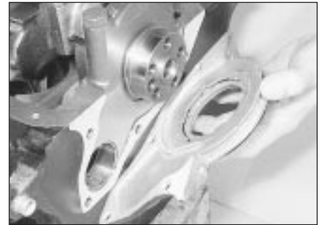
16.16 Refit the crankshaft rear oil seal retainer - note new gasket
