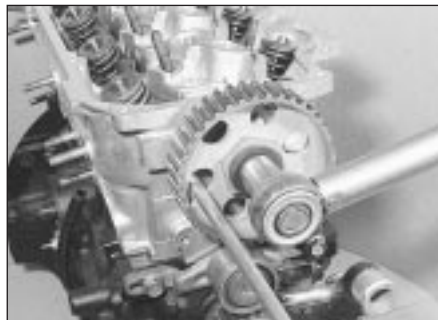
6.16 Method used to loosen the camshaft sprocket bolt
