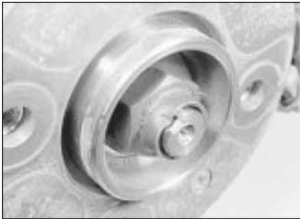
8.40 Stake the hub nut to secure
