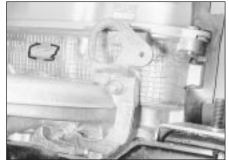
17.24c Engine lift hook is fitted with the inlet manifold
