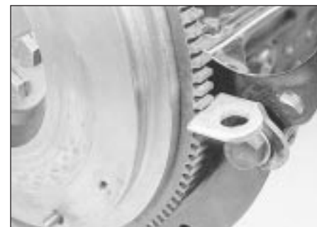
4.7d . . . another method of jamming the flywheel ring gear
