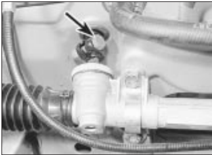
3.8 Pinion coupling clamp bolt (arrowed)
