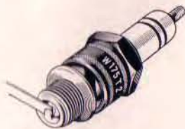
How to measure the electrode gap with a feeler gauge.
