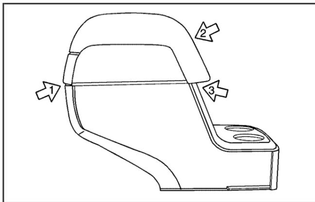
To access the upper storage area, press the upper button (2) and lift up. To access the lower storage area, press the lower button (3) and lift up. The top of the console can be folded forward for increased storage area. Lift up on handle on the rear of the console (1) and pull forward.
