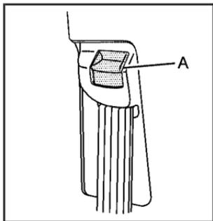
To move it down, push down on the button (A) and move the height adjuster to the desired position. You can move the height adjuster up by pushing up on the shoulder belt guide.
