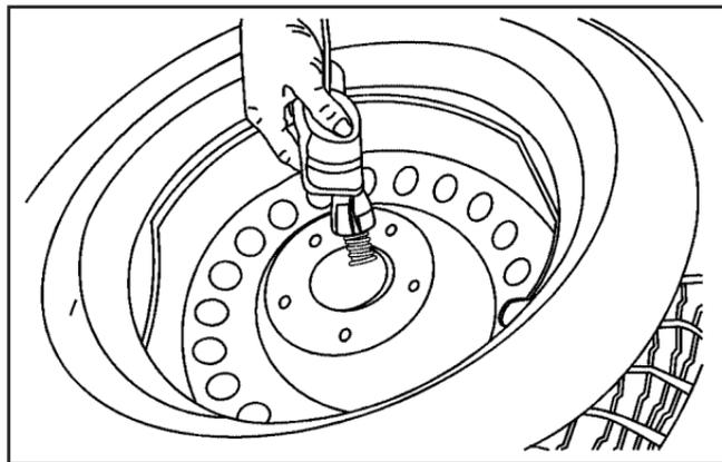
5. Tilt the retainer and slip it through the wheel opening to remove the spare tire from the cable.
