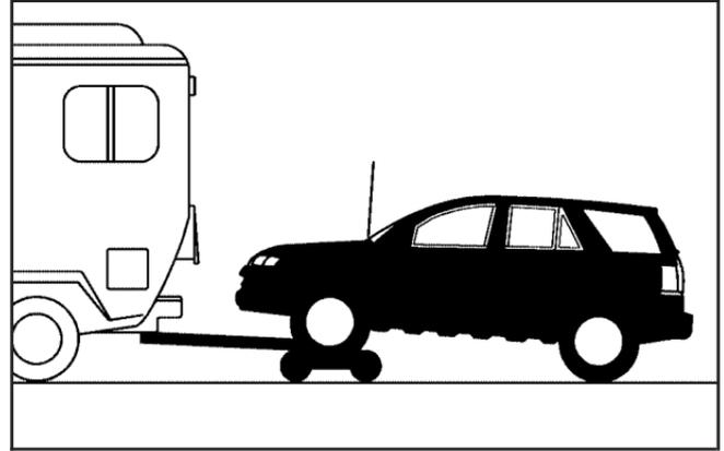
To tow your front-wheel-drive vehicle from the front with two wheels on the ground:
