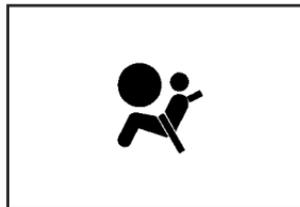
This light comes on when the vehicle is started, and flashes for a few seconds. The light should go out when the system is ready.
