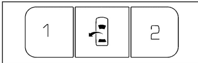
The controls for this feature are located on the driver's door panel, and are used to program and recall memory settings for the driver's seat and outside mirrors.
