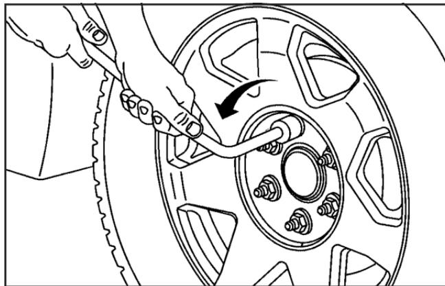
3. Loosen the wheel nuts — but do not remove them — using the lug wrench. For wheels with a wheel lock key, use the wheel lock key between the lock nut and lug wrench.
