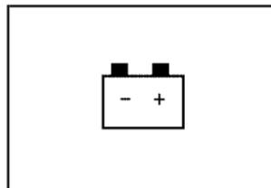
This light comes on briefly when the ignition key is turned, but the engine has not started to run, as a check to show you it is working.
