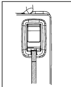
3. Pull up on the release lever located on the back of the seat. The headrest moves forward automatically.
