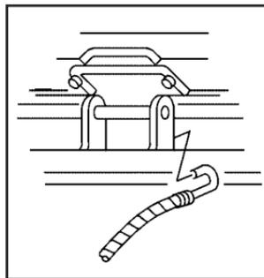
6. Hook the other end of the cable onto the outer portion of the liftgate hinge (B).
