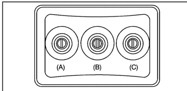
The A/V jacks, located on the rear of the floor console, allow audio or video signals to be connected from an auxiliary device such as a camcorder or a video game unit to the RSE system. Adapter connectors or cables (not supplied) might be required to connect the auxiliary device to the A/V jacks. Refer to the manufacturer's instructions for proper usage.
