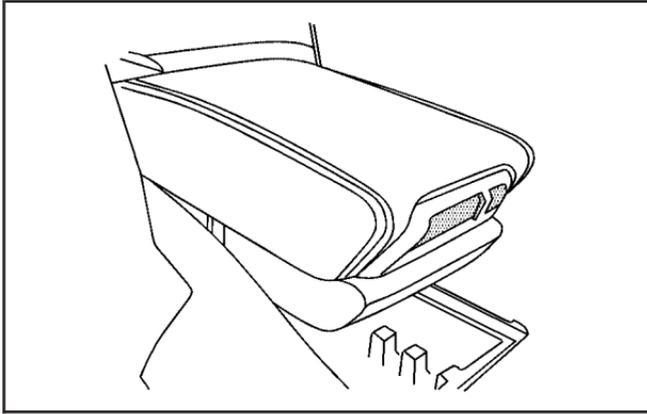
The armrest on the center console can slide forwards and backwards by holding up the lever located on the front of it. To open the armrest storage area, press the button located on the front of the armrest. There is additional storage under the armrest. Move the armrest all the way to the rear position. The tray can be removed for additional storage.
