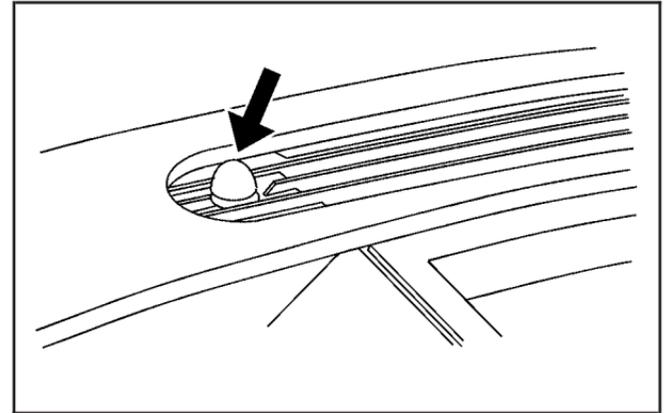
The solar sensor, located in the defrost grille in the middle of the instrument panel, monitors the solar radiation. Do not cover the solar sensor or the system will not work properly.
