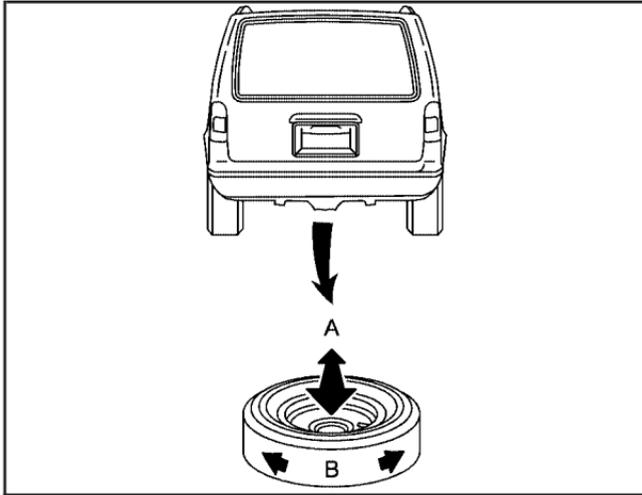
6. Make sure the tire is stored securely. Push, pull (A), and then try to turn (B) the tire. If the tire moves, use the lug wrench to tighten the cable.
