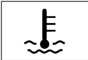
The engine coolant temperature warning light will come on when the engine has overheated.
