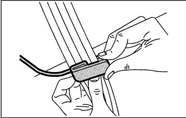
2. Place the guide over the belt, and insert the two edges of the belt into the slots of the guide.
