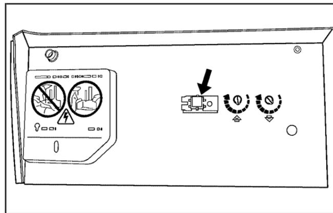
6. After Steps 1 through 5 have been completed, locate inside the garage the garage door opener receiver (motor-head unit). Locate the “Learn” or “Smart” button. The name and color of the button may vary by manufacturer.
