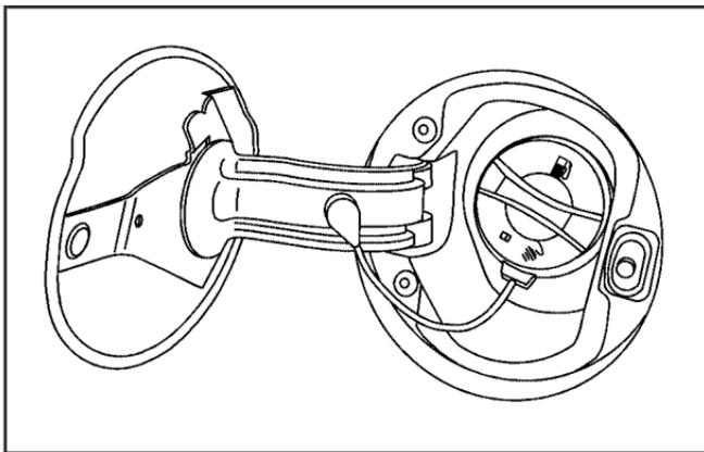
To remove the fuel cap, turn it slowly counterclockwise. The fuel cap has a spring in it; if the cap is released too soon, it will spring back to the right.
