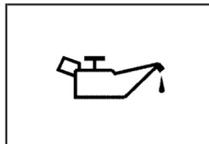
This light comes on briefly when the engine is started as a check to make sure it works. If it does not, the vehicle needs service.
