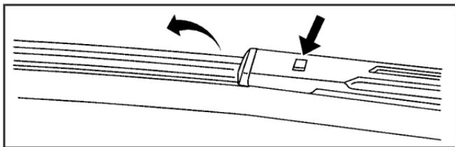
2. Press the button in the middle of the wiper arm connector, and pull the wiper blade away from the arm connector.
