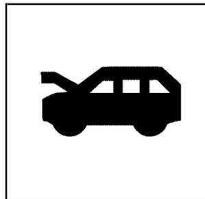
1. Pull the hood release handle with this symbol on it. It is located under the instrument panel on the driver's side of the vehicle.
