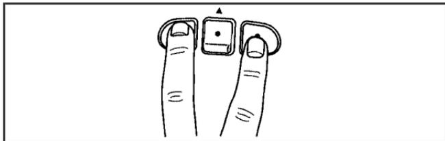
1. From inside the vehicle, press and hold down the two outside buttons at the same time, releasing only when the Universal Home Remote indicator light begins to flash, after 20 seconds. This step will erase the factory settings or all previously programmed buttons.
