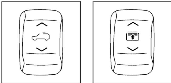
**Vent:** From the closed position, press and hold the front of the driver's side switch to vent the sunroof. Press and hold the rear of the driver's side switch to close the sunroof.
