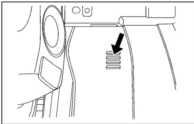
The interior temperature sensor located on the instrument panel to the right of the steering column, measures the temperature of the air inside the vehicle.
