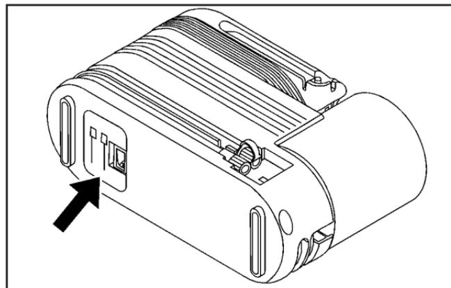
Your tire sealant and compressor kit has an accessory adapter located in a compartment on the bottom of its housing that may be used to inflate air mattresses, balls, etc.
