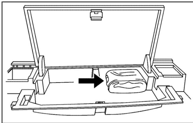
3. The tire sealant and compressor kit is located on the passenger side of the storage compartment.
