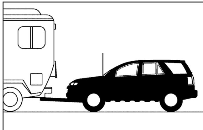
If you have a front-wheel-drive vehicle, it can be dinghy towed from the front. These vehicles may also be towed by putting the front wheels on a dolly. See “Dolly Towing” later in this section.
