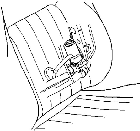
Figure 1. Seat Recline Motor Removal
