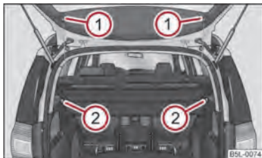
Fig. 61 Removing the luggage compartment cover
