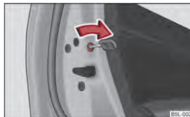
Fig. 11 Child safety locks on the rear doors
