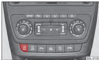
Fig. 105 Dash panel: START-STOP System button
