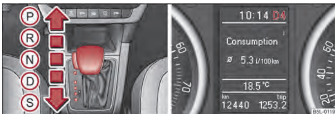
Fig. 106 Selector lever/information display: Selector lever positions
