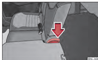
Fig. 54 Folding the seat backrest back into position
