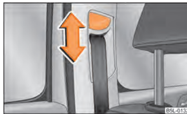
Fig. 119 Front seat: Seat belt height adjuster
