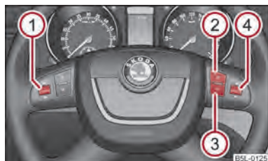
Fig. 112 Multifunction steering wheel: Mobile phone operation
