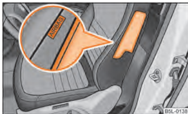
Fig. 125 Installation position of side airbag in driver seat
