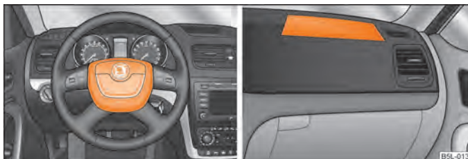
Fig. 121 Driver airbag in the steering wheel/front passenger airbag in the dash panel
