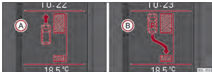
Fig. 102 Information display: the determined parking space with the information to drive on (A) and for engaging the reverse gear (B)
