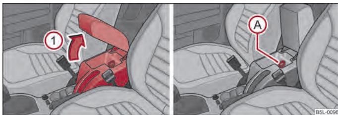
Fig. 83 Armrest: Storage compartment/cooling of storage compartment
