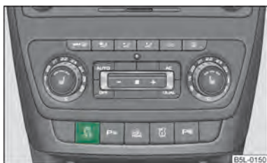
Fig. 137 ESP system: Switch for TCS
