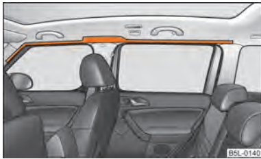
Fig. 127 Installation position of the head airbags
