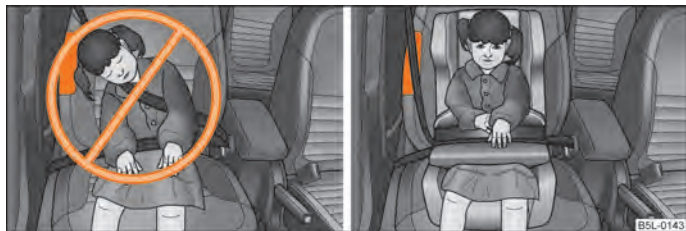
Fig. 130 Seated position of an unprotected child at risk from side airbag/Child properly protected by safety seat
