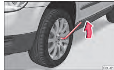
Fig. 168 Changing a wheel: Loosening the wheel bolts
