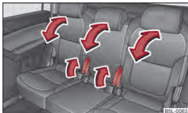
Fig. 50 Adjusting the seat backrest
