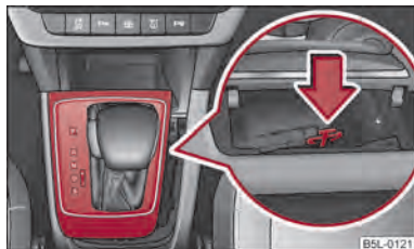
Fig. 108 Selector lever-emergency unlocking
