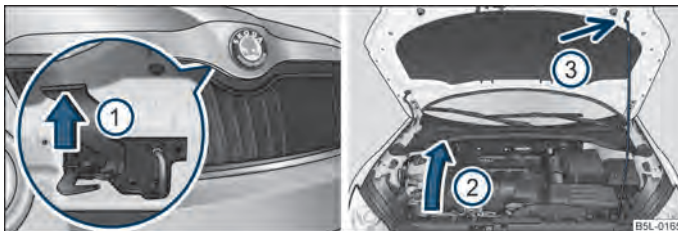
Fig. 152 Radiator grille: Locking lever/securing the bonnet with the bonnet support
