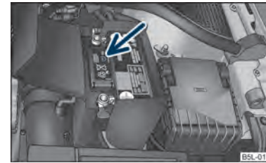
Fig. 158 The battery: Electrolyte level indicator
