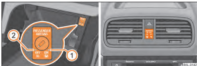
Fig. 129 Storage compartment: Switch for the front passenger front airbag/warning light for a switched off front seat passenger airbag
