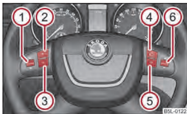
Fig. 109 Multifunction steering wheel: control buttons
