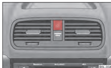
Fig. 29 Dash panel: Switch for hazard warning lights
