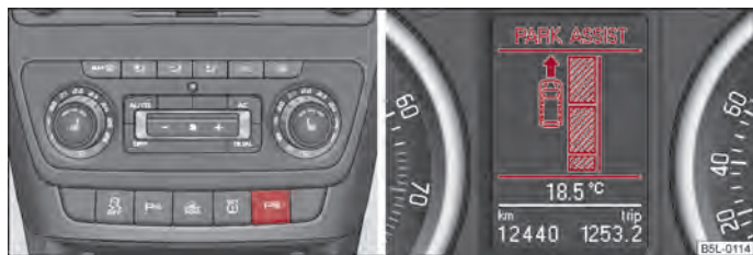
Fig. 101 Switching on the park assist/information display: Finding a suitable parking space
