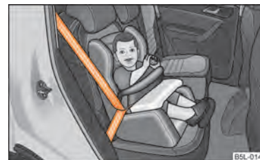
Fig. 132 Child seat with padded table in Group 1 installed on rear seat bench facing the direction of travel
