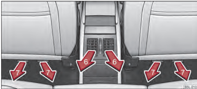
Fig. 89 Air vents at the rear
