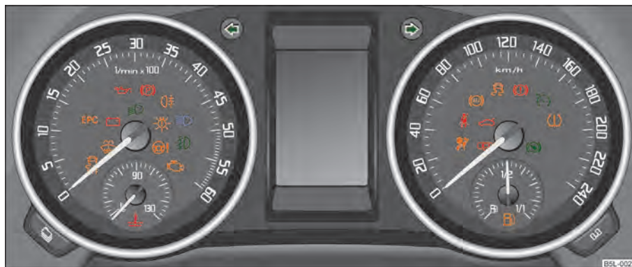
Fig. 8 Instrument cluster with warning lights
