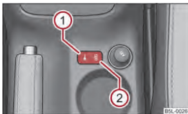
Fig. 13 Centre console: Central locking system
