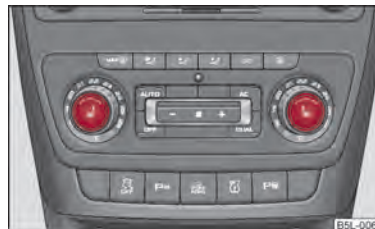
Fig. 56 Dash panel: Regulator for front seat heating
