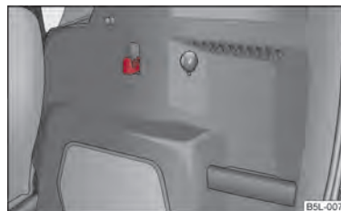
Fig. 58 Luggage compartment: folding hooks
