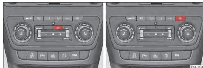
Fig. 35 Switch for windscreen heater/switch for rear window heater
