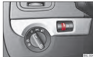
Fig. 27 Dash panel: Instrument lighting
