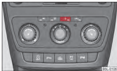
Fig. 93 Button for direct switching on/off of the auxiliary heating (auxiliary heating and ventilation) on the operating part of the air conditioning system
