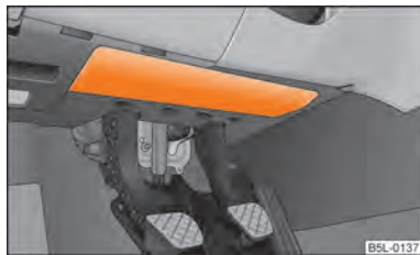
Fig. 124 Driver's knee airbag below the steering column
