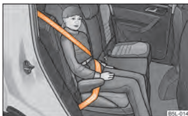
Fig. 134 Child seat in Group 3 installed on the rear seat facing the direction of travel
