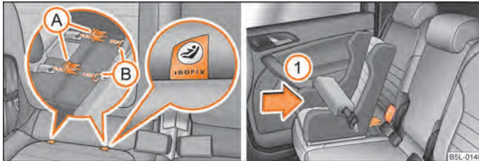
Fig. 135 Locking eyes (ISOFIX system)/the ISOFIX child seat is pushed into the mounting funnels
