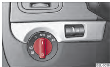
Fig. 25 Dash panel: Light switch
