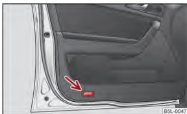
Fig. 34 Front door: Warning light
