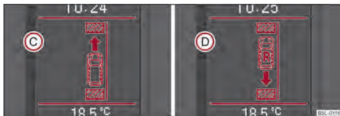
Fig. 103 Information display: Information for engaging the forward gear (C) or the reverse gear (D)
