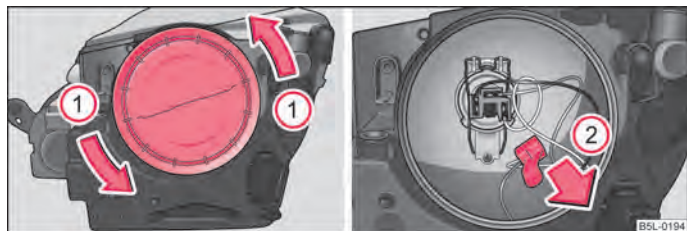
Fig. 182 Remove cap/removing the fixture for the parking light (halogen headlight)
