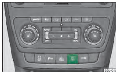
Fig. 139 Button for setting the tyre inflation pressure control value
